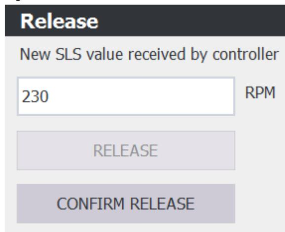
If the “Confirm release” button is not pressed within one minute, the button will be grayed out and the release must be retrIGGERED.
