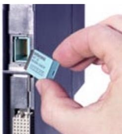
Figure 5-2 Inserting a C-PLUG
