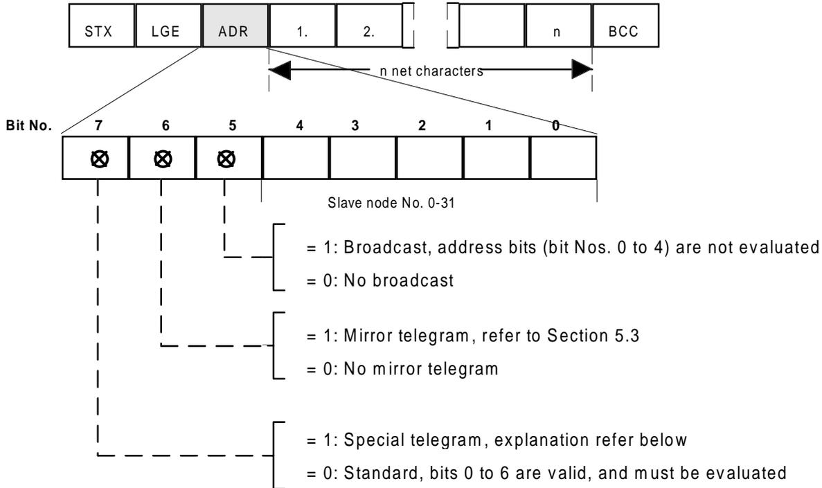
Fig. 4.2: Assignment of the address bytes (ADR)
