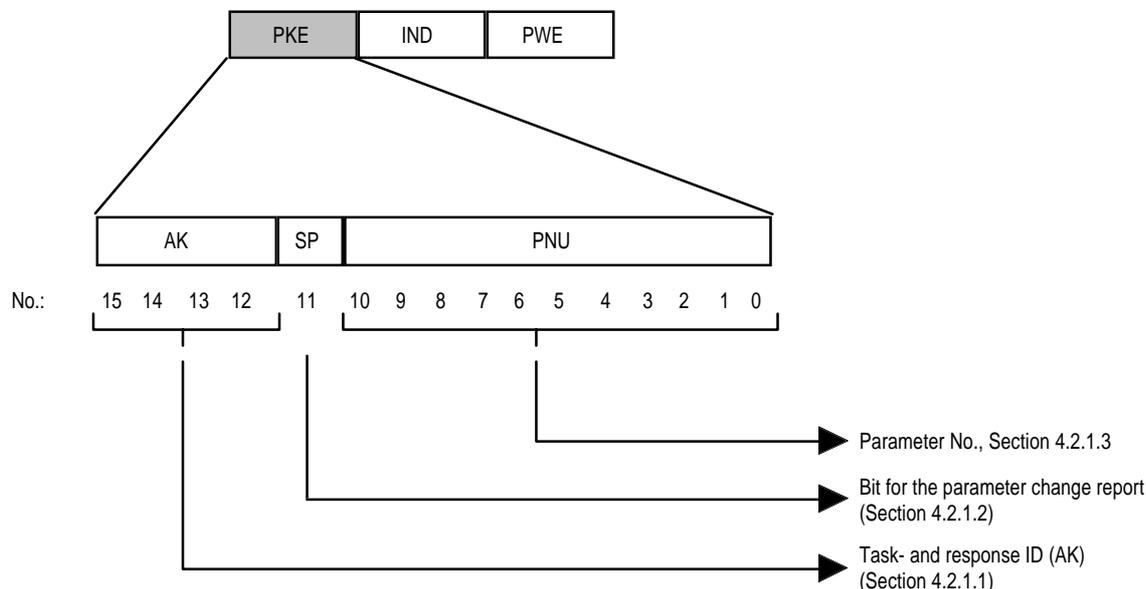
Fig. 4.4: Parameter ID structure
