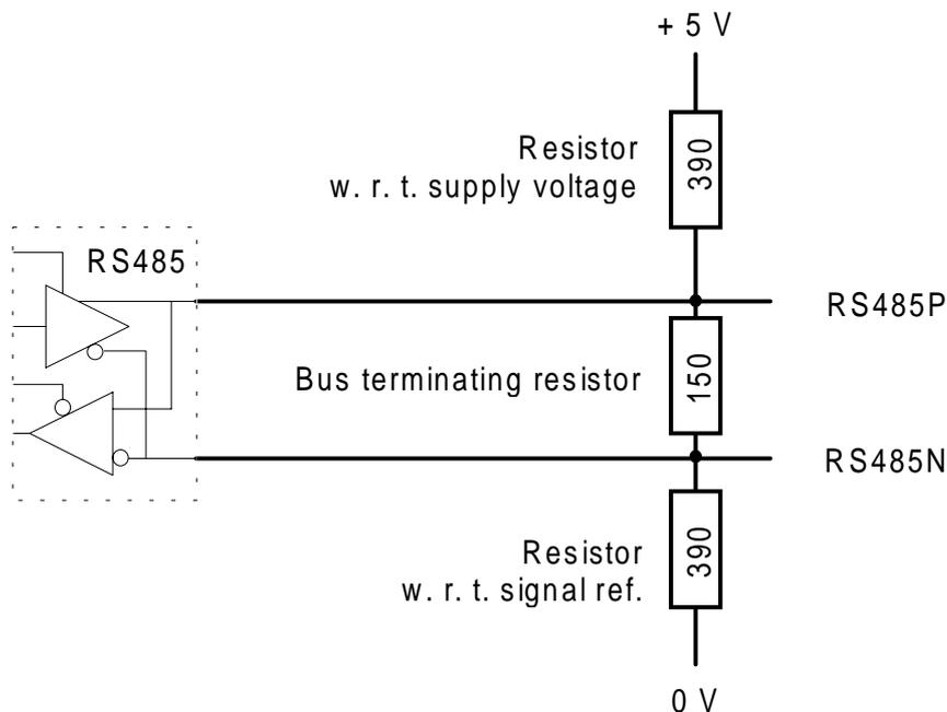
Fig. 4.1: Basis network and bus termination
