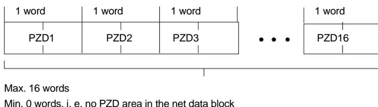
Fig. 5.1: Structure of the process data area PZD
