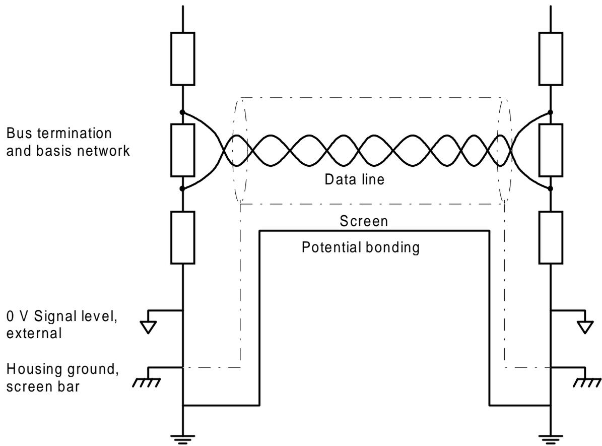
Fig. 4.2: Screening and potential bonding
