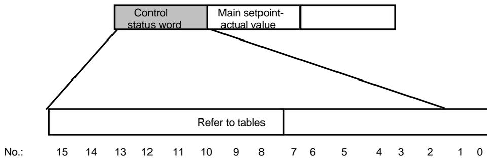
Fig. 5.2: Structure of the control- and status word
