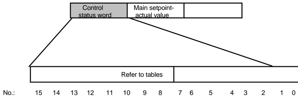
Fig. 5.2: Structure of the control- and status word
