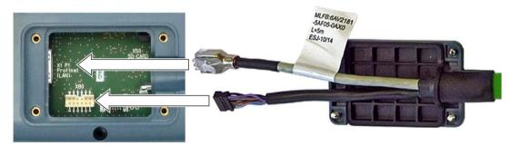
2. Plug in the RJ45 connector at port X1.
