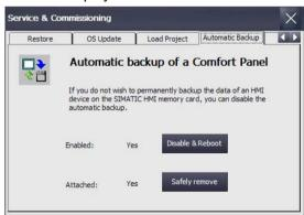
You can see whether or not a system memory card is inserted under "Attached:".
