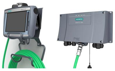
With a fail-safe Mobile Panel, you run the plant in fail-safe mode. You meet the requirements of Safety Integrity Level 3 and Performance Level PL e with a fail-safe Mobile Panel. An emergency stop / stop switch and an enabling button are integrated in a fail-safe Mobile Panel 2nd Generation. You can evaluate the safety-related operator controls in a hard-wired F-system using safety relays.
