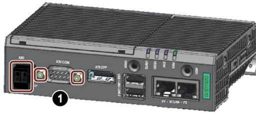
2. Loosen the top housing. Carefully press with the blade of a flat-blade screwdriver in the marked recesses and carefully pull on the appropriate place on the top housing of the enclosure.
