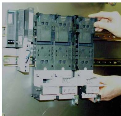
Using both hands shift the terminal module - without skewing it - to the left to the already mounted modules until it audibly latches into the adjacent module.
