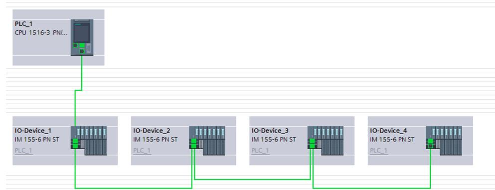
All the IO devices are configured as optional IO devices; hence all the ports have to be firmly connected following the topology.
