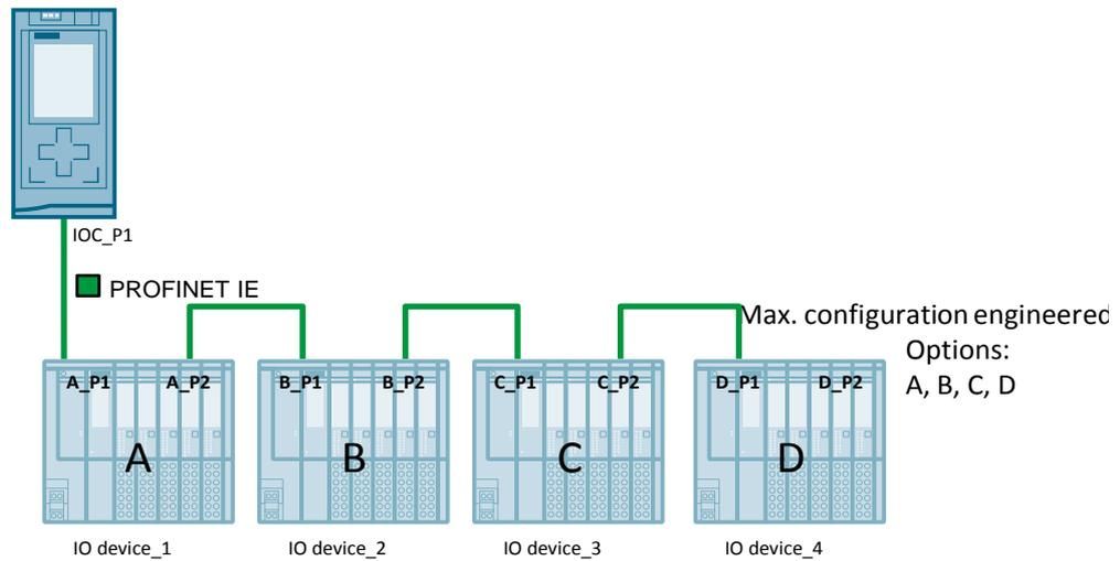
In this example, you are free to change the sequence of the IO devices A, B, C, and D.
