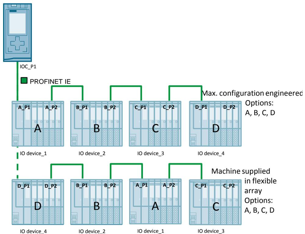
This means that the machine supplied can be set up in flexible array, for example in order to reduce the amount of wiring. In our example, the sequence (A, B, C, D) of the maximum configuration is changed to D, B, A, C.
