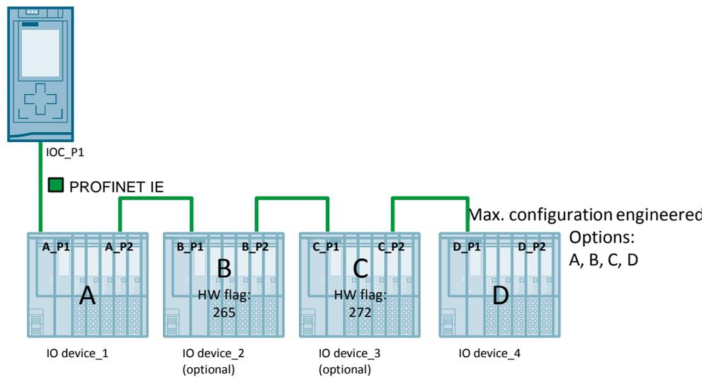
In our example, the options A and D are flexibly interchangeable. However, options B and C can only be used together with A and D as, following the topology, they are firmly connected to the interfaces “A\_P2” and “D\_P1”.
