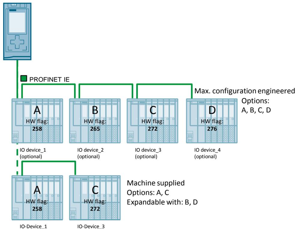
This means that the machine supplied may be extended with the different options. In the present example, options A and C are activated. At a later moment, the machine can also be extended with options B and D.
