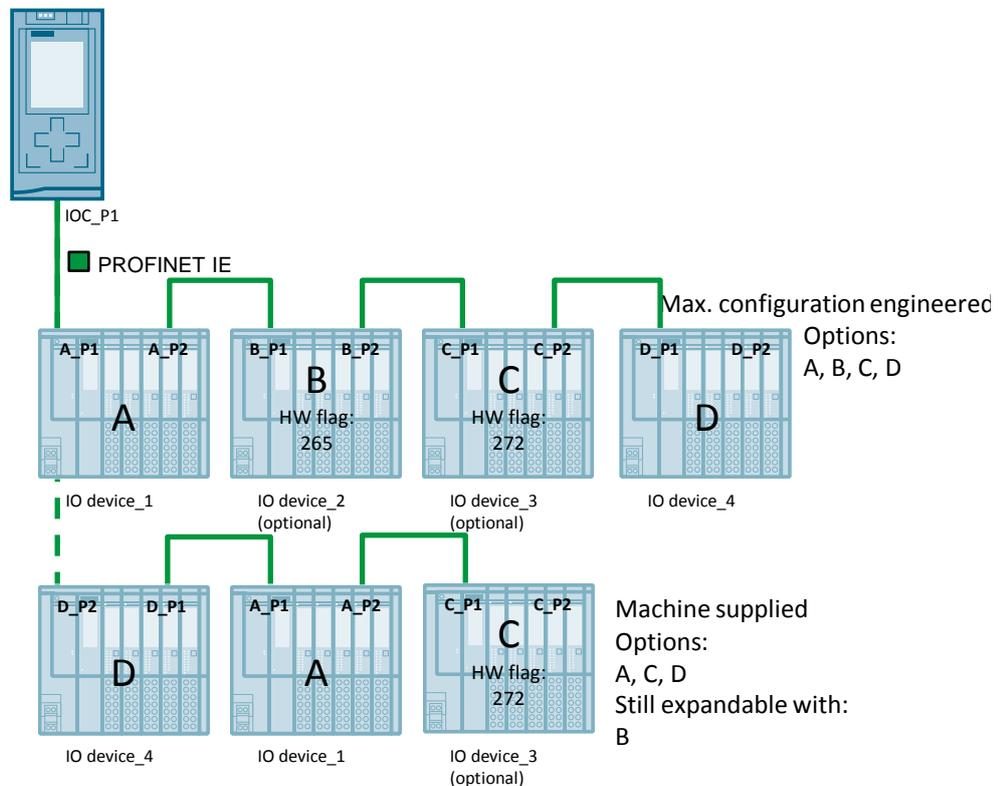
In the machine supplied, the IO device D is connected to the IO controller with port “D\_P2”. The IO device A is connected to D with the optional IO device C. The machine may still be extended with B.
