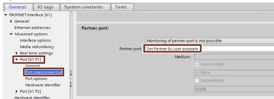
5. In the submenu, select the port connected to component **after** ("A\_P2" in this case). In "Port interconnection", set the "Partner port". Select the option "Set Partner by application program" from the drop-down list.
