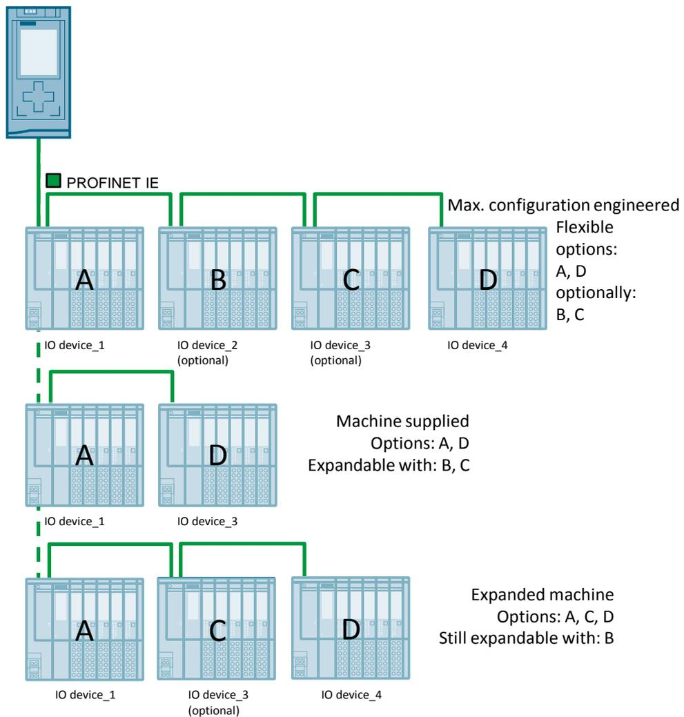
The Configuration Control enables you to operate different configuration levels of a series machine with a single project engineered in the maximum configuration. You can select the configuration level via the application program.
