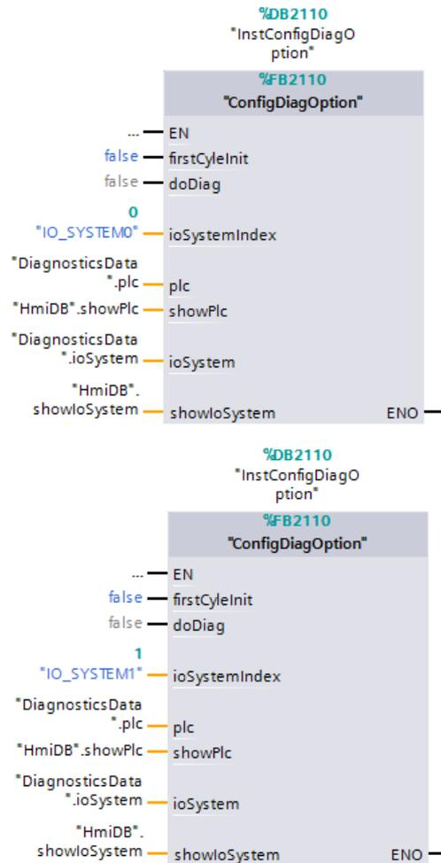
Figure 3-4 Call in the diagnostics functions
