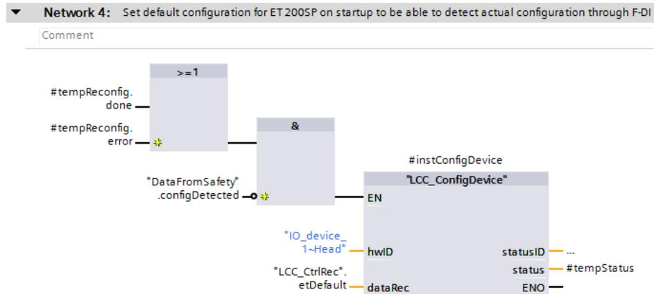
7. Program the configuration control of the remaining configurations of the ET 200SP station. You may use the same instance but must ensure that a maximum of one call is processed per cycle.
