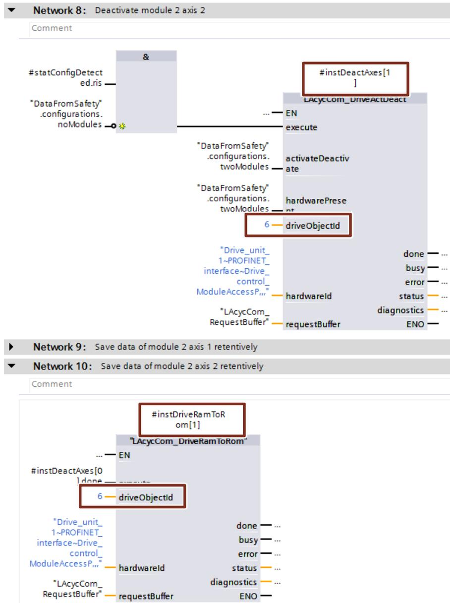
**Note** In a DMM, both motor modules must be activated or deactivated separately.
