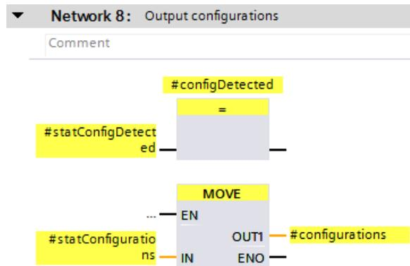
10. Open the FB "Main\_Safety" and call the newly created FB in it. Connect the outputs with a standard DB to transfer the configuration selection to the standard user program.
