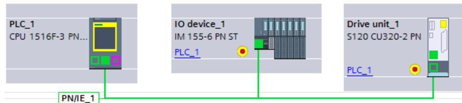
3. Create the topology so that the IO-Controller can assign PROFINET device names and IP addresses to the IO-Devices during commissioning.
