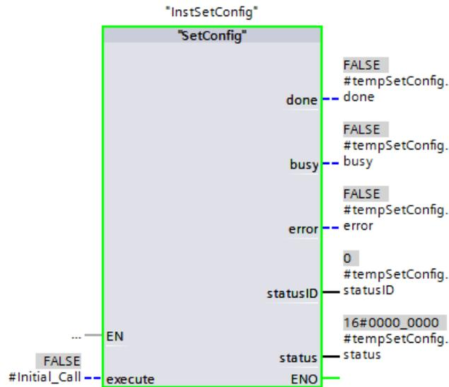
In the event of an error, the status codes of the called blocks are output at output "status" and the source of the error is specified at output "statusID".
