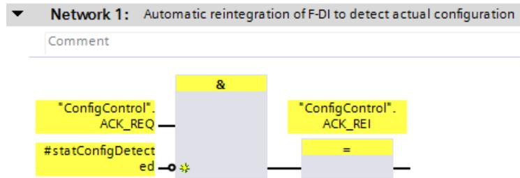
6. Program the selection of configurations. To ensure that the selection is selected only once after the CPU is started and does not change even if the wiring is changed during operation, evaluate the static variable "statConfigDetected".
