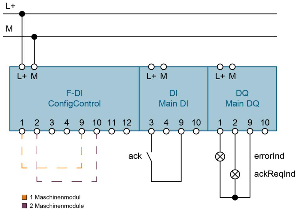
4. Wire a pushbutton to reintegrate fail-safe I/O modules and acknowledge safety functions and faults.
