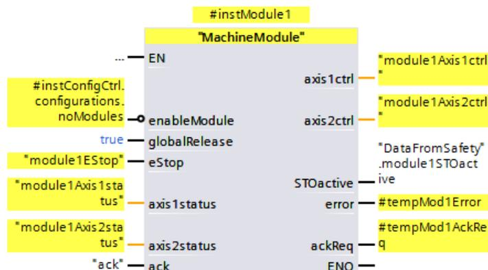
In the FB, an emergency stop command device is evaluated as an example and the safety functions in the drive are controlled using the "LDrvSafe" block library. You can download the block library "LDrvSafe" from the Siemens Industry Online Support:
