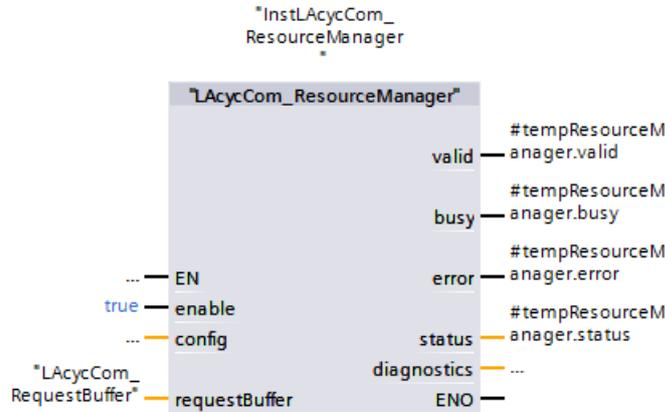
The default configuration is sufficient for this application. The input "config" is therefore not connected.
