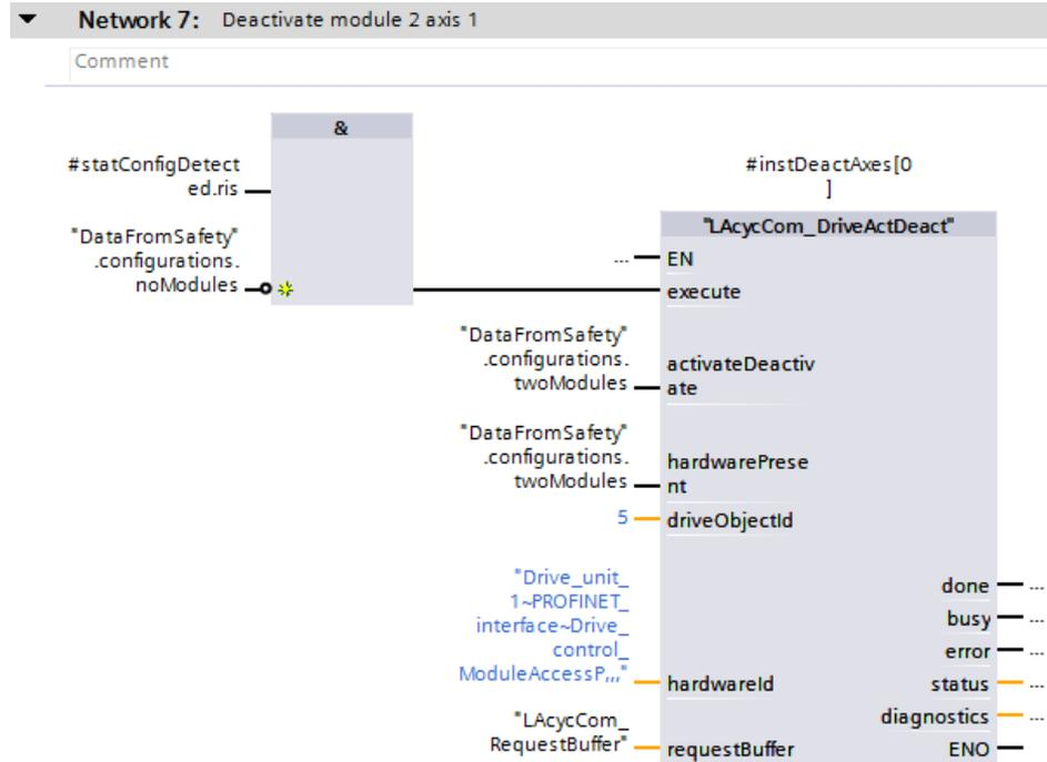
4. To activate or deactivate the motor module depending on the actual configuration, create the variable of the configuration in which the motor module exists at the inputs "activateDeactivate" and "hardwarePresent".
