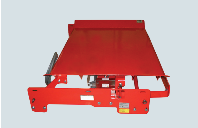
SITRANS WB310 is a heavy-duty, full-frame two load cell, pivoted pan based, belt scale used for process monitoring.
