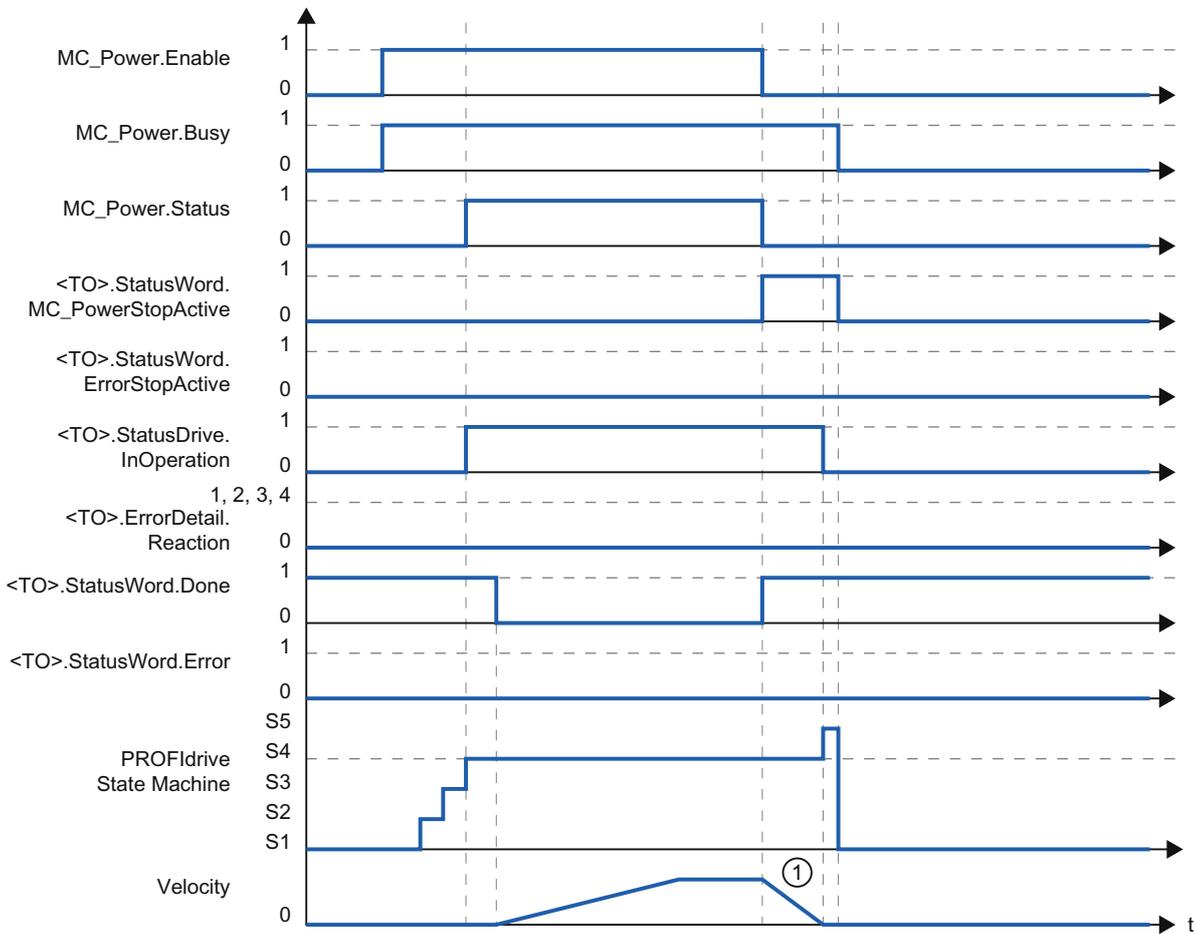
① The axis decelerates with the configured emergency stop deceleration.
