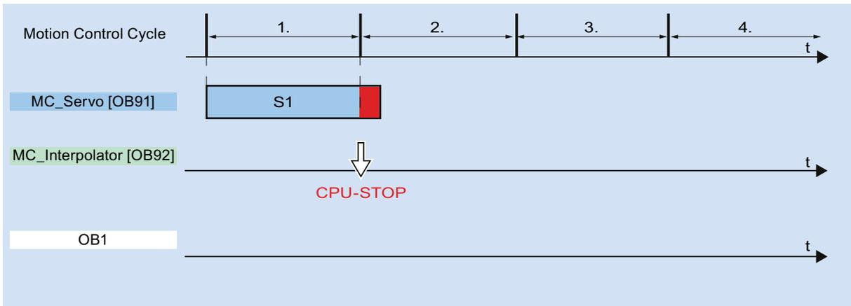
The processing of an MC Interpolator [OB92] can be interrupted by at most one call of the MC Servo [OB91]. If more interruptions occur, the CPU switches to STOP mode.
