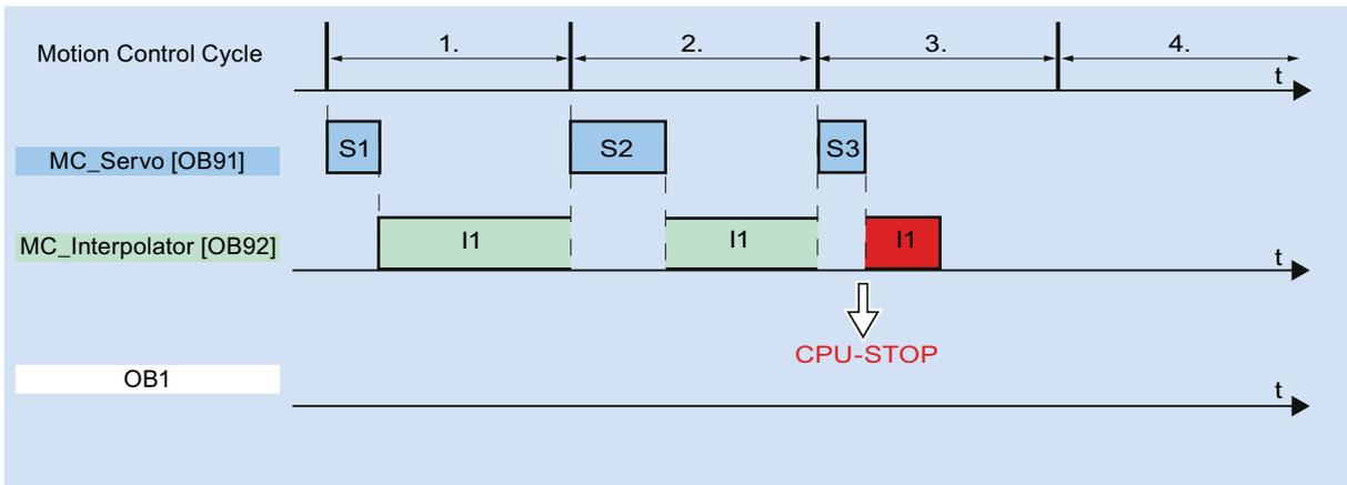
The MC Interpolator [OB92] tolerates a maximum of three successive CPU timeouts. If more timeouts occur, the CPU switches to STOP mode.
