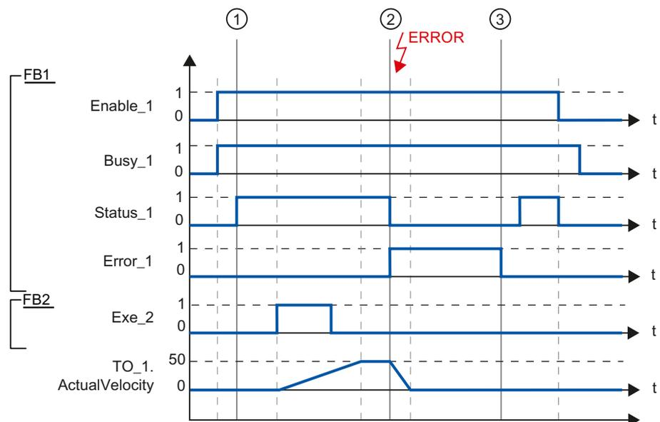
A technology object is enabled with "Enable\_1= TRUE". Successful enabling can be read from "Status\_1" at time ①. The axis will then move with an "MC\_MoveVelocity" job (A2). The velocity profile of the axis can be read from "Velocity Axis\_1".
