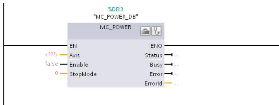
The instance data block is automatically created under "Program Blocks > System Blocks > Program Resources".
