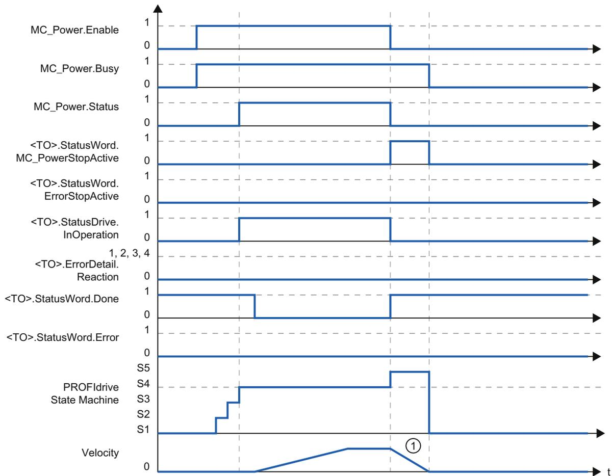
① The deceleration ramp depends on the configuration in the drive.
