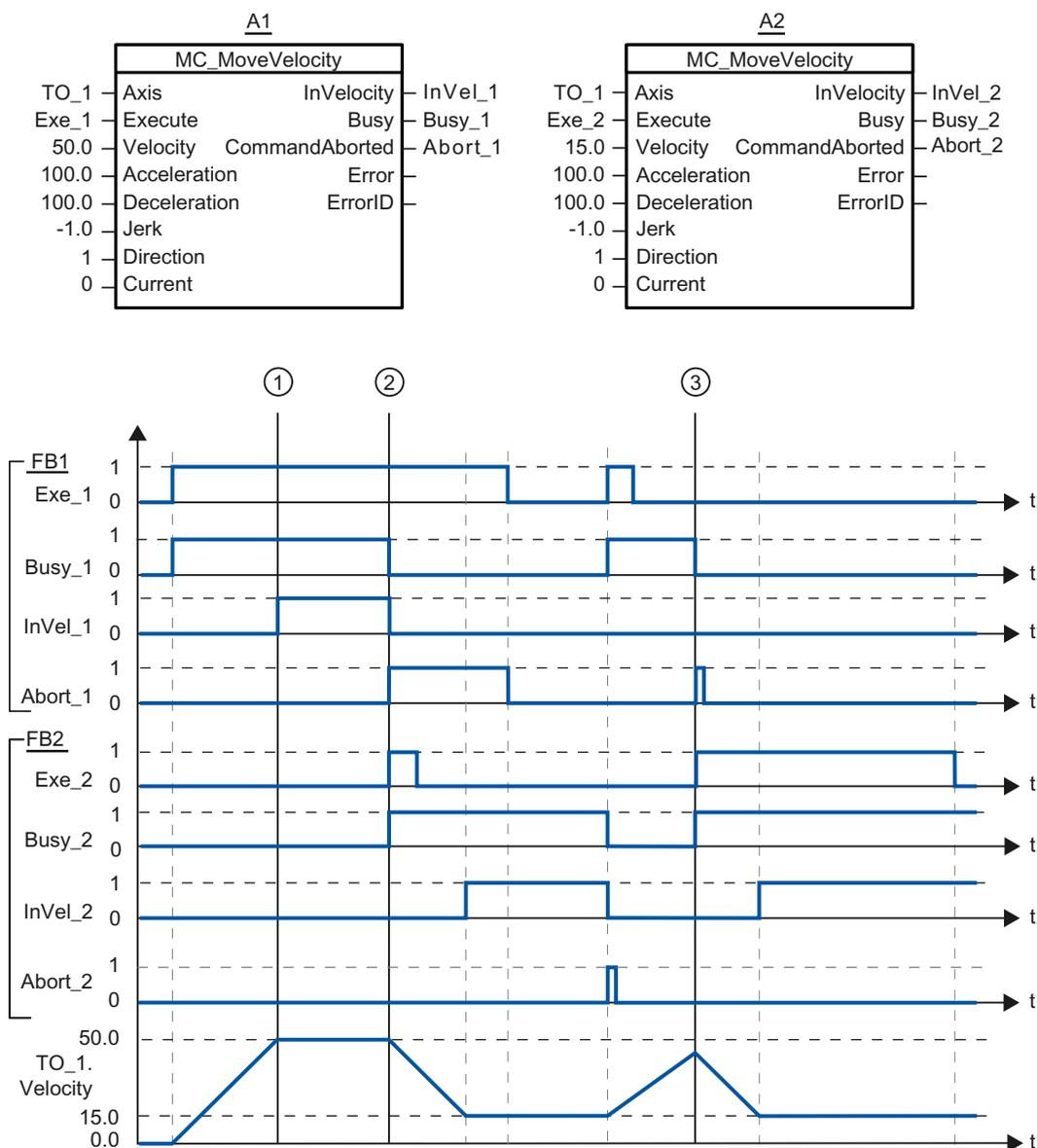
A "MC\_MoveVelocity" job (A1) initiated via "Exe\_1" accelerates the axis and signals at time ① via "InVel\_1" that the setpoint velocity 50.0 has been reached.
