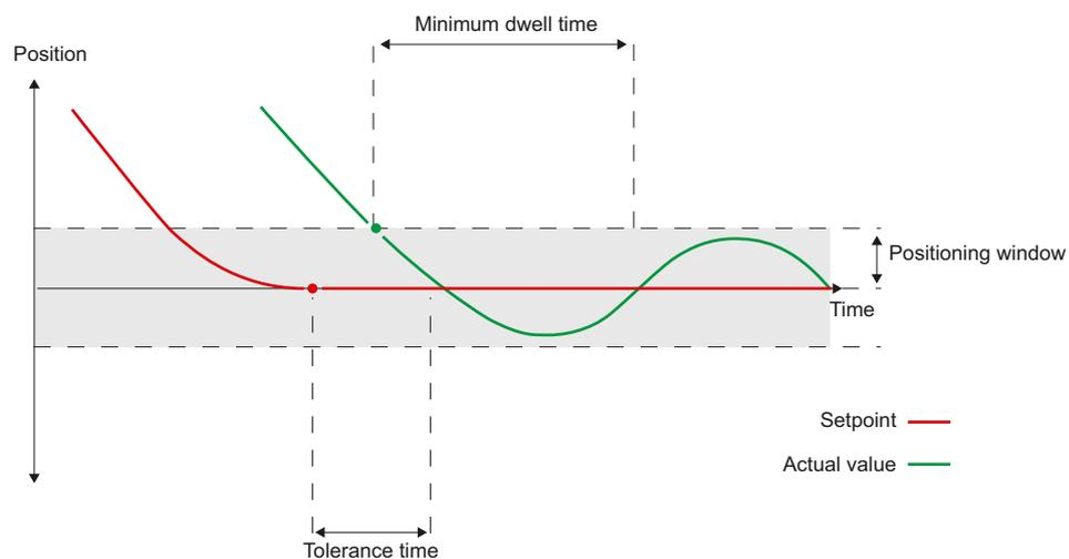
Positioning monitoring does not make any distinction between how the setpoint interpolation was completed. The end of setpoint interpolation can for example be reached as follows:
