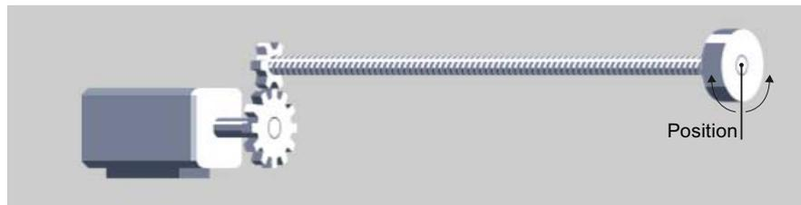
For rotary axes, the position of the axis is specified as an angular measure, e.g. degrees ( $^{\circ}$ ).
