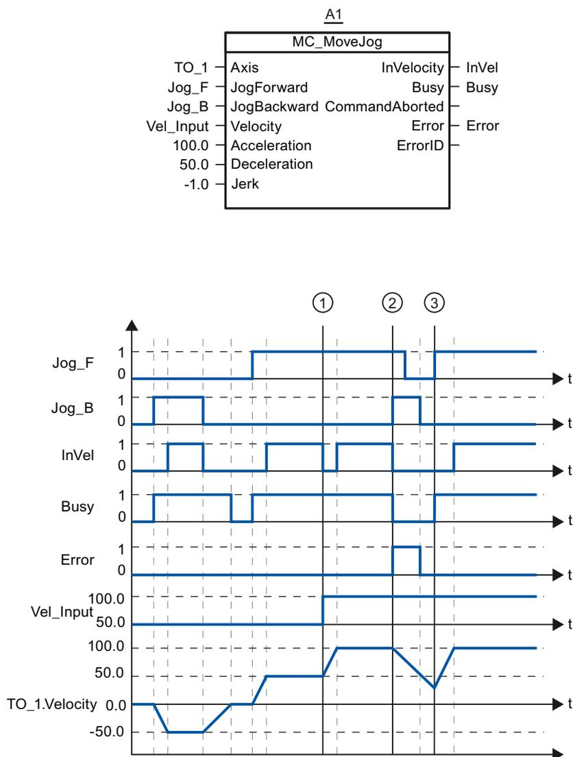
The axis is moved in the negative direction in jog mode via "Jog\_B". When the setpoint velocity -50.0 is reached, this is signaled via "InVel" = TRUE. After "Jog\_B" is reset, the axis is braked and brought to a standstill. Then the axis is moved in the positive direction via "Jog\_F". When the setpoint velocity 50.0 is reached, this is signaled via "InVel" = TRUE.
