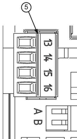
Figure 2-9 Remote contact for 6EP3333-8SB00-0AY0 and 6EP3334-8SB00-0AY0
