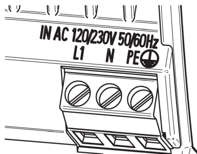
Figure 5-1 Line connection for 6EP3333-8SB00-0AY0 and 6EP3334-8SB00-0AY0
