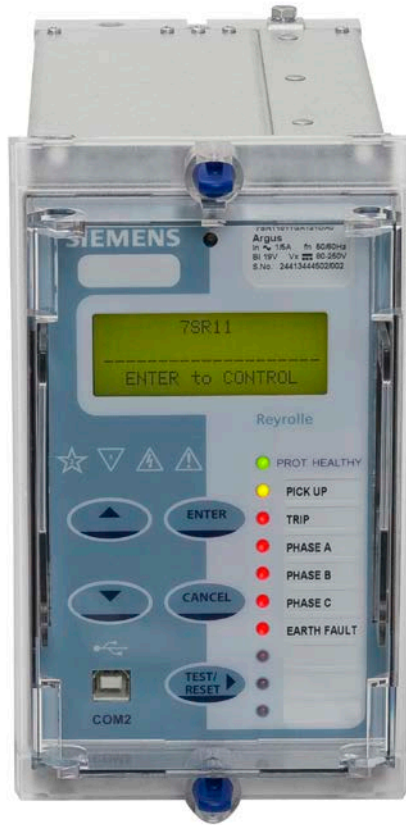
Figure 1.1-3 Fascia of a 7SR11 relay (E4 Case)
