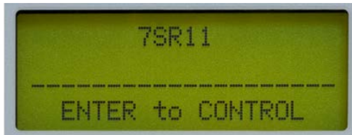
Figure 2-8 Close up of Relay Identifier
