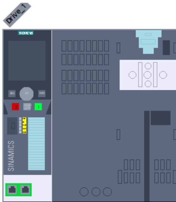
Figure 4-4: SINAMICS G120 hardware configuration
