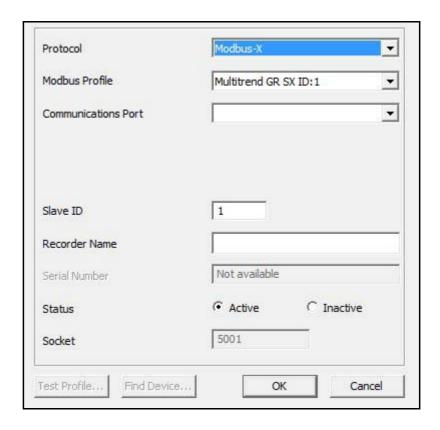
**Protocol** - For active Modbus devices, the recorder name and protocol variant can be changed (Modbus vs Modbus X). For an inactive Modbus device the device profile can also be changed.
