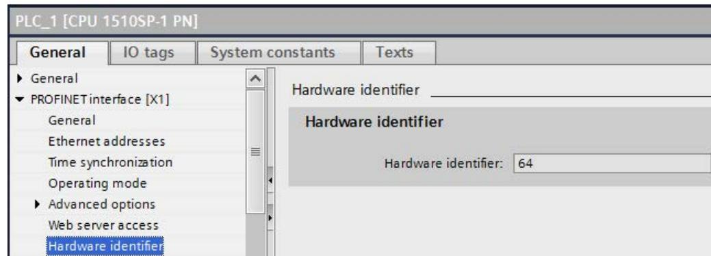
Figure 6-6 Example of a hardware identifier from STEP 7
