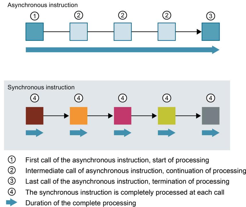
Figure 7-1 Difference between synchronous and asynchronous instructions
