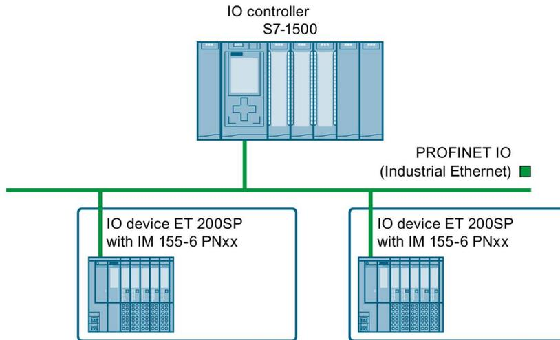
Figure 10-3 ET 200SP as an IO device
