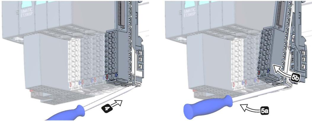
Figure 12-3 Replacing the terminal box on the BaseUnit
