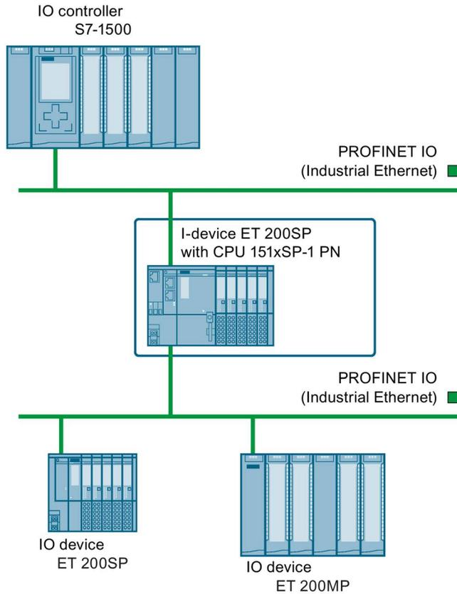
Figure 10-2 ET 200SP CPU as an I-device
