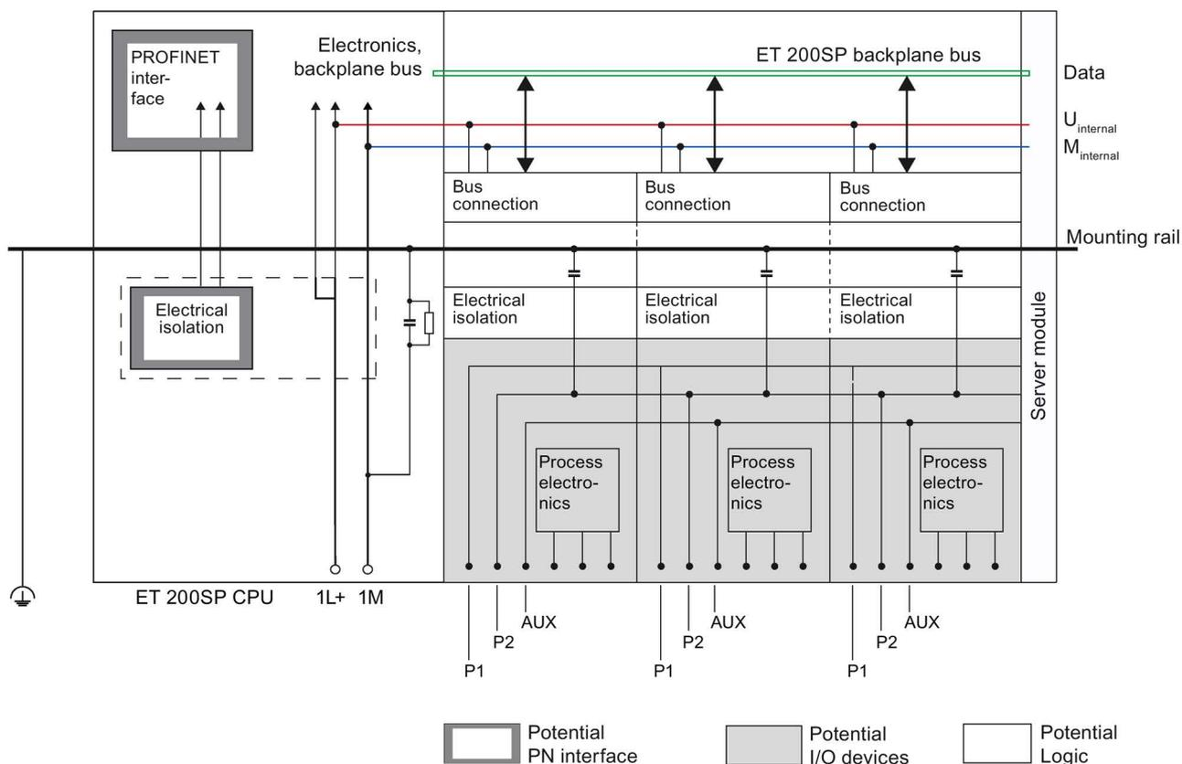
Figure 5-2 Electrical relationships for ET 200SP with CPU
