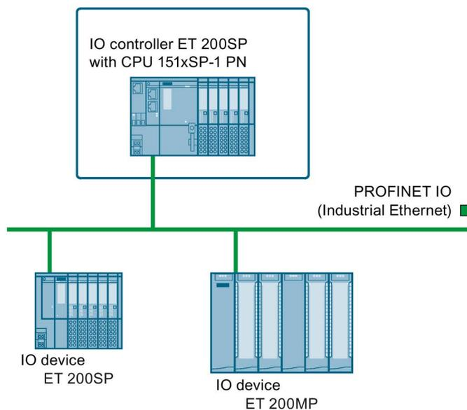
Figure 10-1 ET 200SP CPU as an IO controller
