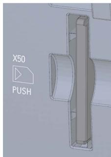
Figure 10-7 Slot for the SIMATIC memory card
