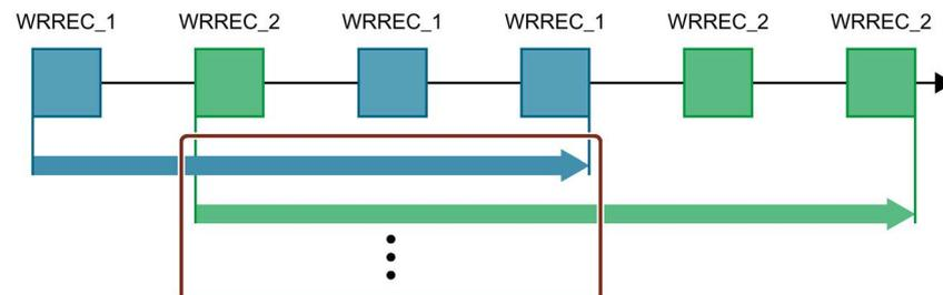
Figure 7-2 Parallel processing of the asynchronous instruction WRREC
