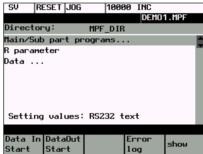
Fig. 5-2 RS232 text file screen (after entering machine tool manufacturer-specific password)
