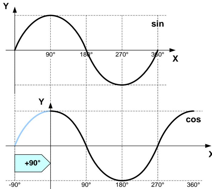
The curves for sinus and cosinus each have to be standardized for the range  $0 \leq X \leq 1$  in the trigonometric fraction of the segment. The function value of the two angle functions have to be in the range of  $-1 \leq Y \leq +1$ . Thus the following assignment results for the two missing parameters of the angle functions:
