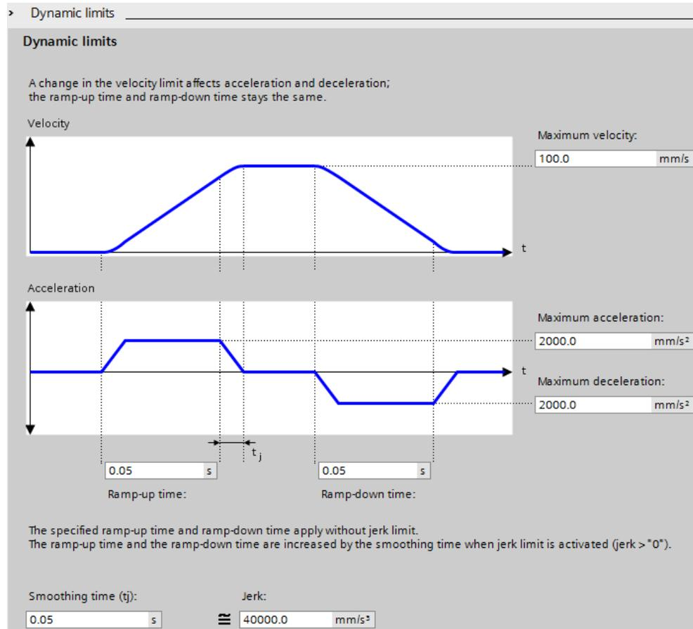
**CAUTION** If the motion of at least one axis is limited, this may cause a deviation of the desired trajectory. This is why you should make sure that the limitations of the traversing axes are not reached during the interpolated motion.
