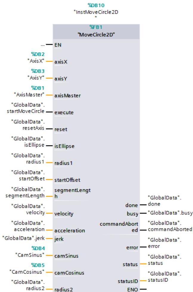
**Note** For each interpolated traversing motion with two axes that is performed in parallel to another interpolated traversing motion, you have to assign the “MoveCircle2D” function block to a separate instance data block or separate multi-instance.
