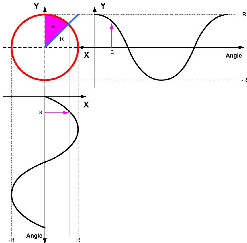
The overlapping of the two motions is based on the segment angle that is overswept when moving on the circular path. The angle count starts on the positive Y axis of the coordinate systems and runs in clockwise direction along the circular path. Depending on the size of the angle specification, either only a section of the circular arc is covered or up to several "revolutions" of the circle can be reached.
