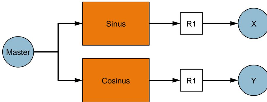
Sinus and cosinus are formed via the respective cam discs. The master axis provides the current angle as an input value. The multiplication of the output values of the cam discs with radius "R" of the circle is reached via scaling the slave values of the cam discs during synchronization via the technology function "MC\_CamIn".
