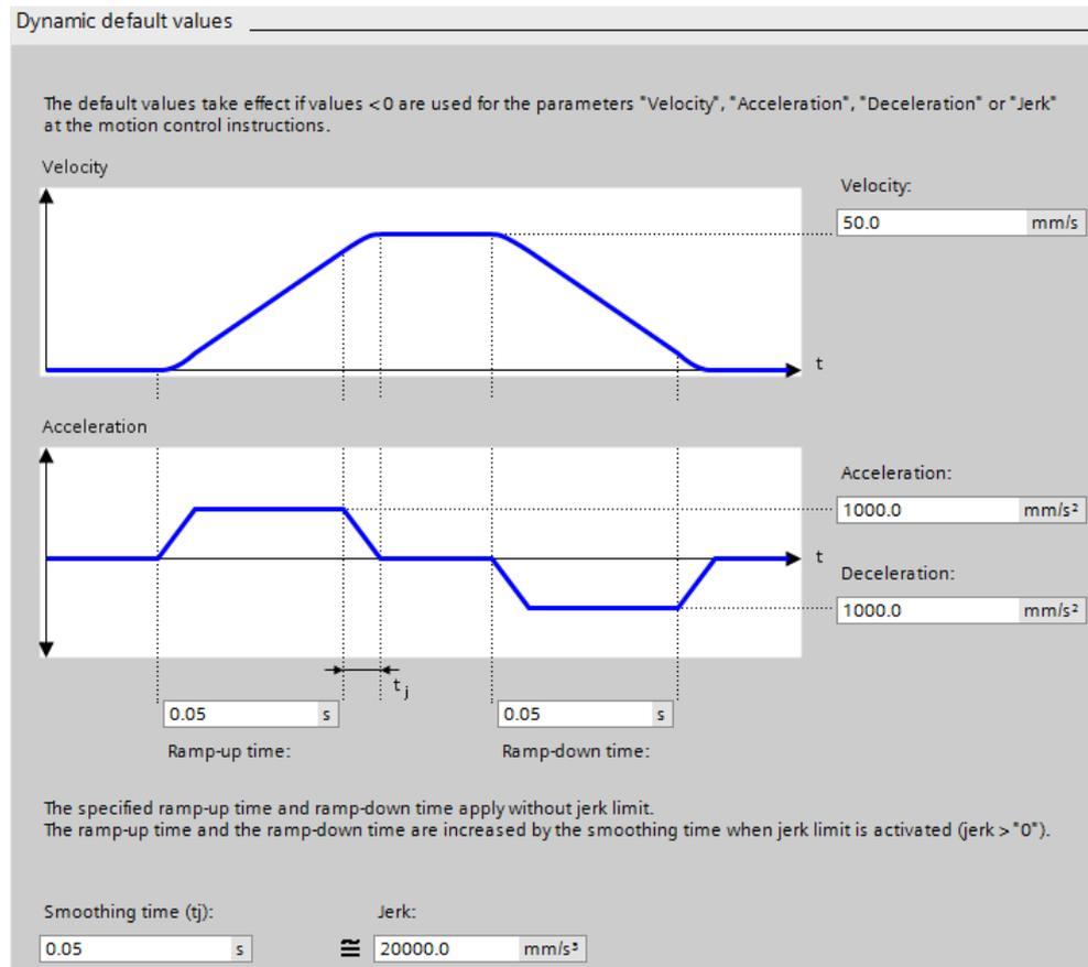
Adjust the settings to your application. The settings do not have an influence on the behavior of the axes during the interpolated motion.
