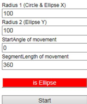
You can switch between circle and ellipsis, and specify the radius. The start angle and the segment length can also be specified. When you are clicking on the "Start" button, the cam discs are created and the execution of the interpolated motion is started.
