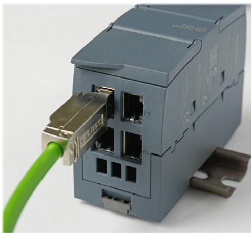
Figura 4-7 Enchufar el IE FC RJ45 Plug 180
