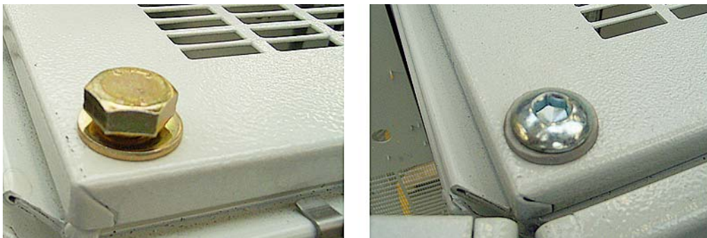
Figure 3-11 Delivery state (left), original roof screws (right)
