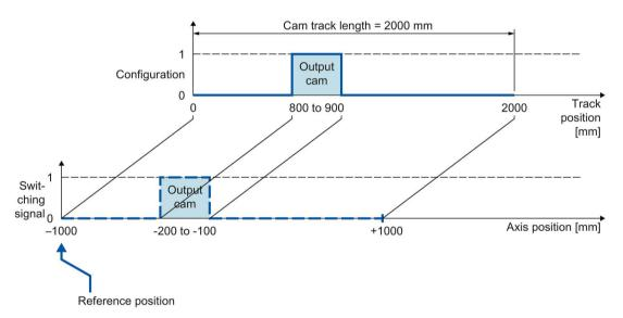
Figure 2-3 Cam track with output cam output at negative axis position
