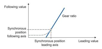
Gear ratio Slope of line/transmission ratio
