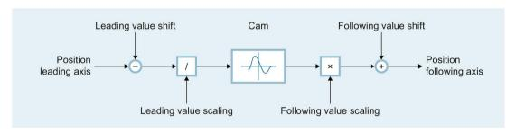
Position following axis = f[(Position leading axis - Leading value shift) / Leading value scaling] × Following value scaling + Following value shift
