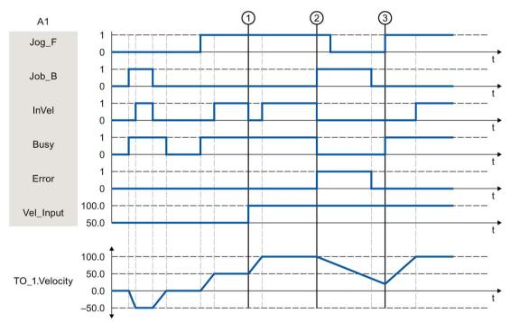
The axis is moved in the negative direction in jog mode via "Jog\_B". When the velocity setpoint -50.0 is reached, this is signaled via "InVel" = TRUE. After "Jog\_B" is reset, the axis is braked and brought to a standstill. Then the axis is moved in the positive direction via "Jog\_F". When the velocity setpoint 50.0 is reached, this is signaled via "InVel" = TRUE.
