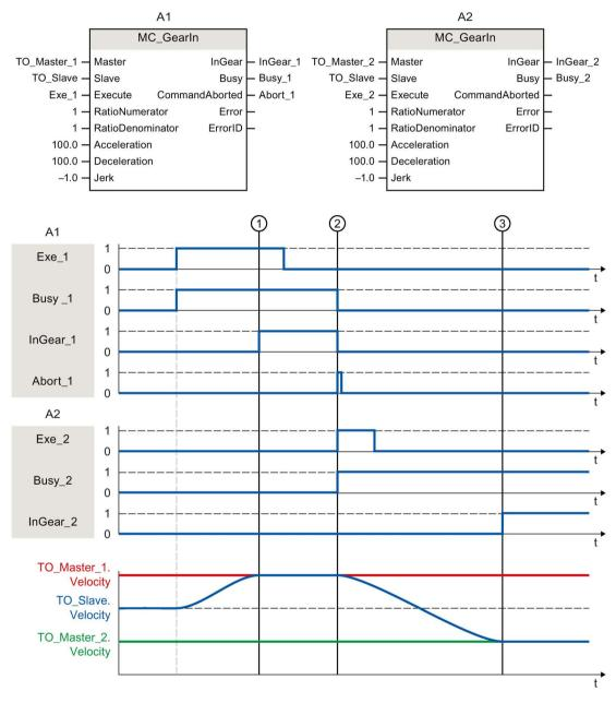
Using "Exe\_1", an "MC\_GearIn" job (A1) is initiated. The following axis (TO\_Slave) is synchronized to the leading axis (TO\_Master\_1). "InGear\_1" signals at time ① that the following axis is synchronized and moves synchronously to the leading axis.
