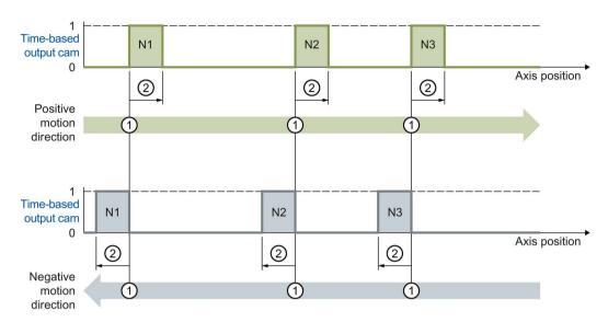
Figure 2-6 Executing a cam track with time-based output cams dependent on the motion direction of the axis
