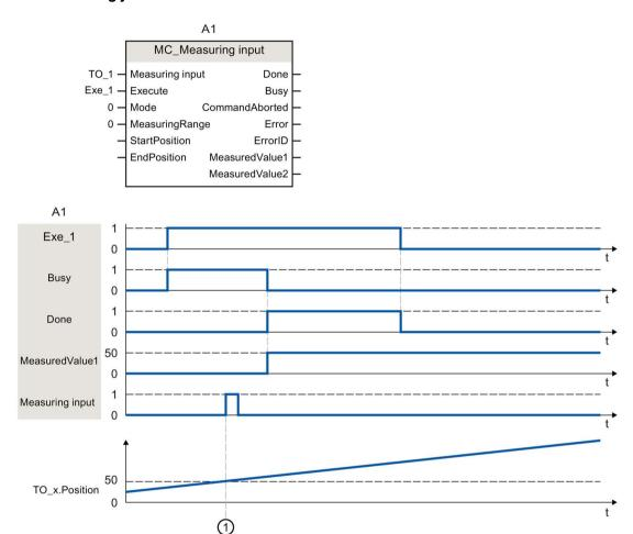
A "MC\_MeasuringInput" job with "Mode" = 0 initiated using "Execute" performs a measurement of the next positive edge. A successfully completed measurement is signaled with "Done" = TRUE. The determined measured value ① (in example: 50) is output using "MeasuredValue1".
