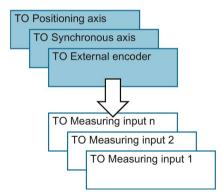
Exactly one axis or one external encoder can be assigned to a measuring input technology object.
