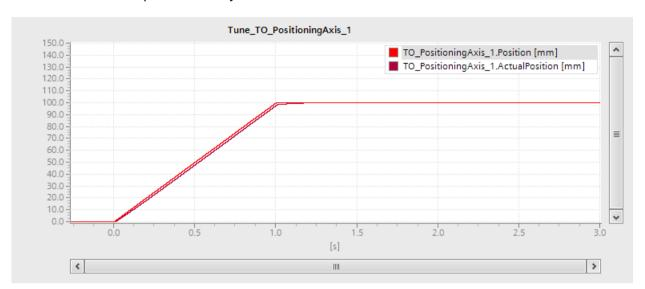
The following trace recording shows a curve in which the gain is optimal and the overall response is steady:
