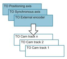
Exactly one axis or one external encoder can be assigned to a cam track.
