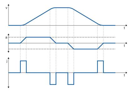
A velocity profile with jerk limitation is employed for a continuous acceleration and deceleration sequence. The jerk can be specified.
