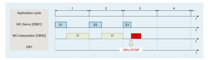
The CPU tolerates a maximum of three consecutive overflows of MC-Interpolator [OB92]. If more overflows occur, the CPU switches to STOP mode.
