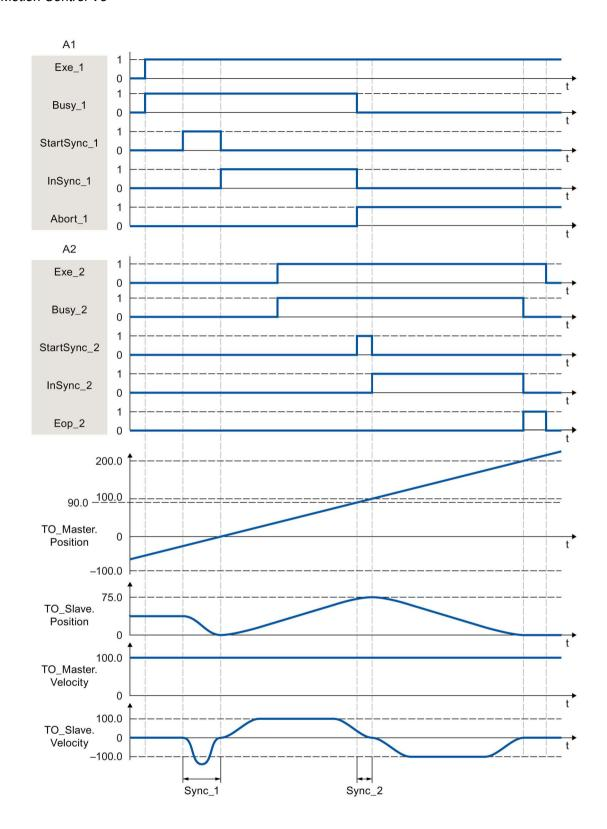
Using "Exe\_1", an "MC\_CamIn" job (A1) is initiated. The start of the synchronization is displayed with StartSync\_1. The following axis (TO\_Slave) is synchronized to the cam (Cam\_1) within the range "Sync\_1" by means of the specified dynamic parameters. "InSync\_1" signals that the following axis is synchronized and moving synchronously to the leading axis.
