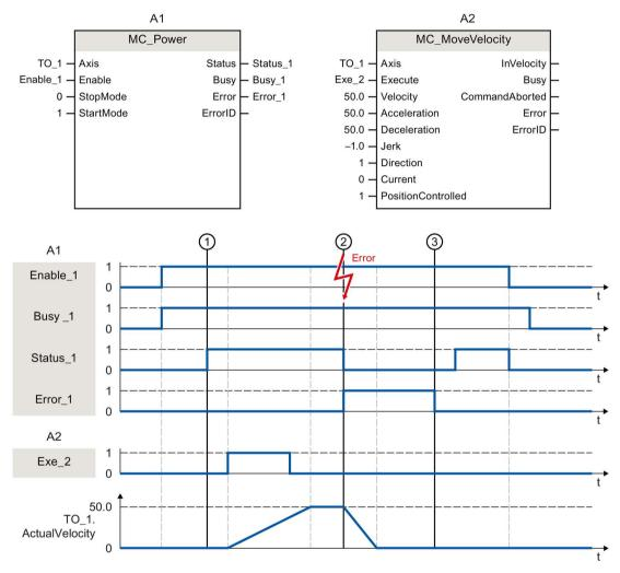
A technology object is enabled with "Enable\_1= TRUE". The successful enable can be read from "Status\_1" at time ①. The axis will then move with an "MC\_MoveVelocity" job (A2). The velocity profile of the axis can be read from "Velocity Axis\_1".
