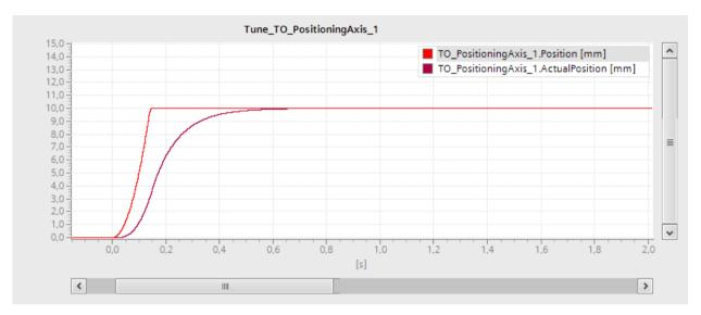
The following trace recording shows a curve with overshoot when approaching the setpoint:
