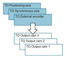
Exactly one axis or one external encoder can be assigned to an output cam.
