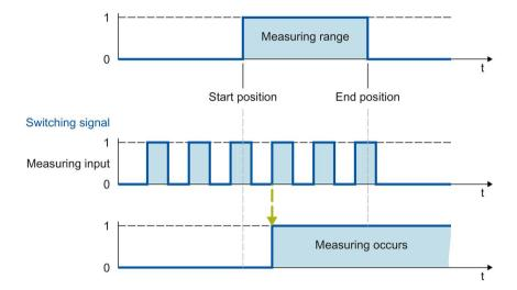
Figure 2-1 Example of measuring with measuring range in Mode = 0 (measurement of next positive edge)
