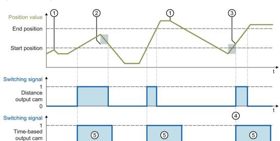
The following examples show the effects of the hysteresis on the switching behavior of output cams with positive activation direction.
