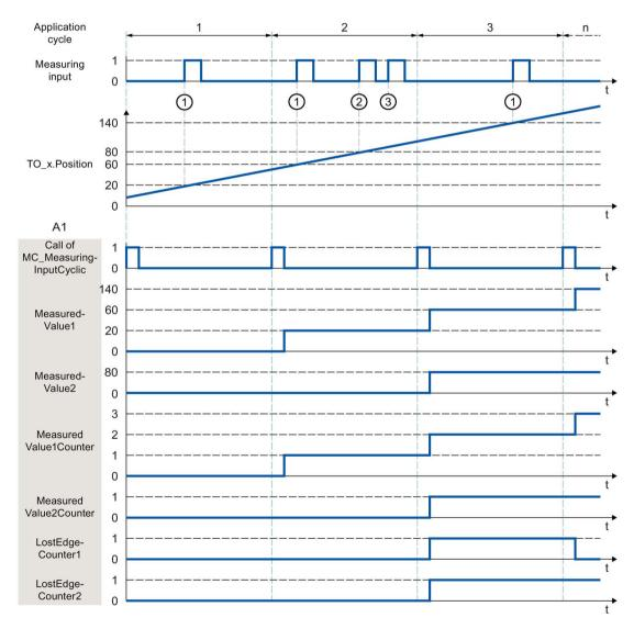
A "MC\_MeasuringInputCyclic" command initiated using "Execute" (signal and start point not shown) (e.g. call in MC-PreServo [OB67]) with "Mode" = 0 and without specified measuring range "MeasuringRange" = FALSE performs a measurement of the positive edges. By
