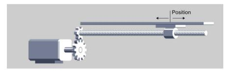
For linear axes, the position of the axis is specified as a linear measure, e.g. millimeters (mm).
