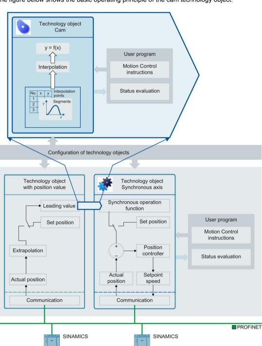
The figure below shows the basic operating principle of the cam technology object:
