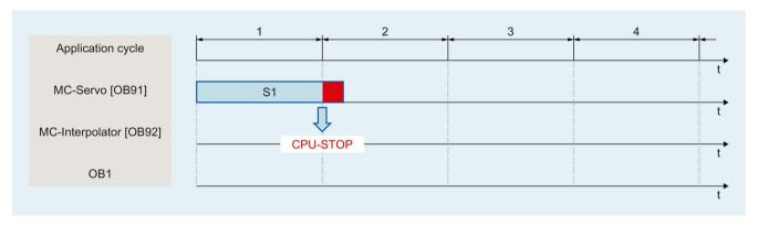
The execution of an MC-Interpolator [OB92] may only be interrupted by an MC-Servo [OB91] call. If more interruptions occur, the CPU switches to STOP mode.
