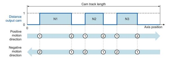
Figure 2-5 Executing a cam track with distance output cams dependent on the motion direction of the axis
