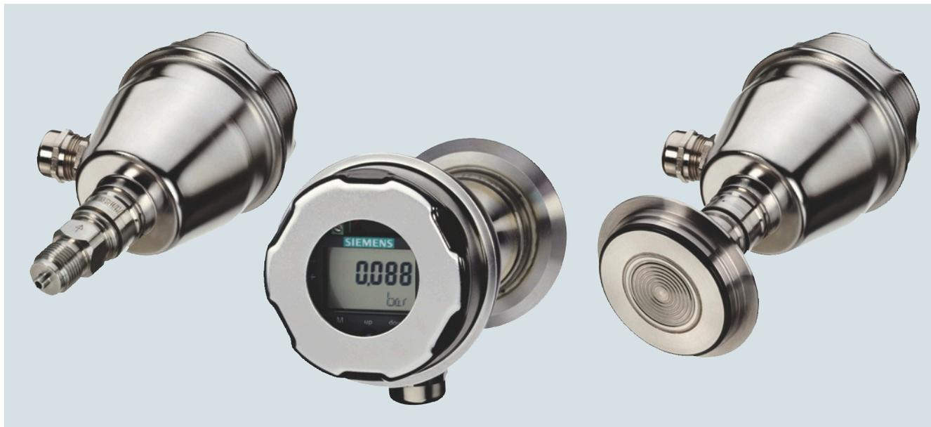
The SITRANS P300 is a digital pressure transmitter for relative and absolute pressure. The conventional thread versions are available as process connections, as are flush-mounted versions. A large number of the flush-mounted versions are suitable for food and pharmaceutical applications, and satisfy the EHEDG and 3A hygiene requirements.
