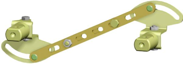
Mechanical interlocking make sure that two circuit breakers cannot trip simultaneously, but always just individually. Both circuit breakers may be switched off simultaneously. Interlocking can be used between two 3VT2 circuit breakers or between one 3VT2 and one 3VT3 circuit breaker. Both circuit breakers must be furnished with rotary operating mechanisms (at least one of them with a rotary operating mechanism and knob).
