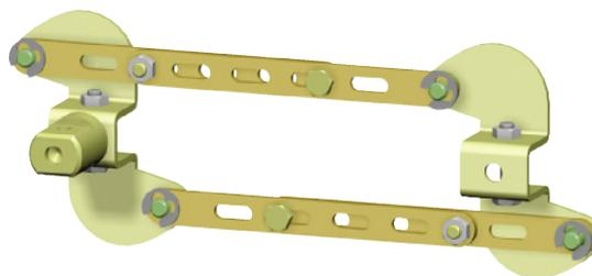
Mechanical interlocking for parallel switching are for simultaneous switching of two circuit breakers. Parallel switching can be used between two 3VT3 circuit breakers or between 3VT3 and 3VT2 circuit breakers. Each circuit breaker must be furnished with a rotary operating mechanism and at least one of them with a knob.
