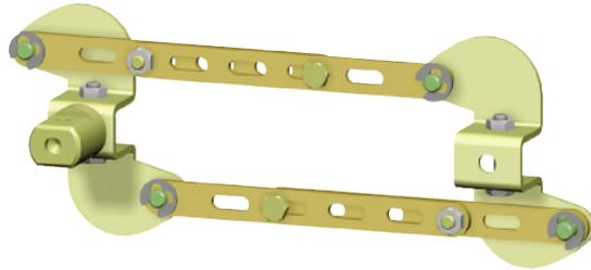
Mechanical interlocking for parallel switching are for simultaneous switching of two circuit breakers. Parallel switching can be used between two 3VT2 circuit breakers or between 3VT2 and 3VT3 circuit breakers. Each circuit breaker must be furnished with a rotary operating mechanism and at least one of them with a knob.
