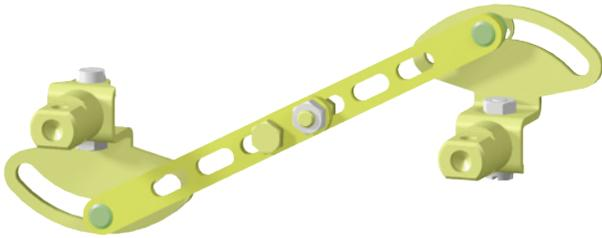
Mechanical interlocking make sure that two circuit breakers can not trip simultaneously, but always just individually. Both circuit breakers may be switched off simultaneously. Interlocking can be used between two 3VT1 circuit breakers. Each circuit breaker must be furnished with a rotary operating mechanism – at least one of them with a rotary operating mechanism and a knob (see page 1/25).
