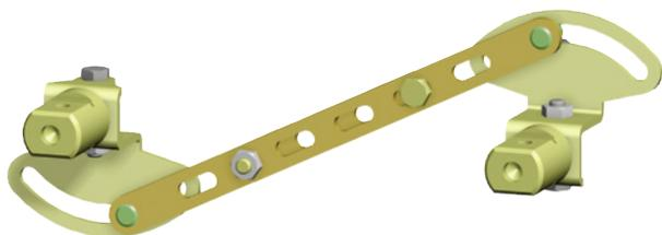
Mechanical interlocking make sure that two circuit breakers cannot trip simultaneously, but always just individually. Both circuit breakers may be switched off simultaneously. Interlocking can be used between two 3VT3 circuit breakers or between one 3VT3 and one 3VT2 circuit breaker. Both circuit breakers must be furnished with rotary operating mechanisms (at least one of them with a rotary operating mechanism and knob).
