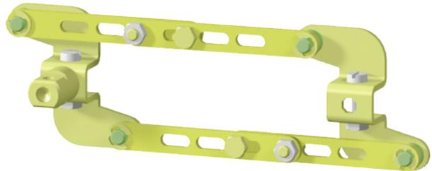
Mechanical interlocking for parallel switching are for simultaneous switching of two circuit breakers. Parallel switching can be used between two 3VT1 circuit breakers. Each circuit breaker must be furnished with a rotary operating mechanism and at least one of them with a knob (see page 1/25).
