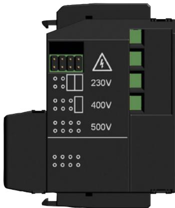
The particular rated operating voltage of the shunt trip unit is set up by jumpers located on the right hand side in the trip unit. Default setting is always the maximum value.
