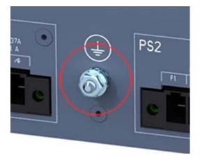
Grounding bolts on the underside of the housing of the X-300EEC or on the rear of the XR-300M-EEC
