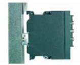
Figure 5-1 Mounting an IE Switch X-300 on a DIN rail (35 mm)
