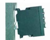
Figure 5-2 Removing an IE Switch X-300 from a DIN rail (35 mm)
