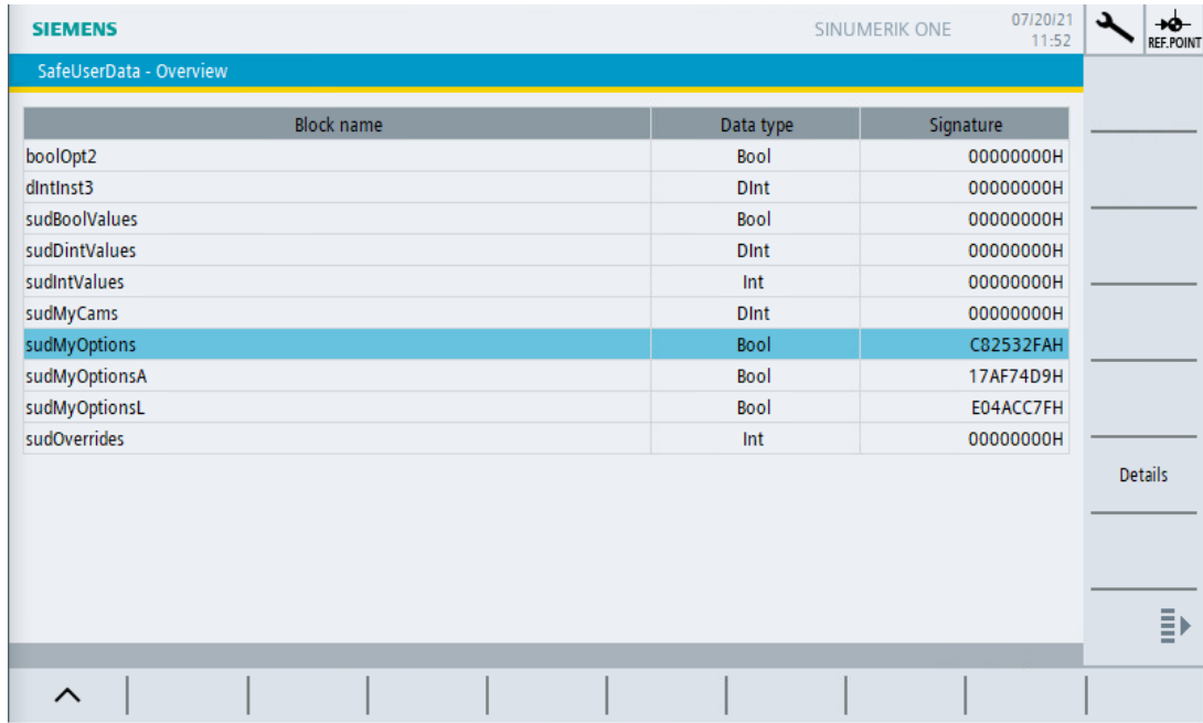
Figure 7-19 SINUMERIK ONE example: SafeUserData - Block overview
