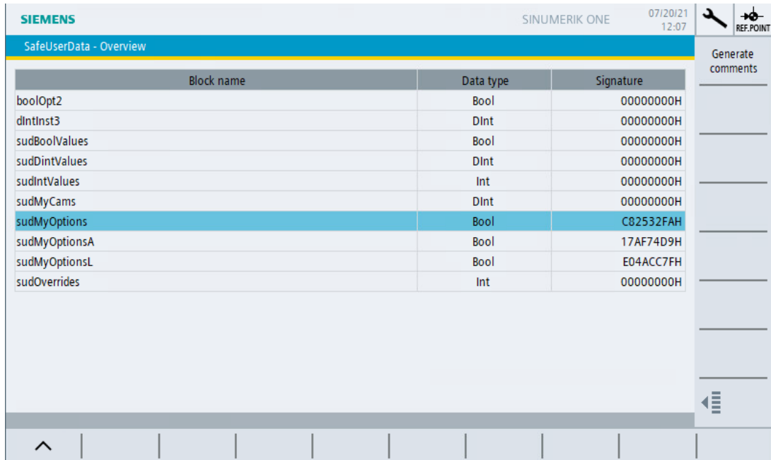
Figure 7-27 SafeUserData - Generating overview with softkey comments
