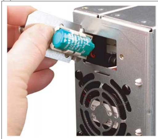
Figure 19-30 Removing the battery holder
