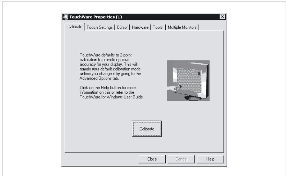
Figure 19-17 Menu for touch screen calibration (Touchware version 5.64 SR3)
