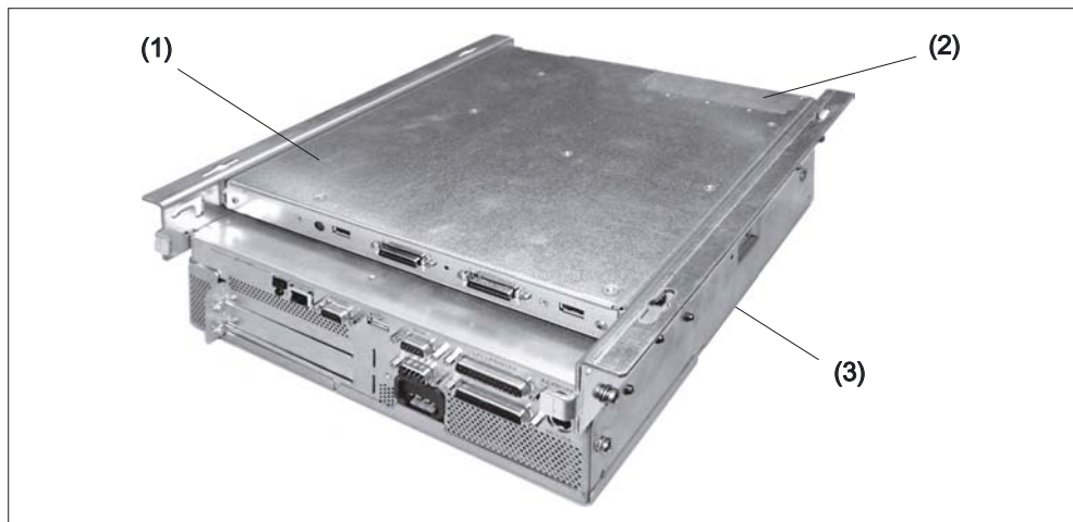
Figure 21-13 PCU/transmitter unit assembled for "flat" mounting
