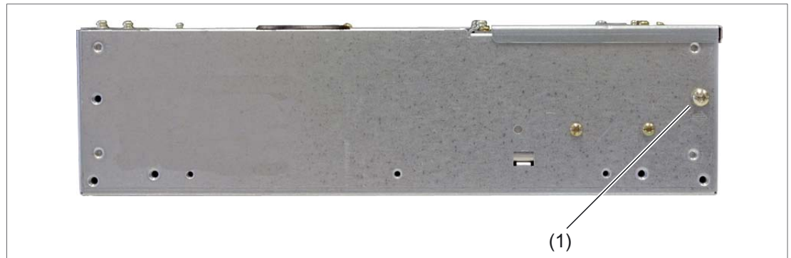
Figure 19-13 Underside of PCU 50.3
