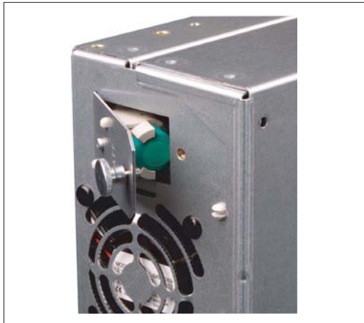
Figure 19-29 Opening the battery compartment
