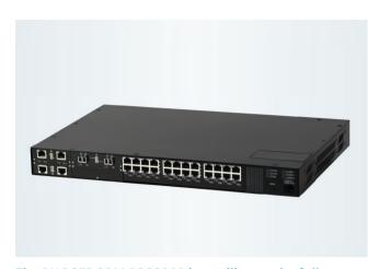
The RUGGEDCOM RSG2300 is a utility-grade, fully managed, 32-port modular Ethernet switch specifically designed to operate reliably in electrically harsh and climatically demanding environments.
