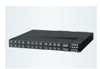
The RUGGEDCOM RSG2488 is a utility-grade, field upgradable, fully managed, 28-port Gigabit Ethernet switch with hot-swappable dual redundant power supplies and full support for IEEE1588 precision timing protocol. It is specifically designed to operate reliably in electrically harsh and climatically demanding environments.
