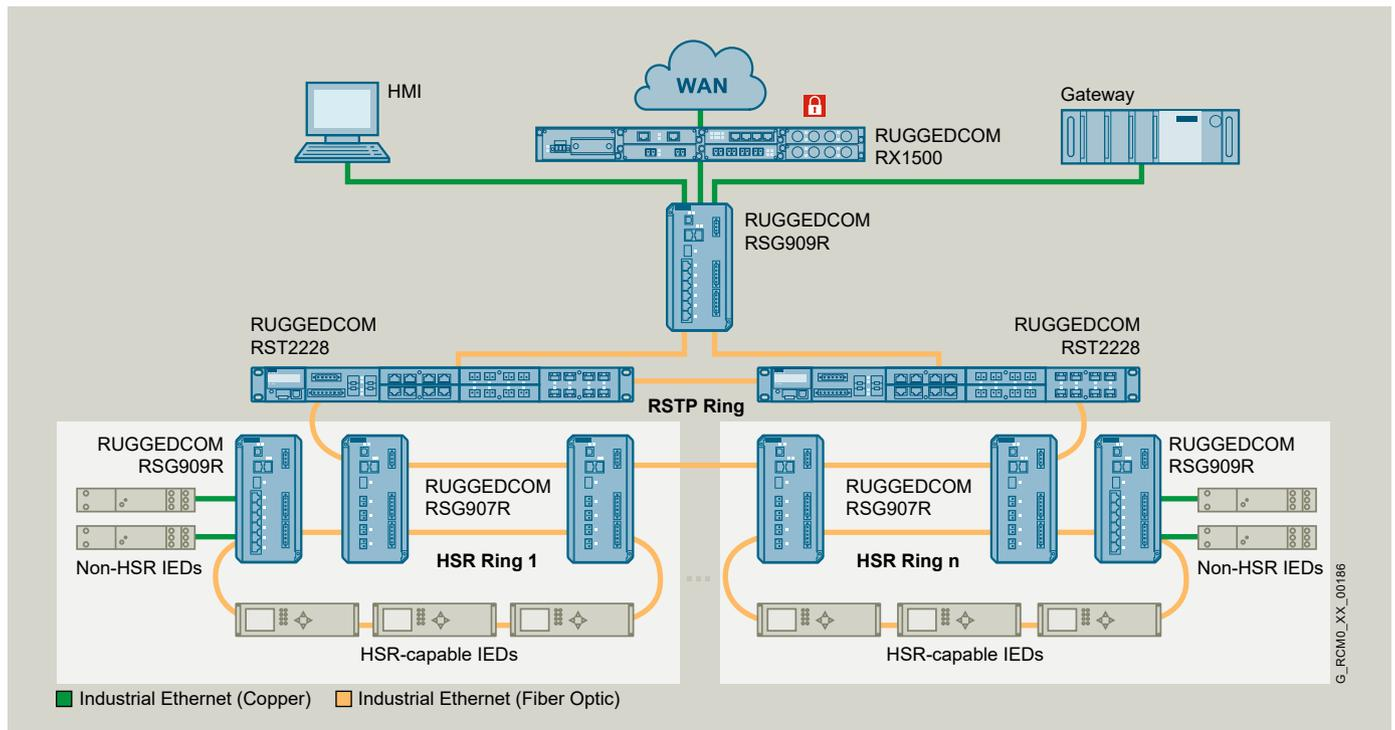
RUGGEDCOM RSG907R/RSG909R switches terminating each HSR ring can be directly connected to an RSTP network via their coupling ports.
