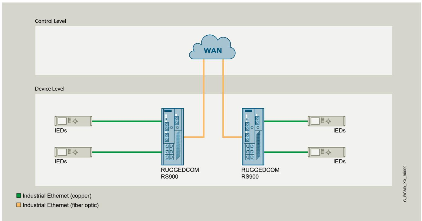
The RUGGEDCOM RS900 makes it possible to remotely monitor field data using multiple types of communications.
