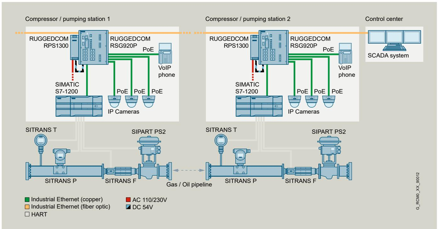
The RUGGEDCOM RSG920P is ideal for the field level where growing demands for Ethernet connectivity exist.
