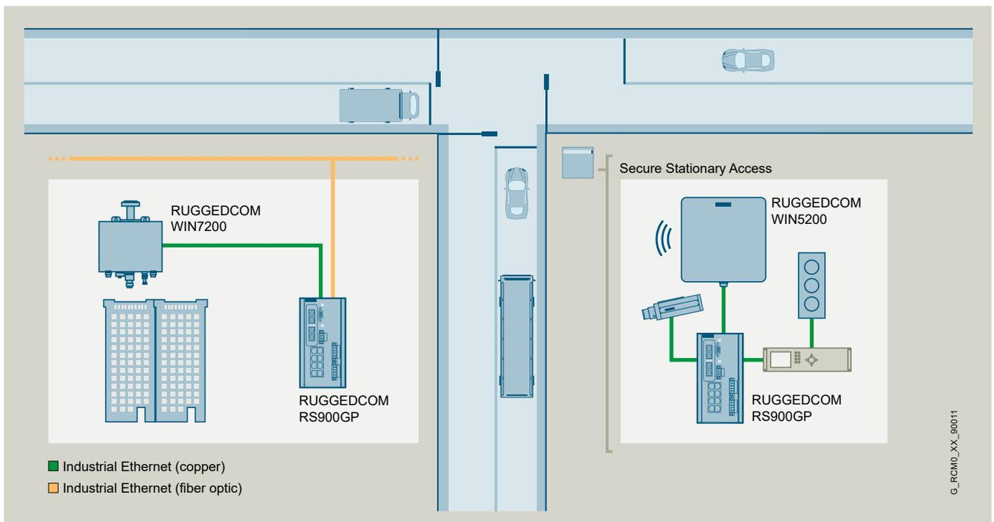
Multiple Power-over-Ethernet devices are powered by the RUGGEDCOM RS900GP in the field.
