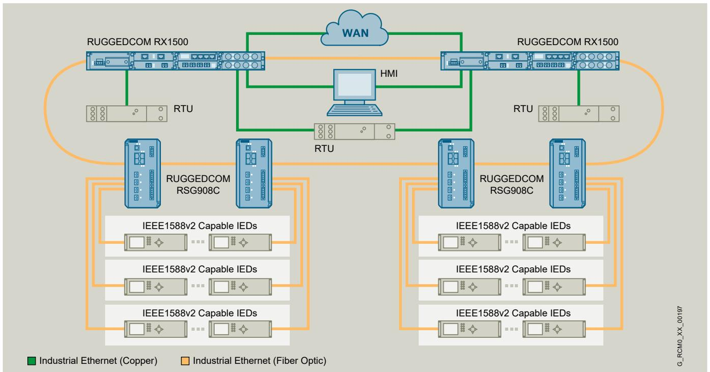
The RUGGEDCOM RSG908C allows the aggregation of large fiber optic 100BASE-FX subrings of IEDs at protection bays into 1 Gbps fiber optic rings while providing IEEE 1588 timing.
