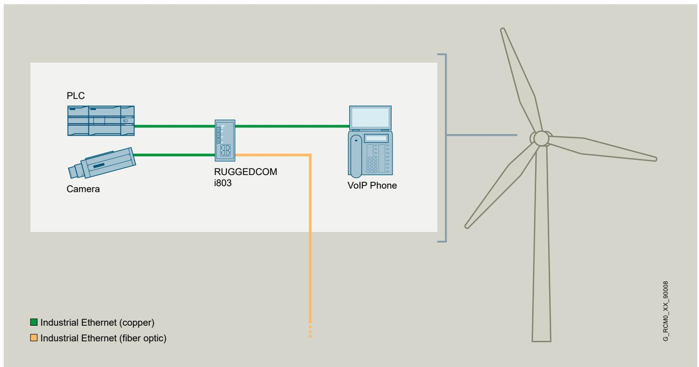
Inside the nacelle of a wind turbine, the RUGGEDCOM i802 enables connectivity for up to 6 Ethernet devices over copper and a backhaul over fiber-optic.
