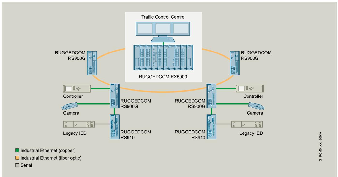
A reliable eRSTP ring network with Gigabit bandwidths can be achieved with the RUGGEDCOM RS900G.
