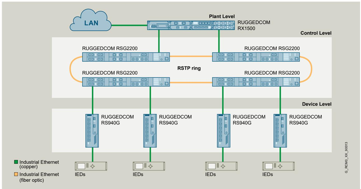
The RUGGEDCOM RS940G can connect up to 8 devices with Gigabit speeds on the device level.
