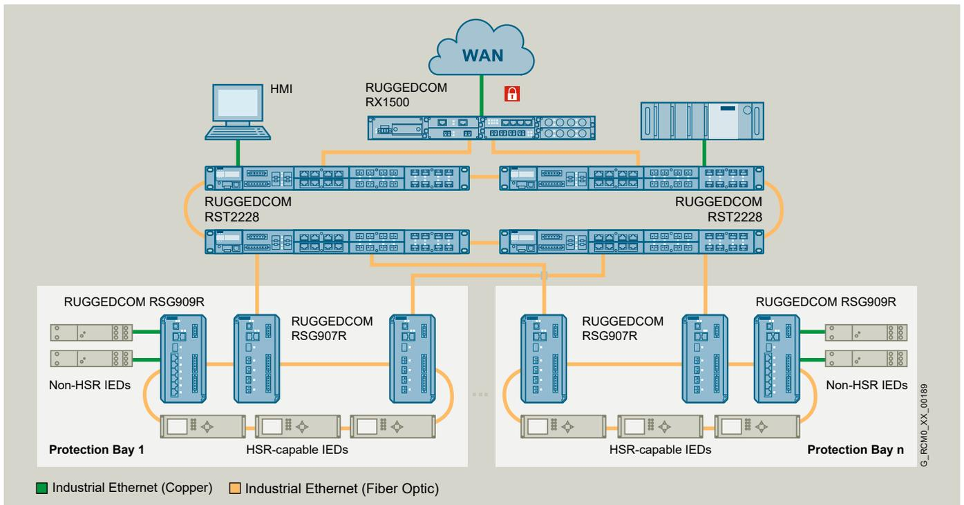
Two RUGGEDCOM RSG907R/RSG909R are used in each HSR bay ring for redundant coupling with PRP station level LANs.
