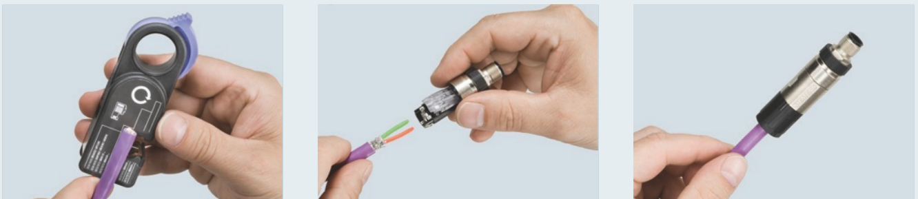
Stripping and assembly with M12 plug-in connector
