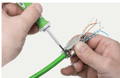
Fasten the casing using a screwdriver
