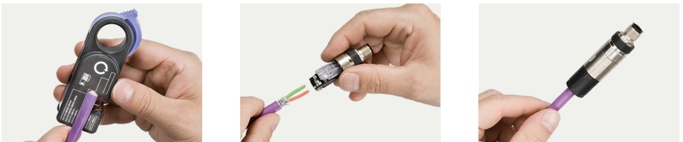
Stripping and assembly with M12 plug-in connector
