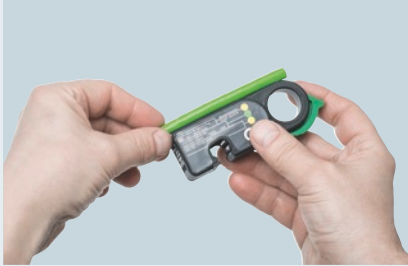
Measure the cable end
