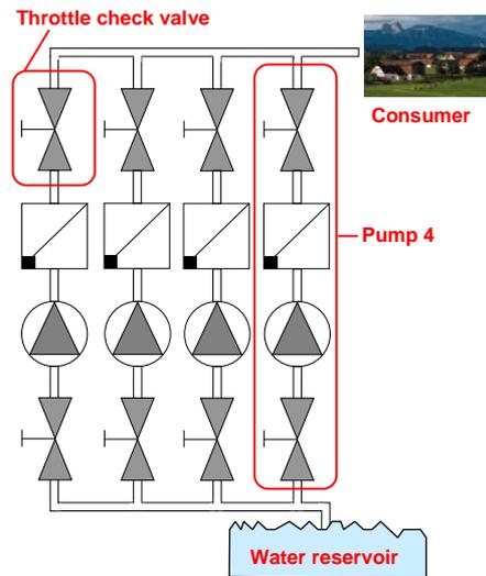
The delivery height  $H$  of each pump depends on the conveying current  $Q$ . Figure 1-4 shows how the delivery height is increased for a quadrupled conveying current when cascading 4 pumps.
