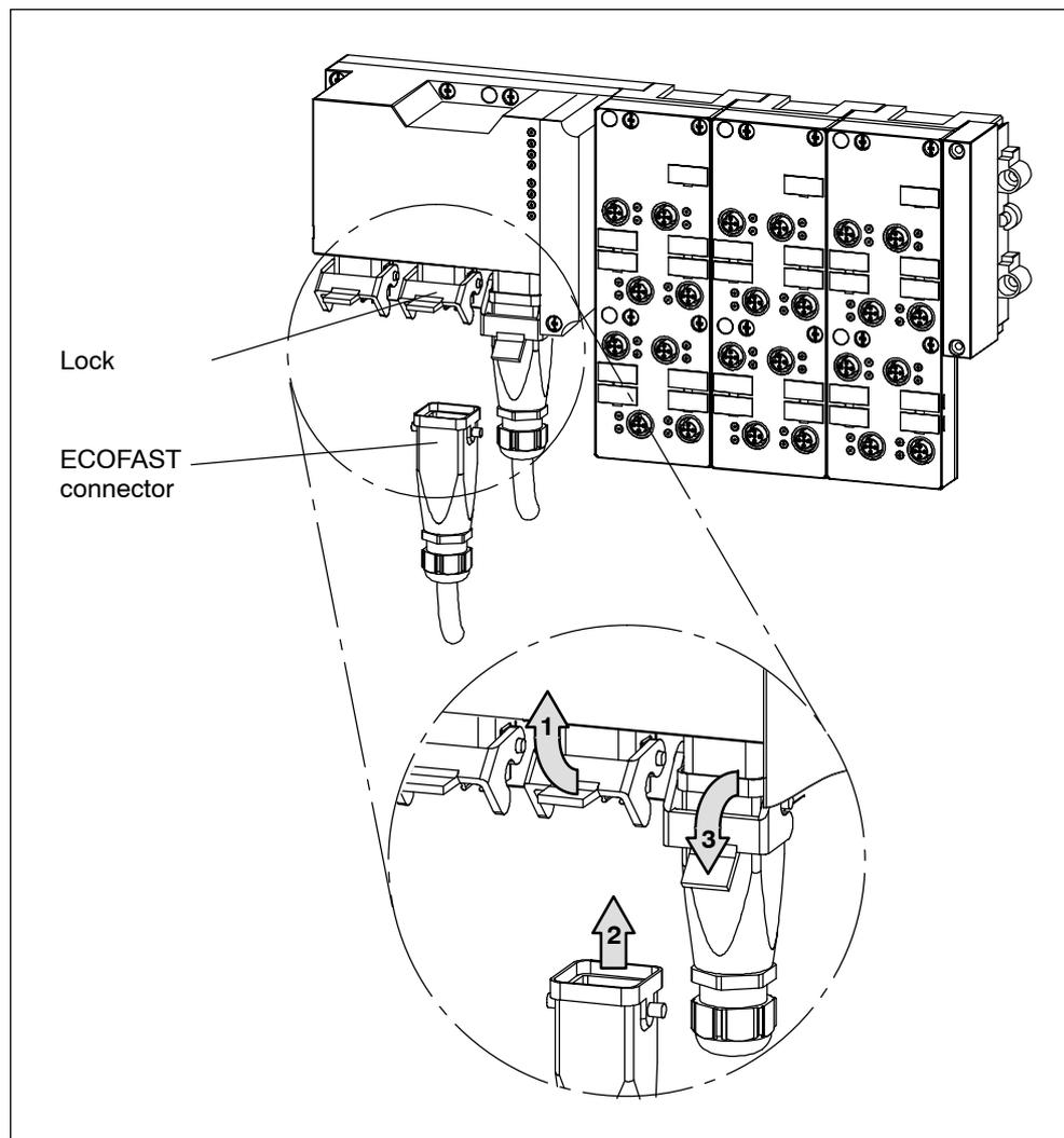
Figure 5-3 Plugging the connector into the BM 147 CPU
