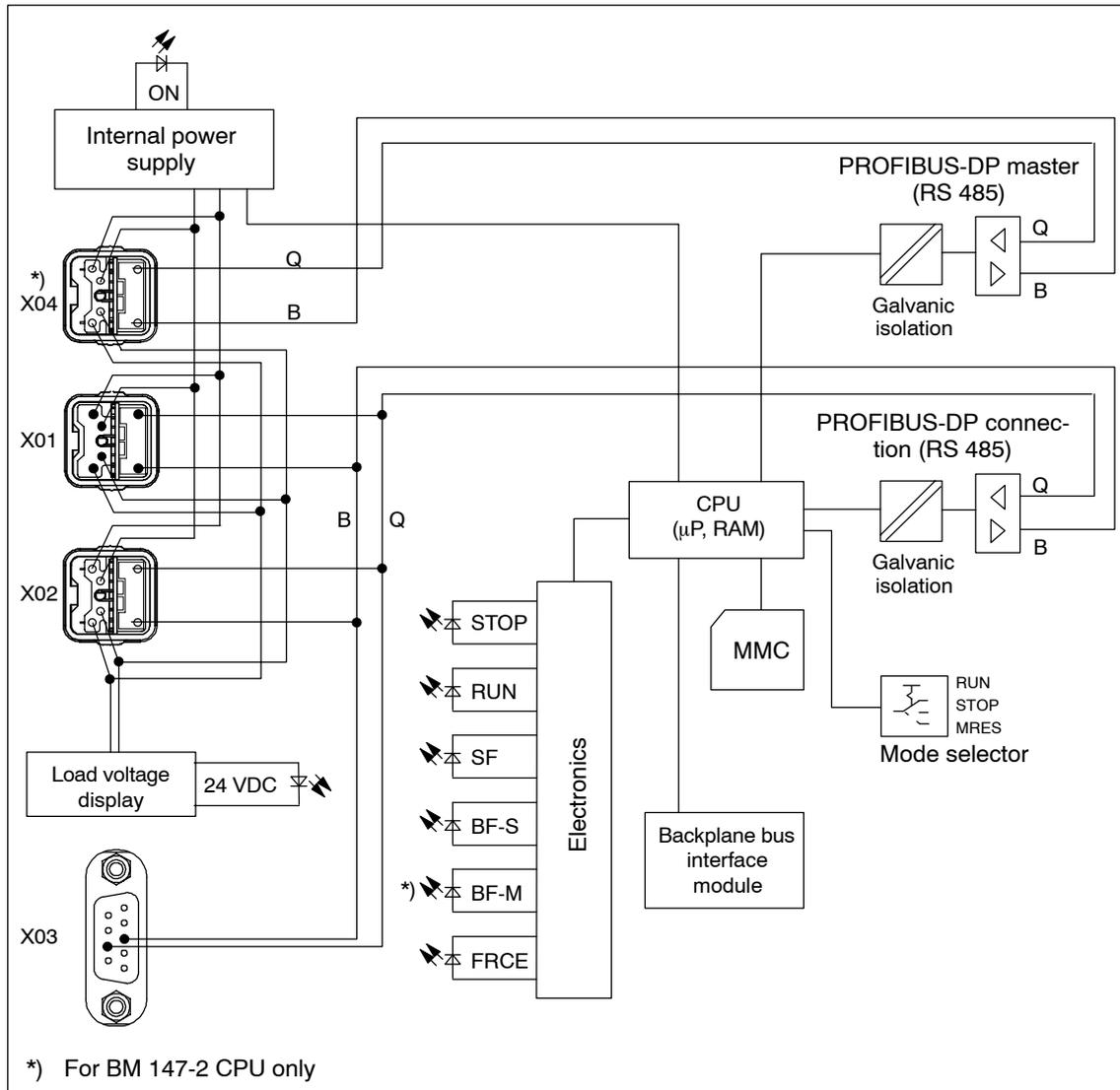
Figure 9-1 Block diagram BM 147 CPU
