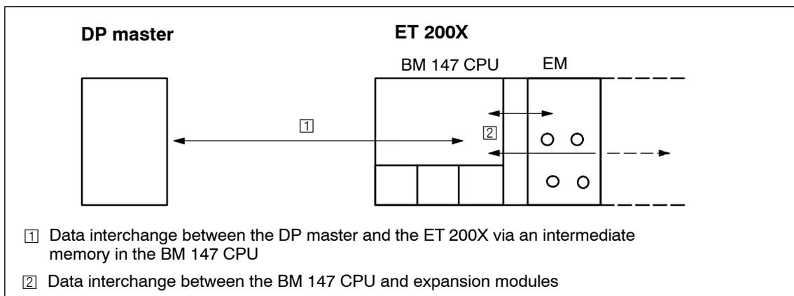
Figure 2-1 Principles of data interchange between the DP master and the ET 200X with the BM 147 CPU
