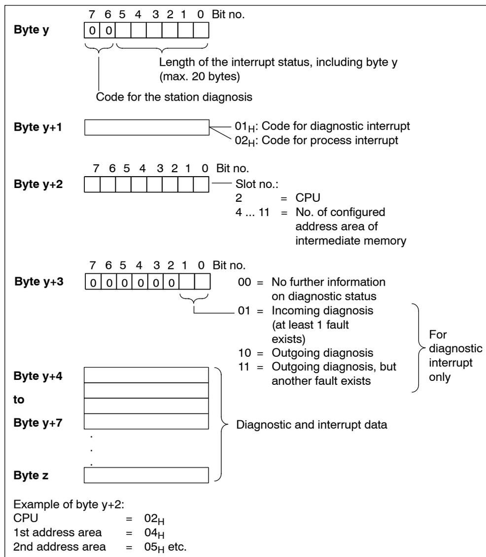
Figure 6-7 Structure of the interrupt status
