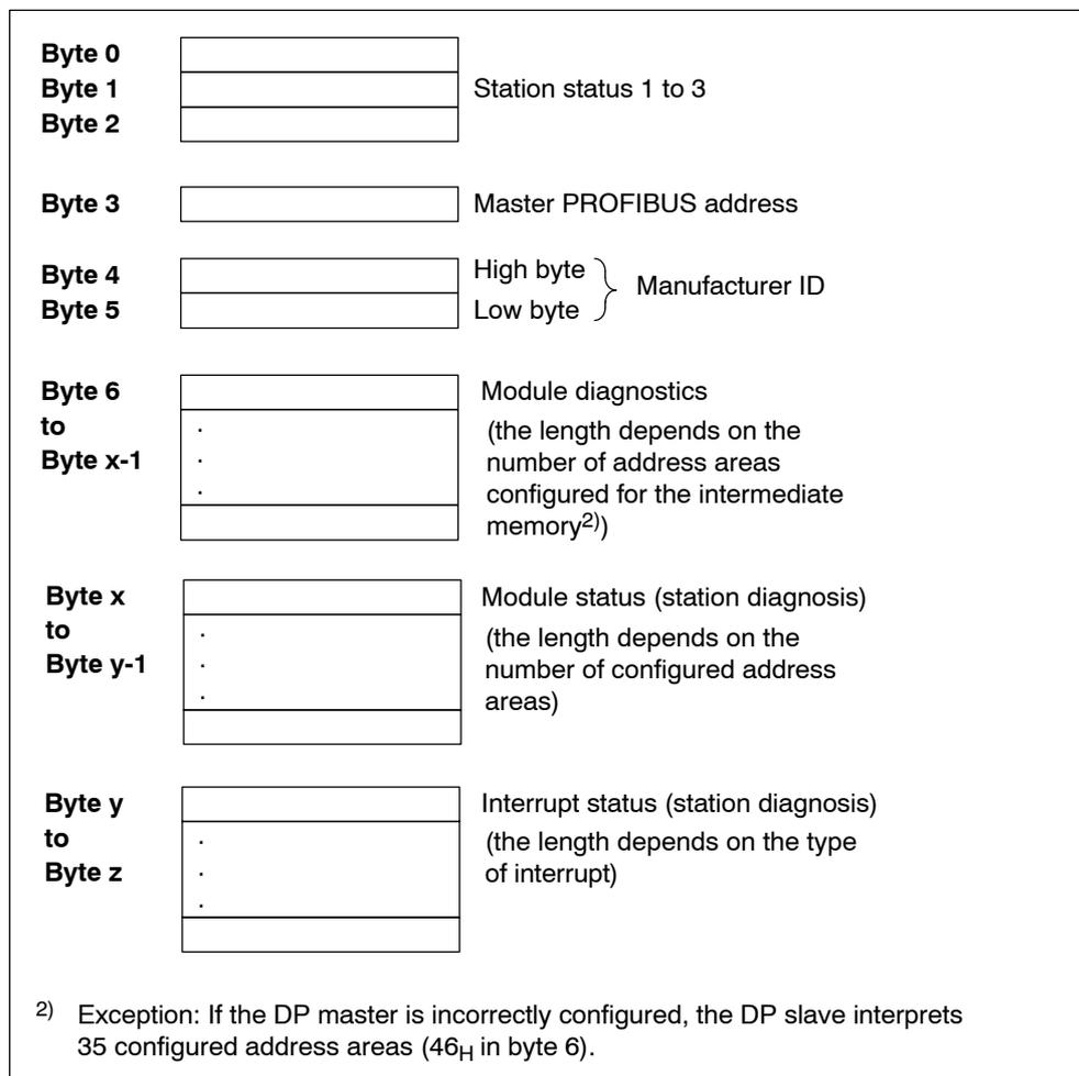
Figure 6-4 Format of the slave diagnostic data
