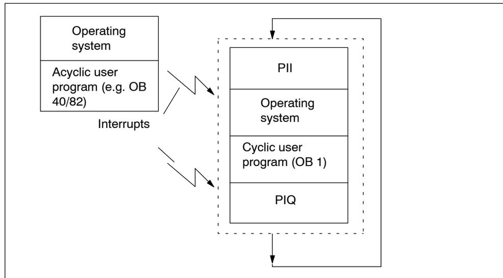
Figure 8-1 Component parts of the cycle time
