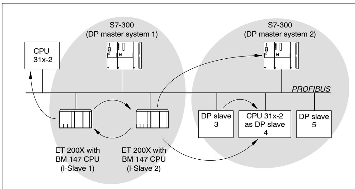
Figure 3-7 Direct communication with the BM 147 CPU
