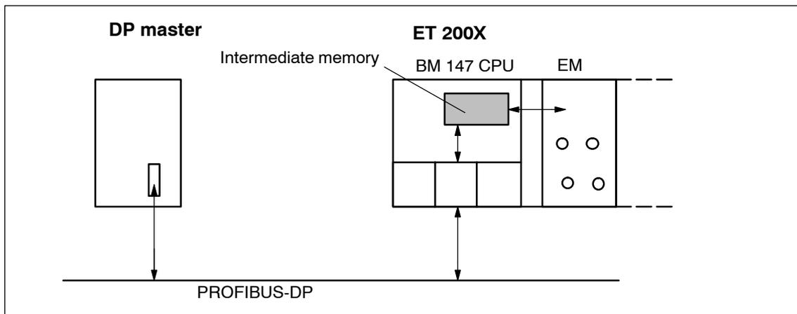
Figure 2-6 Intermediate memory in the BM 147 CPU
