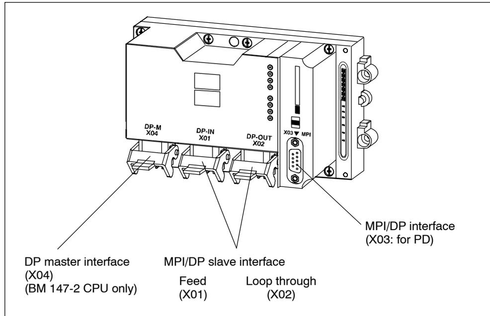
Figure 5-2 Interfaces on basic module BM 147 CPU
