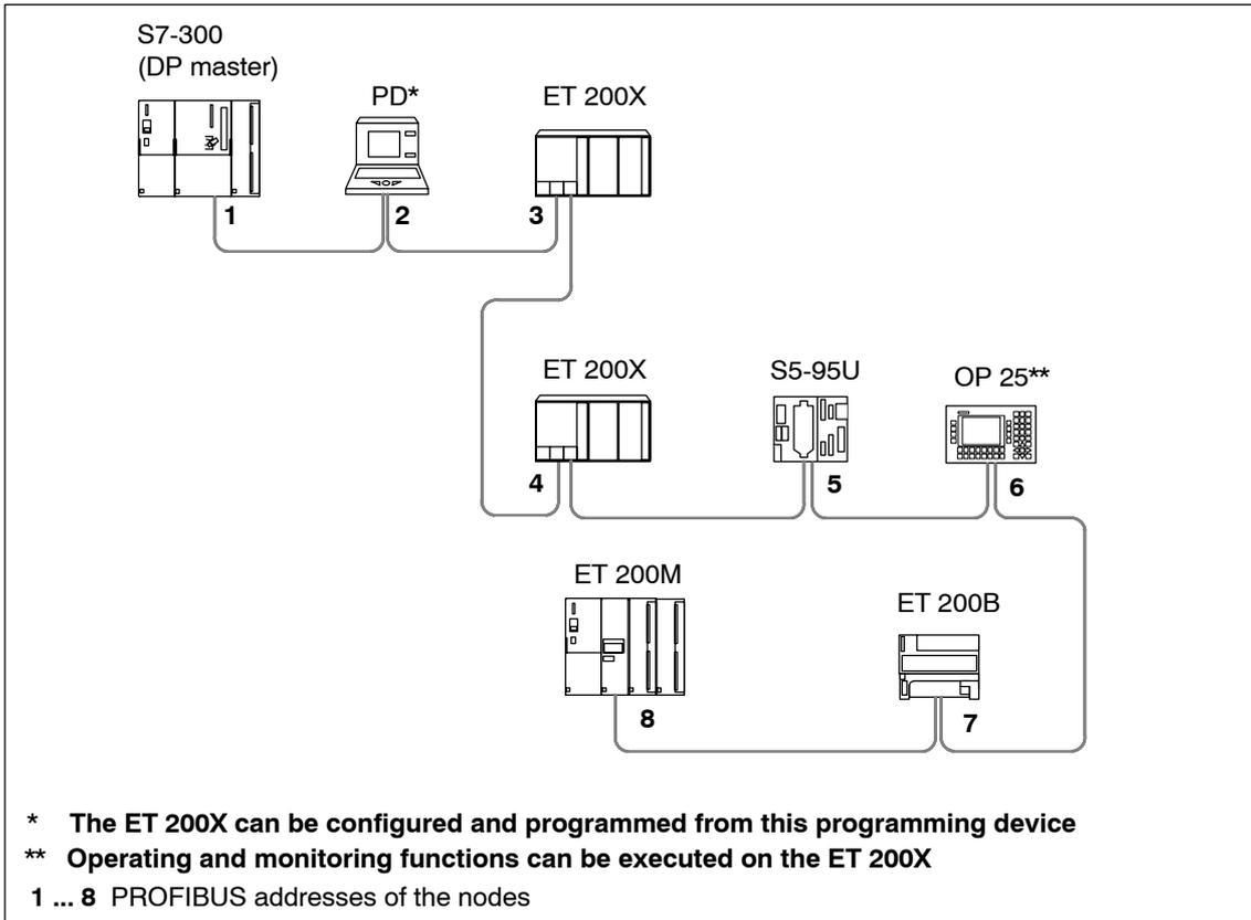
Figure 3-1 Example of a PROFIBUS network
