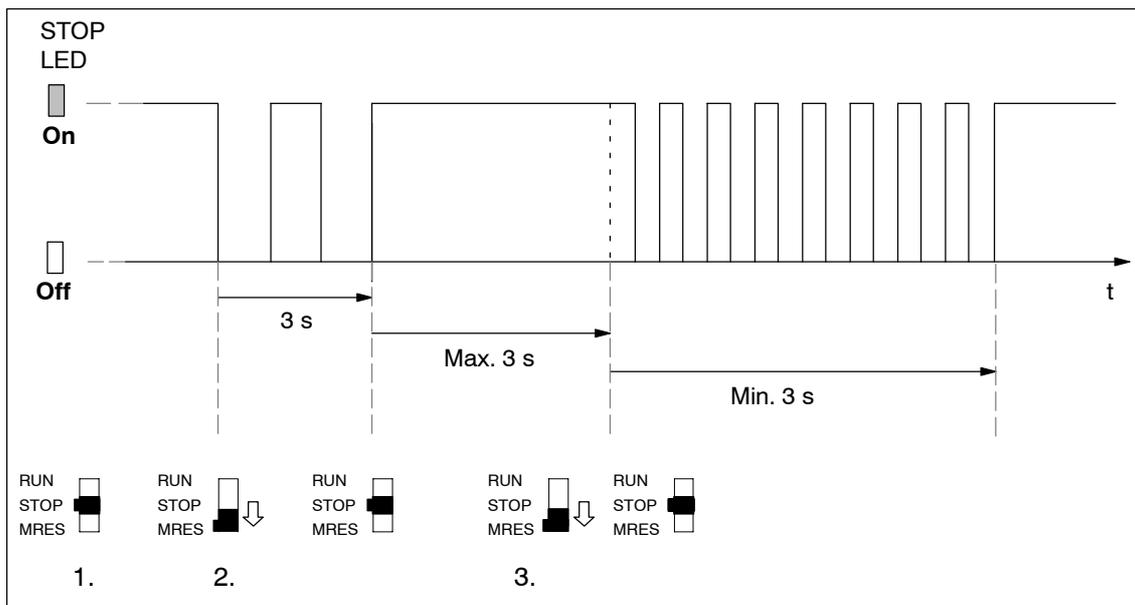
Figure 6-1 Operating sequence on the mode selector for performing a general reset
