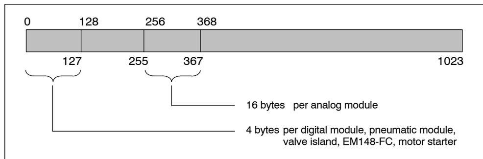
Figure 2-2 Structure of the default address area
