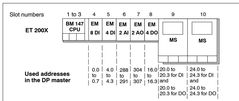
Figure 2-4 Example of address assignment to expansion modules
