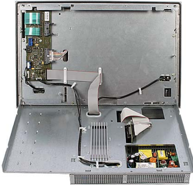
Figure 1-2 Example 12" touch screen device: Separating the computer unit from the control unit
