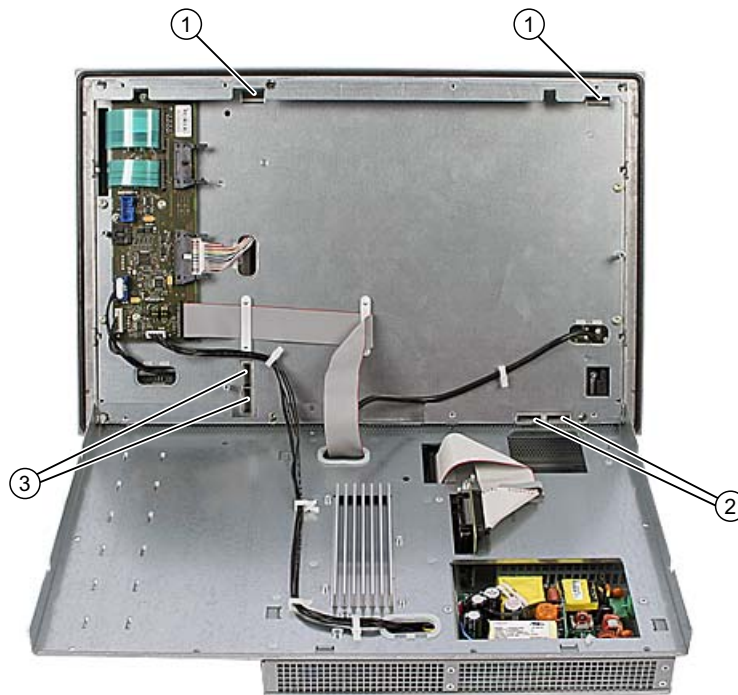
Figure 1-3 Device rear with connections and slots for the labeling strips
