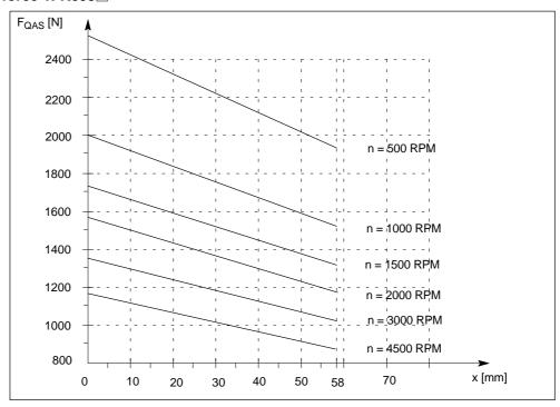
Fig. 2-15 Cantilever force  $F_Q$  at a distance x from the shaft shoulder for a nominal bearing lifetime of 20 000 h.
