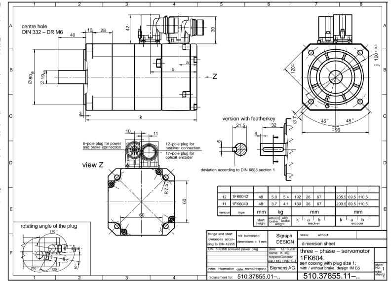
Fig. 4-2 1FK604□ standard, non-ventilated with angled connector, Size 1
