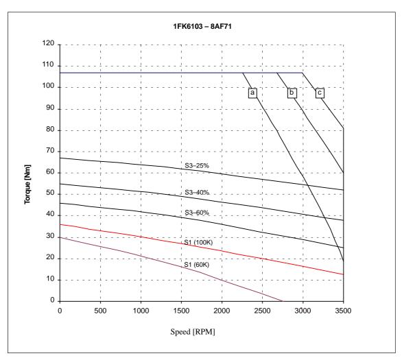
Speed-torque diagram 1FK6103 Standard Fig. 2-10
