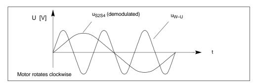
Fig. 3-3 Signal sequence and assignment for a positive direction of rotation (clockwise direction rotation when viewing the drive end)
