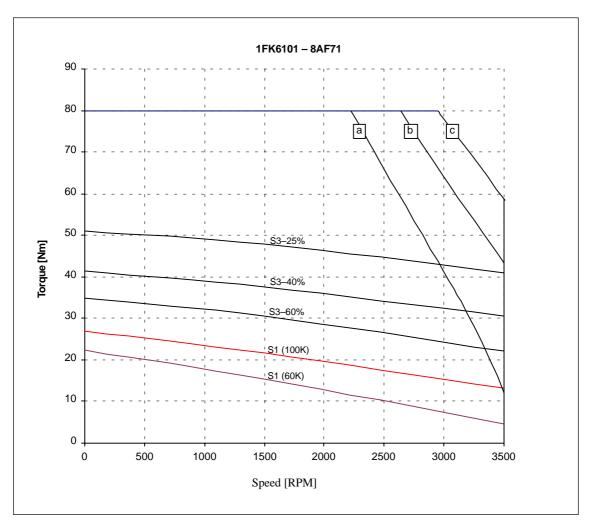
Speed-torque diagram 1FK6101 Standard Fig. 2-9
