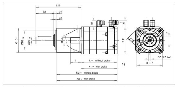
Fig. 3-4 Dimensions, standard 1FK6 motor, shaft height 36 to shaft height 80, with planetary gearbox
