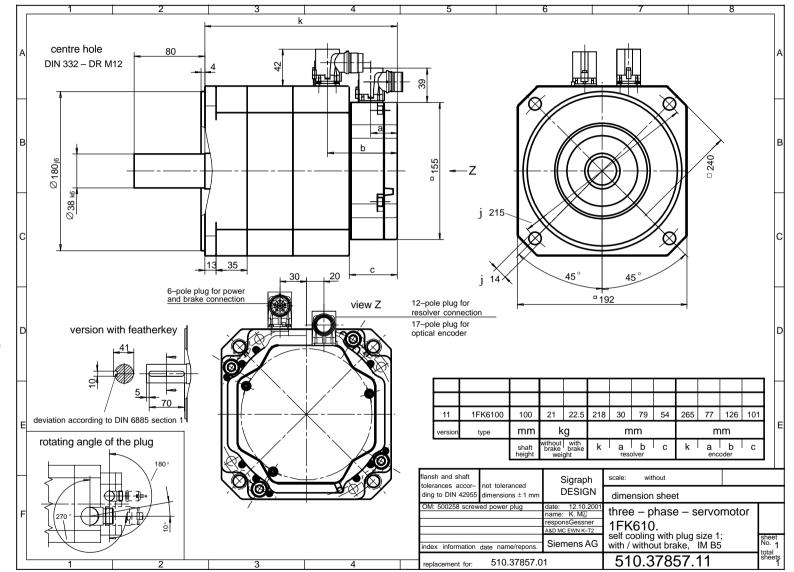
Fig. 4-5 1FK610□ standard, non-ventilated with connector, Size 1
