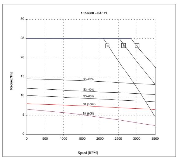
Fig. 2-6 Speed-torque diagram 1FK6080 Standard
