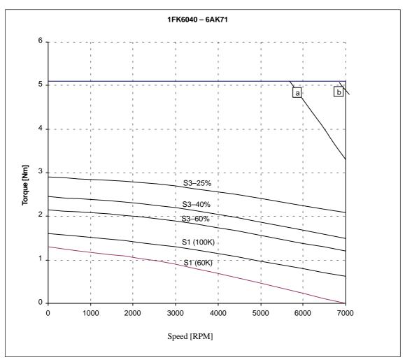
Fig. 2-2 Speed-torque diagram 1FK6040 Standard
