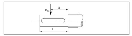
Fig. 2-11 Force application point at the DE shaft end
