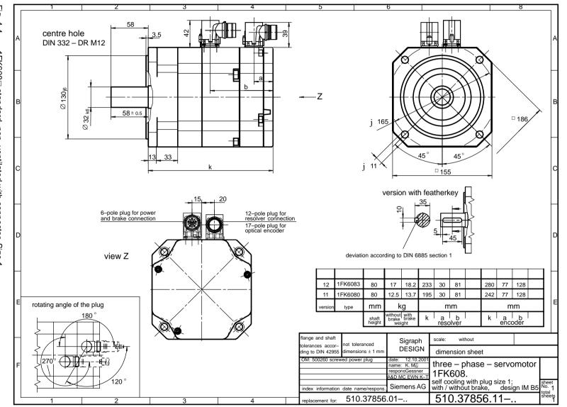
Fig. 4-4 1FK608□ standard, non-ventilated with connector, Size
