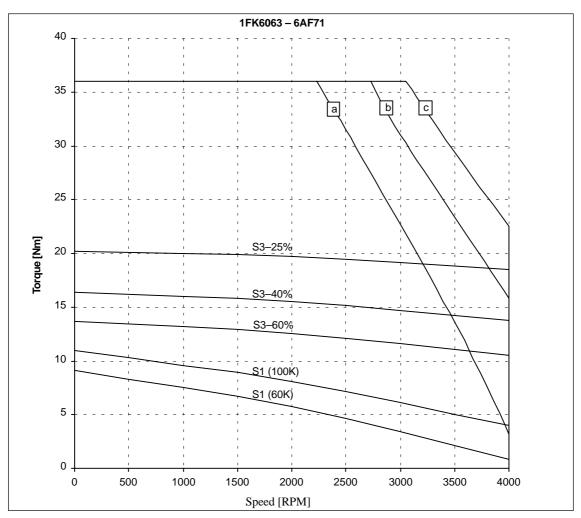
Fig. 2-5 Speed-torque diagram 1FK6063 Standard
