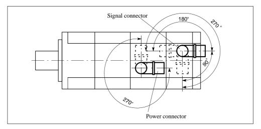
Fig. 1-2 Connectors can be rotated
