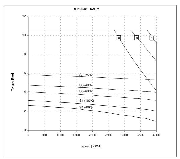
Speed-torque diagram 1FK6042 Standard Fig. 2-3
