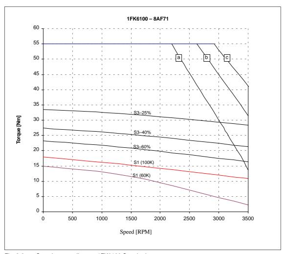
Fig. 2-8 Speed-torque diagram 1FK6100 Standard
