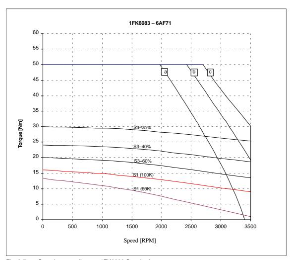
Fig. 2-7 Speed-torque diagram 1FK6083 Standard
