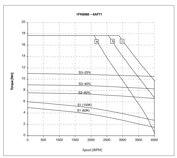
Fig. 2-4 Speed-torque diagram 1FK6060 Standard
