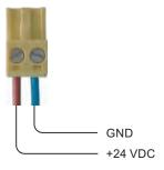
Do not confuse the lines. Refer to the label for the contact pins on the rear of the HMI device.
