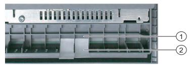
6. Slide the labeling strips into the guide up to the stop.
