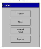
The HMI device automatically switches to "Transfer" mode during initial startup under the following conditions:
