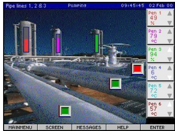
Examples of Screen Designs on a Minitrend V5.
