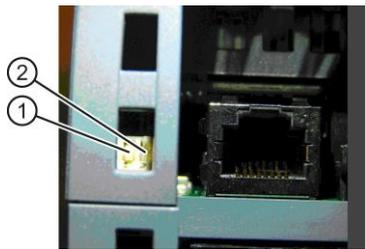
Figure 8-4 DIP switches at SIWAREX WP241 weighing module
