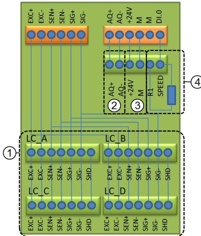
Figure 6-8 Terminal board SIWAREX WT241
