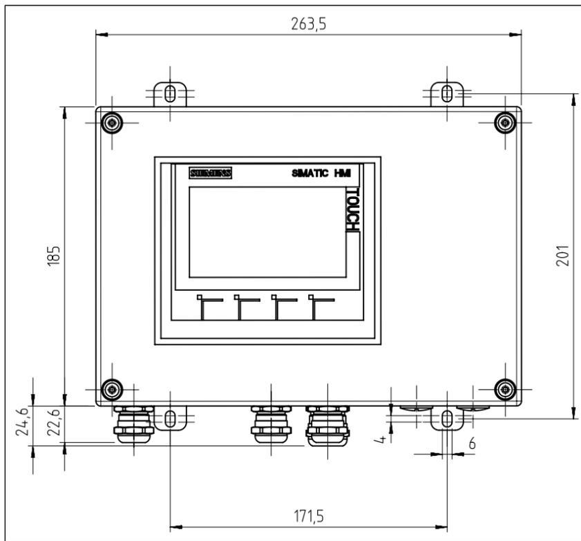
Figure 5-1 SIWAREX WT241 weighing terminal – dimensions and hole pattern
