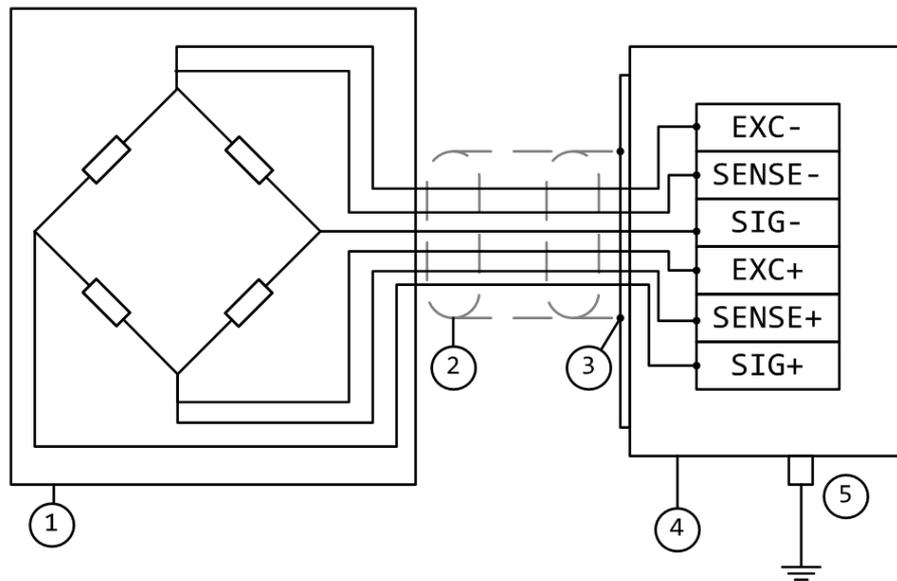
Figure 6-9 Connection of strain gauge load cell(s) with 6-wire system
