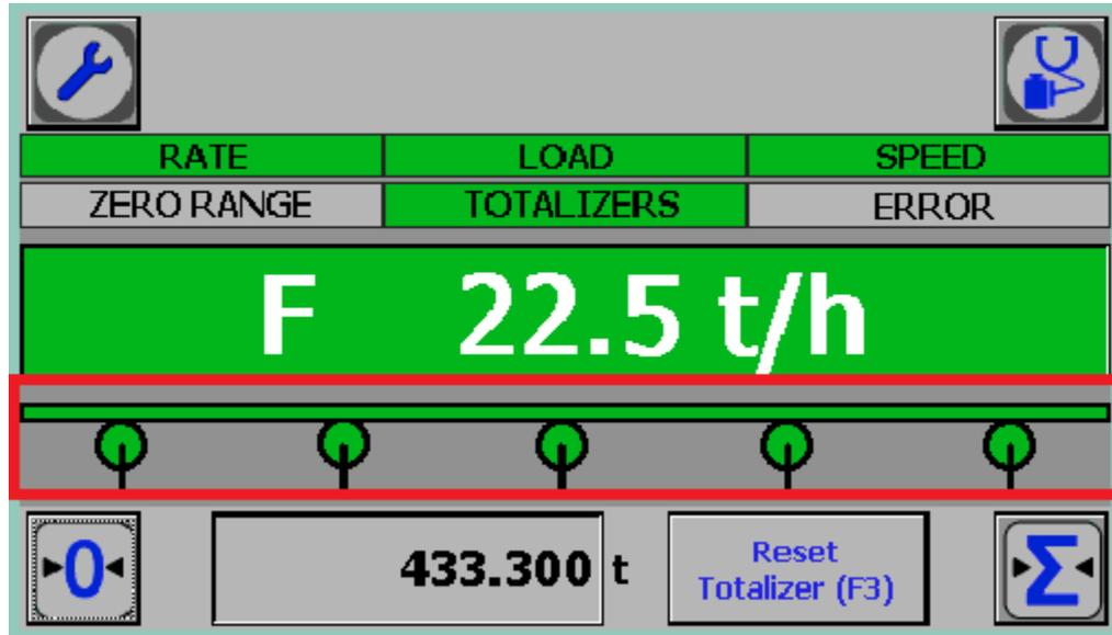
Figure 8-3 SIWAREX WT241 operating view – press the belt scale to jump to menu 2.2.1
