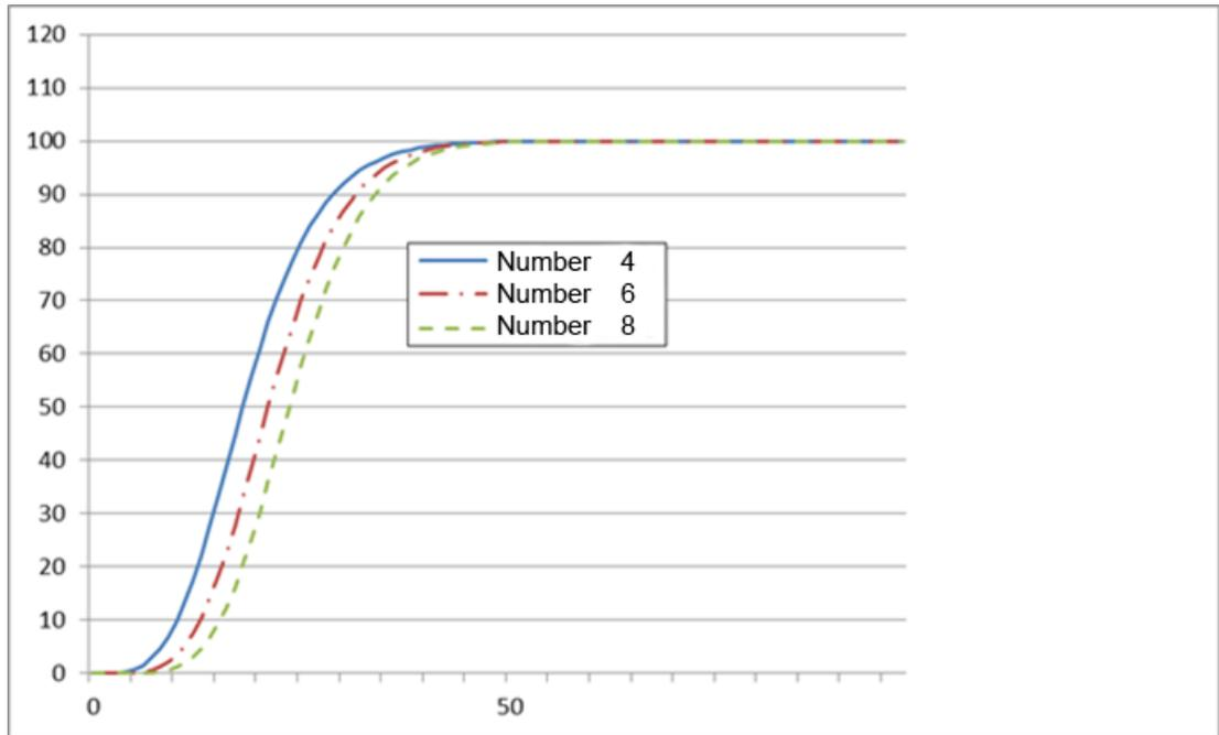
Figure 11-1 Step response of the digital low-pass filter when  $f_g = 2$  Hz
