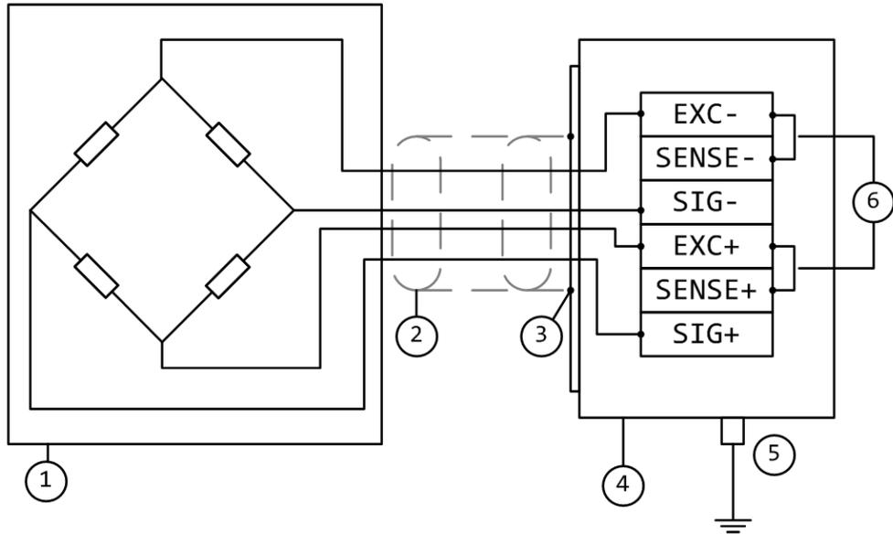
Figure 6-10 Connection of strain gauge load cell(s) with 4-wire system
