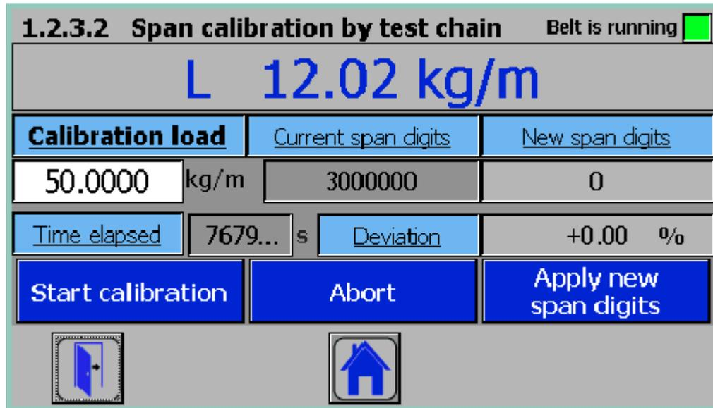
Figure 7-12 Span calibration by test chain
