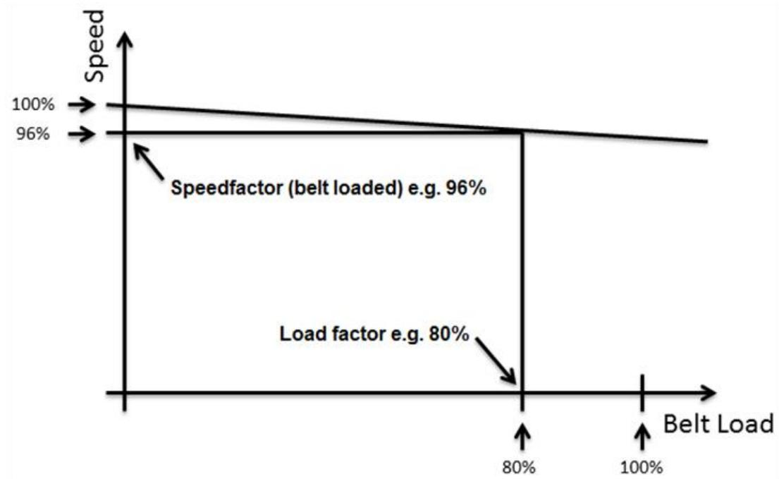
Figure 7-8 Speed characteristic without sensor
