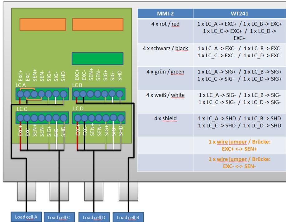
Figure 6-7 Connecting a Siemens belt scale MMI-2 to SIWAREX WT241
