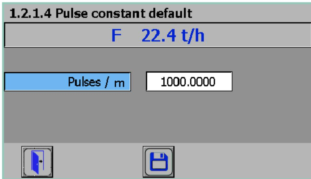
Figure 7-4 Specification of pulse constant
