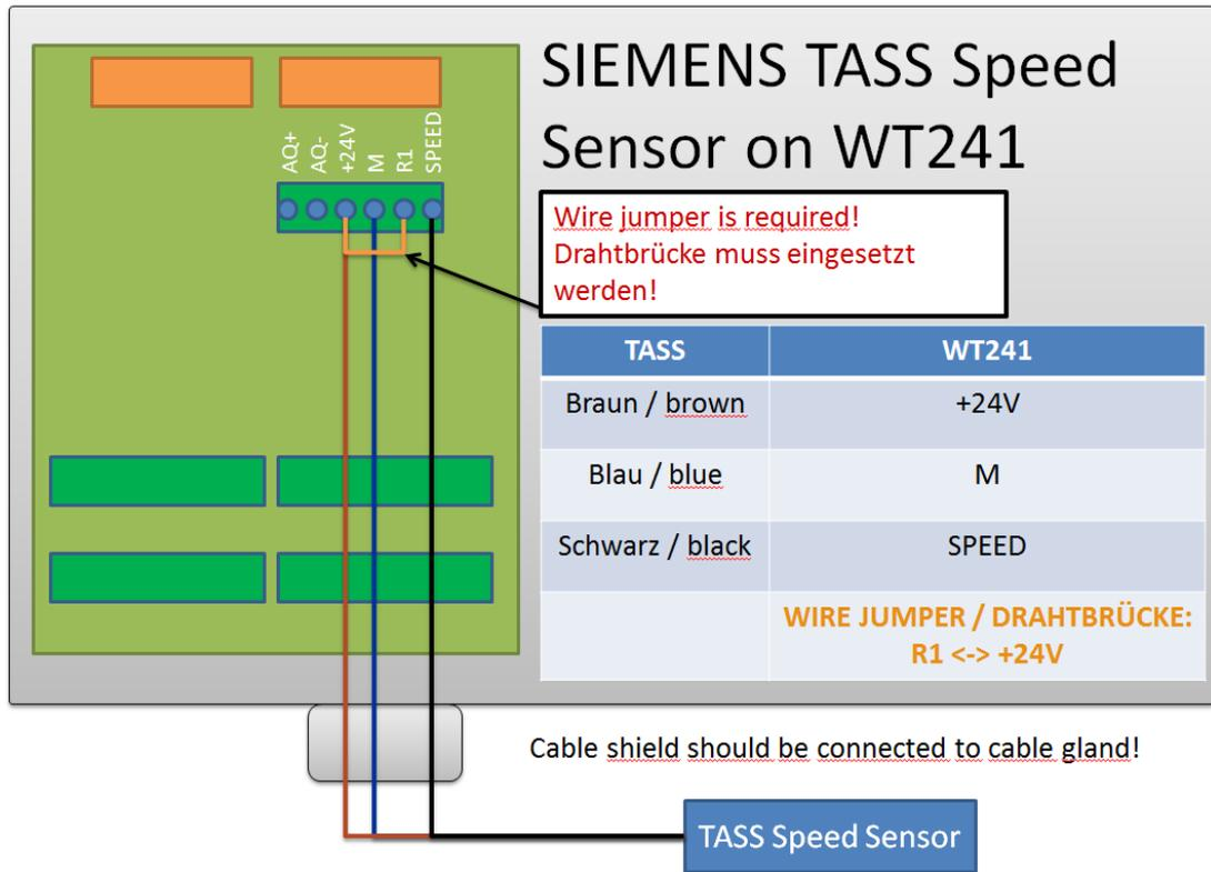
Figure 6-12 TASS speed sensor on WT241
