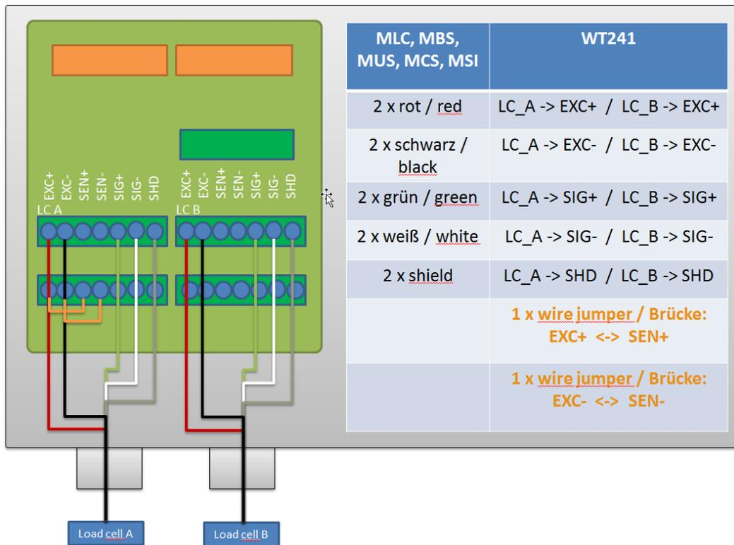
Figure 6-6 Connecting Siemens beltscales MLC, MBS, MUS, MCS, MSU to SIWAREX WT241
