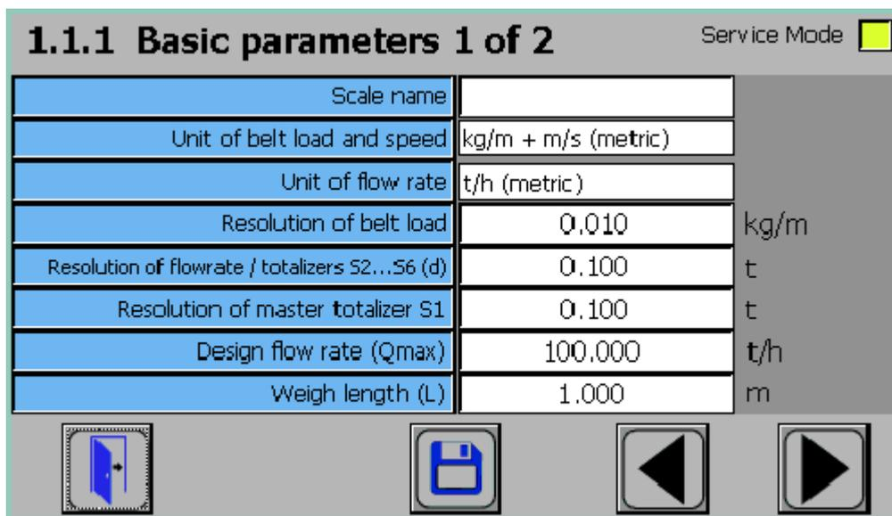
Figure 7-2 Basic parameters 1 of 2
