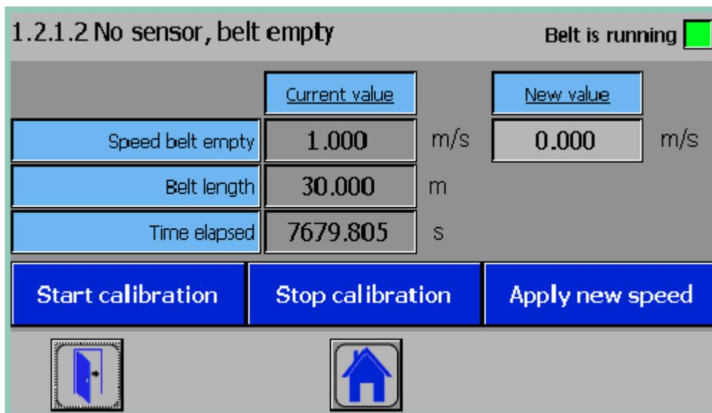
Figure 7-7 Speed calculation with empty belt
