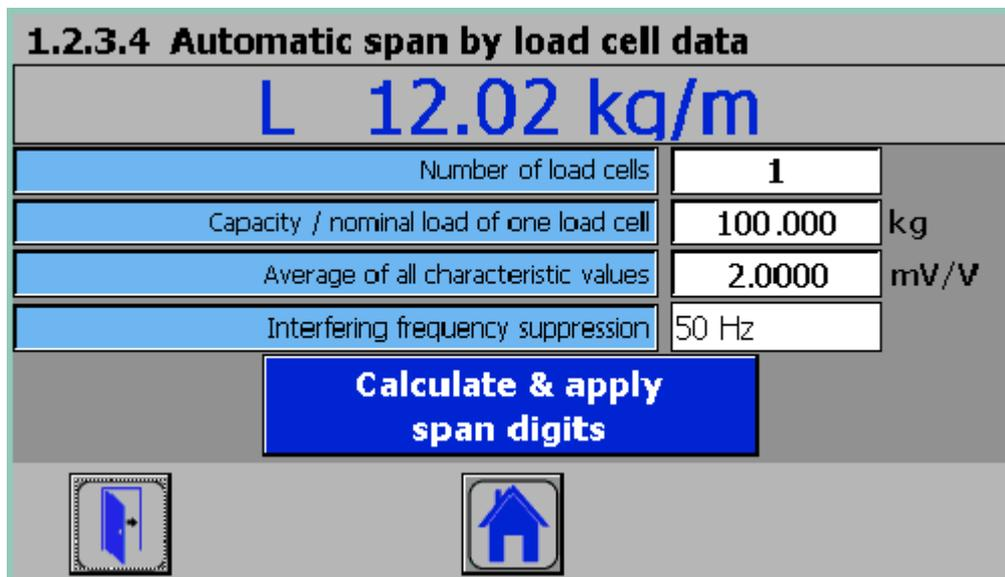
Figure 7-14 Automatic span calibration
