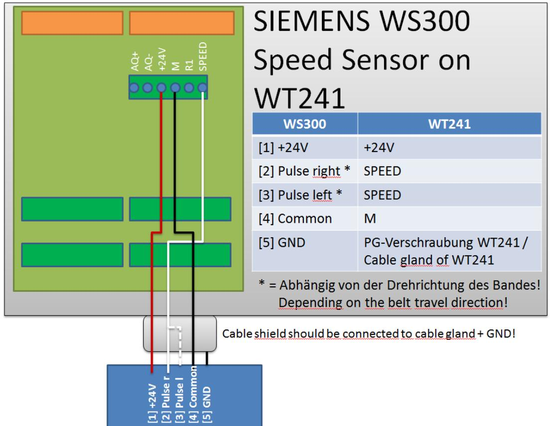
Figure 6-13 WS300 speed sensor on WT241
