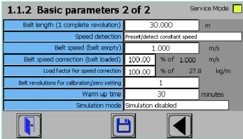
Figure 7-6 Specification of a known, constant belt speed
