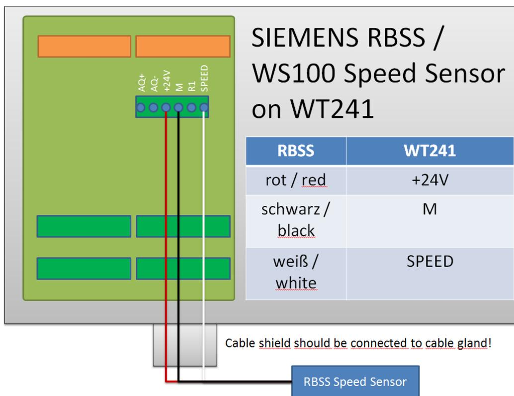
Figure 6-11 RBSS speed sensor on WT241
