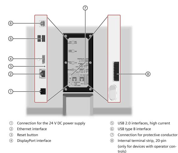
The following figure shows the position of the interfaces.
