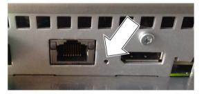
3. Switch on the device's power supply and keep the reset button pressed for an additional 10 seconds.
