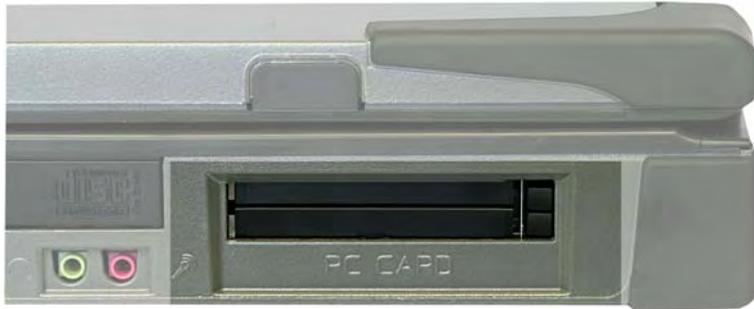
The PC Card ejectors have a spring-coil mechanism. ### Before you insert the card, ensure that the ejector is engaged. To remove the PC Card, press the ejector once to unlock it and a second time to eject the PC Card.
