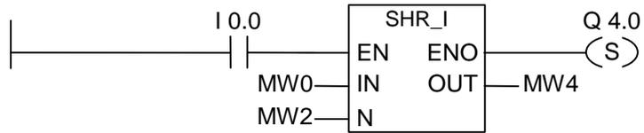
The SHR\_I box is activated by logic "1" at I0.0. MW0 is loaded and shifted right by the number of bits specified with MW2. The result is written to MW4. Q4.0 is set.
