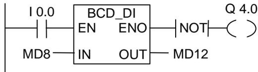
If I0.0 is "1", then the content of MD8 is read as a seven-digit BCD coded number and converted to a double integer. The result is stored in MD12. The output Q4.0 is "1" if the conversion is not executed (ENO = EN = 0).
