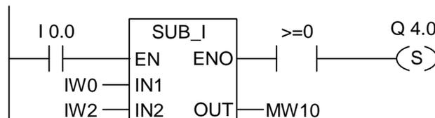
The box is activated by signal state "1" at I0.0. If the value of IW0 is higher or equal to the value of IW2, the result of the math function "IW0 - IW2" is greater than or equal to "0". Q4.0 is set if the function is properly executed and the result is **greater** than or equal to "0".
