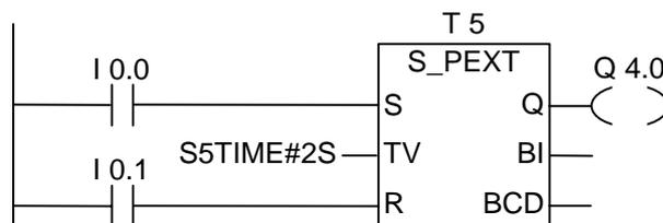
If the signal state of input I0.0 changes from "0" to "1" (positive edge in RLO), the timer T5 will be started. The timer will continue to run for the specified time of two seconds (2 s) without being affected by a negative edge at input S. If the signal state of I0.0 changes from "0" to "1" before the timer has expired the timer will be re-triggered. The output Q4.0 is logic "1" as long as the timer is running.
