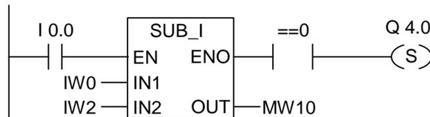
The box is activated by signal state "1" at I0.0. If the value of IW0 is equal to the value of IW2, the result of the math function "IW0 - IW2" is "0". Q4.0 is set if the function is properly executed and the result is **equal** to "0".
