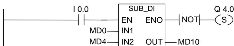
The SUB\_DI box is activated if I0.0 = "1". The result of the subtraction MD0 - MD4 is output to MD10. If the result was outside the permissible range for a double integer, the output Q4.0 is set.
