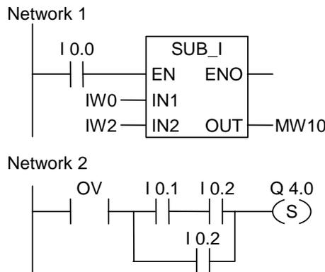
The box is activated by signal state "1" at I0.0. If the result of the math function "IW0 - IW2" is outside the permissible range for an integer, the OV bit is set.
