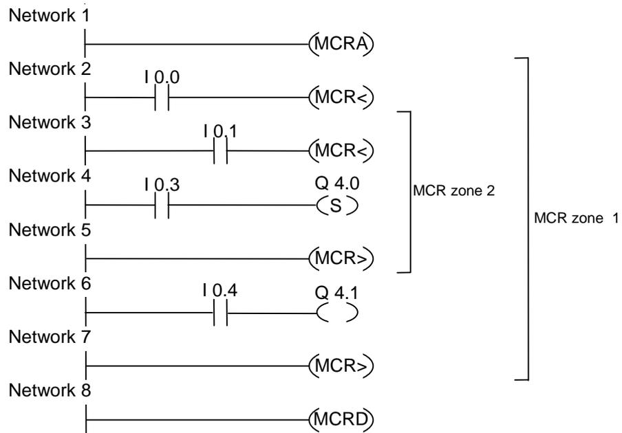
MCR functionality is activated by the ---(MCRA) rung. It is then possible to create up to eight nested MCR zones. In the example there are two MCR zones. The first ---(MCR>) (MCR OFF) rung belongs to the second ---(MCR<) (MCR ON) rung. All rungs between belong to the MCR zone 2. The functions are executed as follows:
