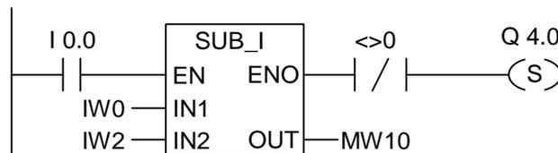
Q4.0 is set if the function is properly executed and the result is **equal** to "0".
