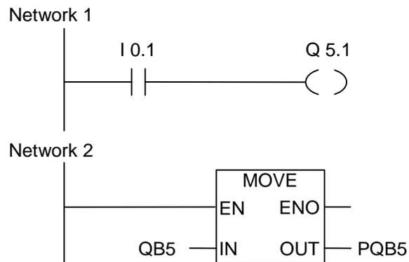
In this example Q5.1 is the desired immediate output bit.
