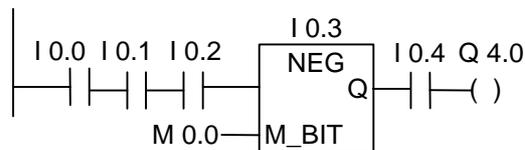
The signal state at output Q4.0 is "1" if the following conditions exist:
