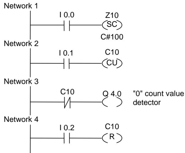
If the signal state of input I0.0 changes from "0" to "1" (positive edge in RLO), the preset value of 100 is loaded to counter C10.
