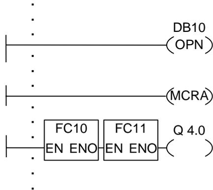
The Ladder rungs shown above are program sections from a function block written by a user. In this FB, DB10 is opened and MCR functionality is activated. If the unconditional call of FC10 is executed, the following occurs:
