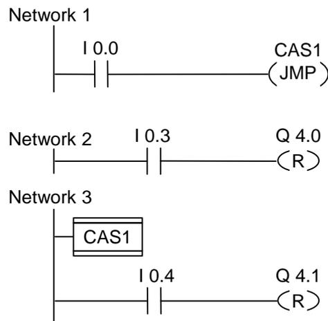
If I0.0 = "0", the jump to label CAS1 is executed. Because of the jump, the instruction to reset output Q4.0 is not executed even if there is a logic "1" at I0.3.
