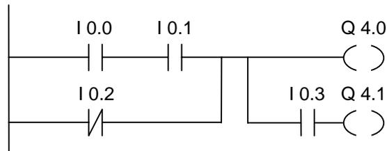
The signal state of output Q4.0 is "1" if one of the following conditions exists:
