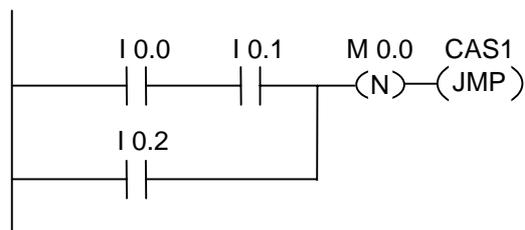
The edge memory bit M0.0 saves the old RLO state. When there is a signal change at the RLO from "1" to "0", the program jumps to label CAS1.
