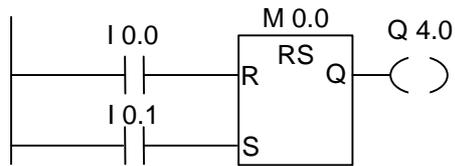
If the signal state is "1" at input I0.0 and "0" at I0.1, memory bit M0.0 is set and output Q4.0 is "0". Otherwise, if the signal state at input I0.0 is "0" and at I0.1 is "1", memory bit M0.0 is reset and output Q4.0 is "1". If both signal states are "0", nothing is changed. If both signal states are "1", the set instruction dominates because of the order; M0.0 is set and Q4.0 is "1".
