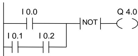
The signal state of output Q4.0 is "0" if one of the following conditions exists:
