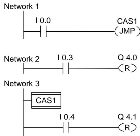
If I0.0 = "1", the jump to label CAS1 is executed. Because of the jump, the instruction to reset output Q4.0 is not executed even if there is a logic "1" at I0.3.
