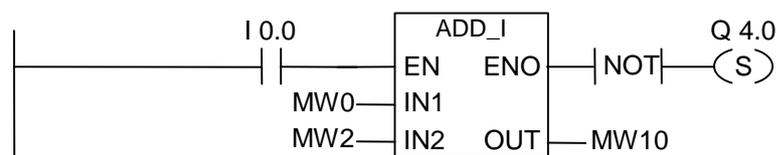
The ADD\_I box is activated if I0.0 = "1". The result of the addition MW0 + MW2 is output to MW10. If the result was outside the permissible range for an integer, the output Q4.0 is set.
