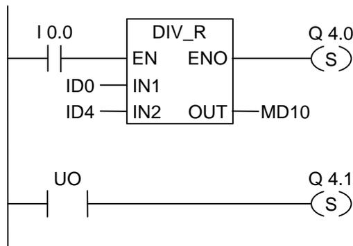
The box is activated by signal state "1" at I0.0. If the value of ID0 or ID4 is an invalid floating-point number, the math function is invalid. If the signal state of EN = 1 (activated) and if an error occurs during the processing of the function DIV\_R, the signal state of ENO = 0.
