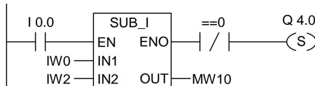
Q4.0 is set if the function is properly executed and the result is **not equal** to "0".
