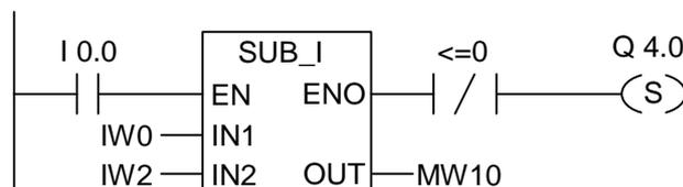
Q4.0 is set if the function is properly executed and the result is **not less** than or equal to "0".
