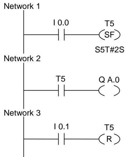
If the signal state of input I0.0 changes from "1" to "0" the timer is started.
