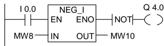
If I0.0 is "1", then the value of MW8 with the opposite sign is output by the OUT parameter to MW10.
