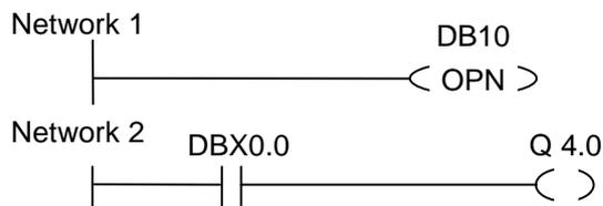
Data block 10 (DB10) is opened. The contact address (DBX0.0) refers to bit zero of data byte zero of the current data record contained in DB10. The signal state of this bit is assigned to the output Q4.0.
