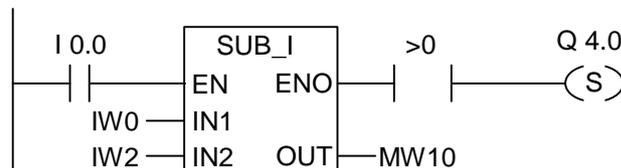
The box is activated by signal state "1" at I0.0. If the value of IW0 is higher than the value of IW2, the result of the math function "IW0 - IW2" is greater than "0". Q4.0 is set if the function is properly executed and the result is **greater** than "0".
