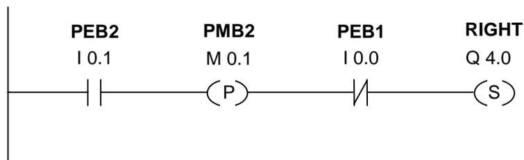
Network 3: If neither photoelectric barrier is broken, then there is no package between the barriers. The direction pointer shuts off.
