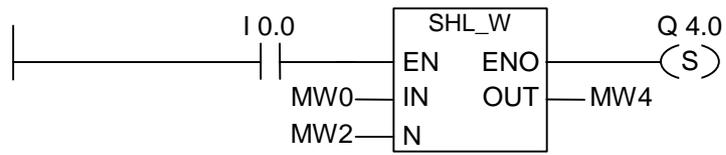
The SHL\_W box is activated by logic "1" at I0.0. MW0 is loaded and shifted left by the number of bits specified with MW2. The result is written to MW4. Q4.0 is set.
