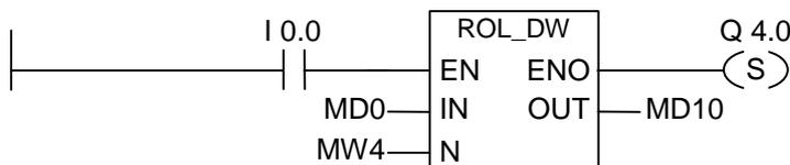
The ROL\_DW box is activated by logic "1" at I0.0. MD0 is loaded and rotated to the left by the number of bits specified with MW4. The result is written to MD10. Q4.0 is set.
