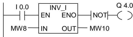
If I0.0 is "1", then every bit of MW8 is reversed, for example:
