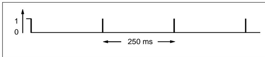
As soon as the time runs out, the timer is restarted. Because of this, the signal check made by —| / |— M0.2 produces a signal state of 1 only briefly.
