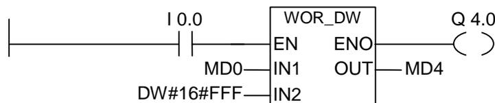
The instruction is executed if I0.0 is "1". Bits 0 to 11 are set to "1", the remaining MD0 bits are not changed:
