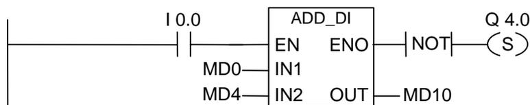
The ADD\_DI box is activated if I0.0 = "1". The result of the addition MD0 + MD4 is output to MD10. If the result was outside the permissible range for a double integer, the output Q4.0 is set.
