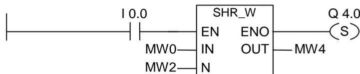
The SHR\_W box is activated by logic "1" at I0.0. MW0 is loaded and shifted right by the number of bits specified with MW2. The result is written to MW4. Q4.0 is set.
