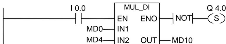
The MUL\_DI box is activated if I0.0 = "1". The result of the multiplication MD0 x MD4 is output to MD10. If the result was outside the permissible range for a double integer, the output Q4.0 is set.
