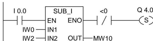
Q4.0 is set if the function is properly executed and the result is **not** less than "0".
