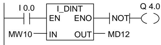
If I0.0 is "1", then the content of MW10 is read as an integer and converted to a double integer. The result is stored in MD12. The output Q4.0 is "1" if the conversion is not executed (ENO = EN = 0).
