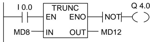
If I0.0 is "1", then the content of MD8 is read as a real number and converted to a double integer. The integer part of the floating-point number is the result and is stored in MD12. The output Q4.0 is "1" if an overflow occurred, or the instruction was not executed (I0.0 = 0).
