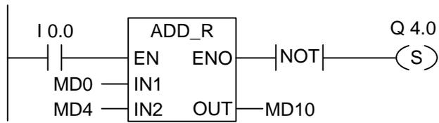
The ADD\_R box is activated by logic "1" at I0.0. The result of the addition MD0 + MD4 is output to MD10. If the result was outside the permissible range for a floating-point number or if the program statement was not processed (I0.0 = 0), the output Q4.0 is set.
