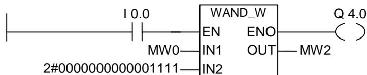
The instruction is executed if I0.0 is "1". Only bits 0 to 3 of MW0 are relevant, the rest of MW0 is masked by the IN2 word bit pattern:
