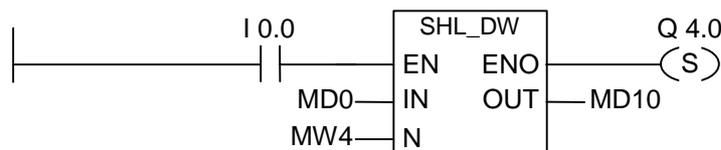
The SHL\_DW box is activated by logic "1" at I0.0. MD0 is loaded and shifted left by the number of bits specified with MW4. The result is written to MD10. Q4.0 is set.
