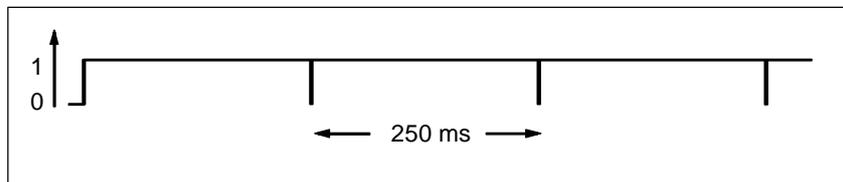
Every 250 ms the RLO bit is 0. The jump is ignored and the contents of memory word MW100 is incremented by 1.
