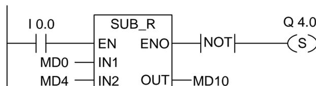
The SUB\_R box is activated by logic "1" at I0.0. The result of the subtraction MD0 - MD4 is output to MD10. If the result was outside the permissible range for a floating-point number or if the program statement was not processed, the output Q4.0 is set.
