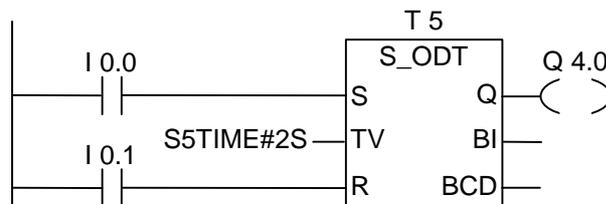
If the signal state of I0.0 changes from "0" to "1" (positive edge in RLO), the timer T5 will be started. If the time of two seconds elapses and the signal state at input I0.0 is still "1", the output Q4.0 will be "1". If the signal state of I0.0 changes from "1" to "0", the timer is stopped and Q4.0 will be "0" (if the signal state of I0.1 changes from "0" to "1", the time is reset regardless of whether the timer is running or not).
