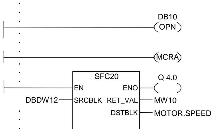
The Ladder rungs shown above are program sections from a function block written by a user. In this FB, DB10 is opened and MCR functionality is activated. If the unconditional call of SFC20 is executed, the following occurs:
