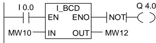
If I0.0 is "1", then the content of MW10 is read as an integer and converted to a three-digit BCD coded number. The result is stored in MW12. The output Q4.0 is "1" if there was an overflow, or the instruction was not executed (I0.0 = 0).
