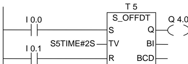
If the signal state of I0.0 changes from "1" to "0", the timer is started.
