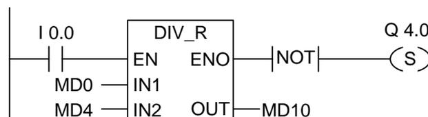
The DIV\_R box is activated by logic "1" at I0.0. The result of the division MD0 by MD4 is output to MD10. If the result was outside the permissible range for a floating-point number or if the program statement was not processed, the output Q4.0 is set.
