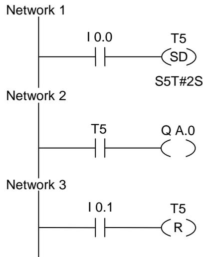
If the signal state of input I0.0 changes from "0" to "1" (positive edge in RLO), the timer T5 is started. If the time elapses and the signal state of input I0.0 is still "1", the signal state of output Q4.0 will be "1".
