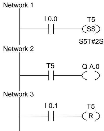
If the signal state of input I0.0 changes from "0" to "1" (positive edge in RLO), the timer T5 is started. If the signal state of input I0.0 changes from "0" to "1" before the timer has expired, the timer is re-triggered. The output Q4.0 will be "1" if the timer elapsed. A signal state "1" at input I0.1 will reset timer T5, which stops the timer and clears the remaining portion of the time value to "0".
