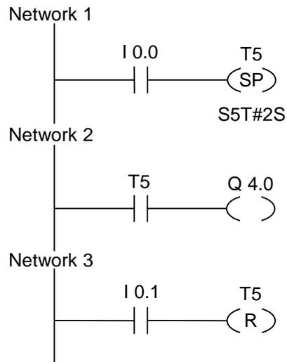
If the signal state of input I0.0 changes from "0" to "1" (positive edge in RLO), the timer T5 is started. The timer continues to run with the specified time of two seconds as long as the signal state of input I0.0 is "1". If the signal state of input I0.0 changes from "1" to "0" before the specified time has elapsed, the timer stops.
