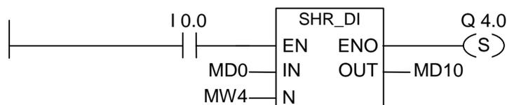
The SHR\_DI box is activated by logic "1" at I0.0. MD0 is loaded and shifted right by the number of bits specified with MW4. The result is written to MD10. Q4.0 is set.
