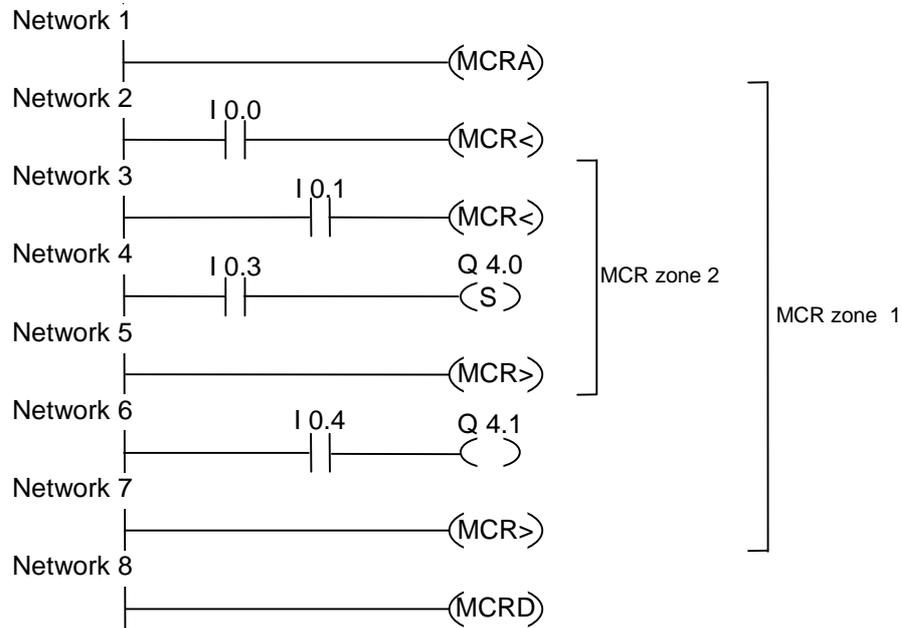
MCR functionality is activated by the MCRA rung. It is then possible to create up to eight nested MCR zones. In the example there are two MCR zones. The functions are executed as follows:
