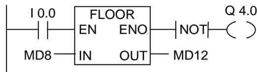
If I0.0 is "1", then the content of MD8 is read as a floating-point number and converted to a double integer by the round to - infinity mode. The result is stored in MD12. The output Q4.0 is "1" if an overflow occurred, or the instruction was not executed (I0.0 = 0).
