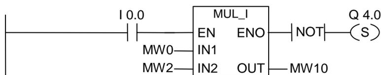
The MUL\_I box is activated if I0.0 = "1". The result of the multiplication MW0 x MW2 is output to MD10. If the result was outside the permissible range for an integer, the output Q4.0 is set.
