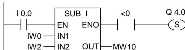
The box is activated by signal state "1" at I0.0. If the value of IW0 is lower than the value of IW2, the result of the math function "IW0 - IW2" is less than "0". Q4.0 is set if the function is properly executed and the result is **less** than "0".
