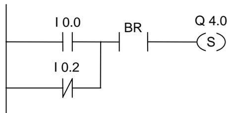
Q4.0 is set if I0.0 is "1" or I0.2 is "0" and in addition to this RLO the logic state of the BR bit is "1".
