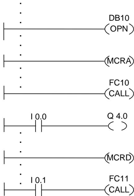
The Ladder rungs shown above are program sections from a function block written by a user. In this FB, DB10 is opened and MCR functionality is activated. If the unconditional call of FC10 is executed, the following occurs:
