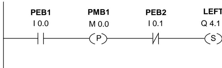
Network 2: If there is a transition in signal state from 0 to 1 (positive edge) at input I 0.1 and, at the same time, the signal state at input I 0.0 is 0, then the package on the belt is moving to the right. If one of the photoelectric light barriers is broken, this means that there is a package between the barriers.
