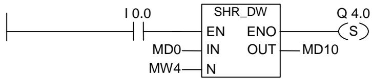
The SHR\_DW box is activated by logic "1" at I0.0. MD0 is loaded and shifted right by the number of bits specified with MW4. The result is written to MD10. Q4.0 is set.
