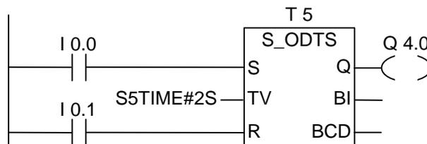
If the signal state of I0.0 changes from "0" to "1" (positive edge in RLO), the timer T5 will be started. The timer runs without regard to a signal change at I0.0 from "1" to "0". If the signal state at I0.0 changes from "0" to "1" before the timer has expired, the timer will be re-triggered. The output Q4.0 will be "1" if the timer elapsed. (If the signal state of input I0.1 changes from "0" to "1", the time will be reset irrespective of the RLO at S.)
