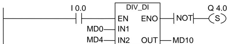
The DIV\_DI box is activated if I0.0 = "1". The result of the division MD0 : MD4 is output to MD10. If the result was outside the permissible range for a double integer, the output Q4.0 is set.
