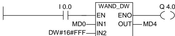
The instruction is executed if I0.0 is "1". Only bits 0 and 11 of MD0 are relevant, the rest of MD0 is masked by the IN2 bit pattern:
