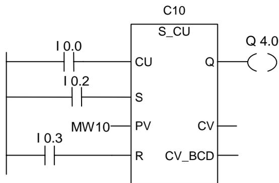
If I0.2 changes from "0" to "1", the counter is preset with the value of MW10. If the signal state of I0.0 changes from "0" to "1", the value of counter C10 will be incremented by one - unless the value of C10 is equal to "999". Q4.0 is "1" if C10 is not equal to zero.
