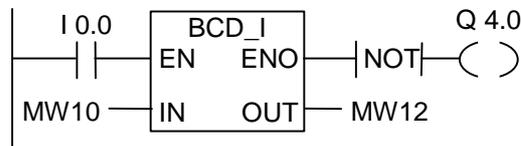
If input I0.0 is "1", then the content of MW10 is read as a three-digit BCD coded number and converted to an integer. The result is stored in MW12. The output Q4.0 is "1" if the conversion is not executed (ENO = EN = 0).
