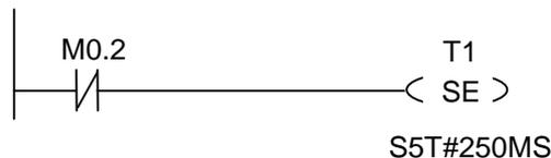
Network 2: The state of the timer is saved temporarily in an auxiliary memory marker.
