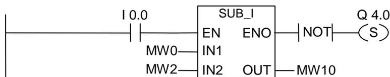
The SUB\_I box is activated if I0.0 = "1". The result of the subtraction MW0 - MW2 is output to MW10. If the result was outside the permissible range for an integer or the signal state of I0.0 = 0, the output Q4.0 is set.
