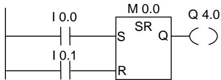
If the signal state is "1" at input I0.0 and "0" at I0.1, memory bit M0.0 is set and output Q4.0 is "1". Otherwise, if the signal state at input I0.0 is "0" and at I0.1 is "1", memory bit M0.0 is reset and output Q4.0 is "0". If both signal states are "0", nothing is changed. If both signal states are "1", the reset instruction dominates because of the order; M0.0 is reset and Q4.0 is "0".
