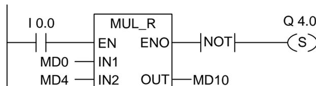
The **MUL\_R** box is activated by logic "1" at I0.0. The result of the multiplication MD0 x MD4 is output to MD0. If the result was outside the permissible range for a floating-point number or if the program statement was not processed, the output Q4.0 is set.
