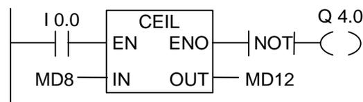
If I0.0 is 1, the contents of MD8 are read as a floating-point number which is converted into a double integer using the function **Round**. The result is stored in MD12. The output Q4.0 is "1" if an overflow occurred or the instruction was not processed (I0.0 = 0).
