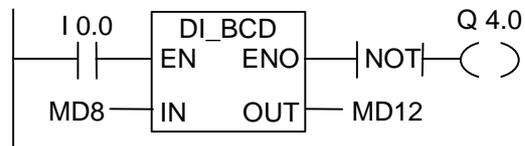
If I0.0 is "1", then the content of MD8 is read as a double integer and converted to a seven-digit BCD number. The result is stored in MD12. The output Q4.0 is "1" if an overflow occurred, or the instruction was not executed (I0.0 = 0).
