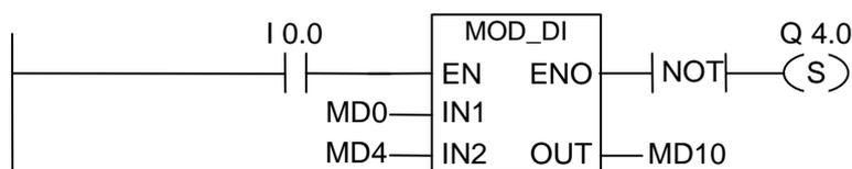
The DIV\_DI box is activated if I0.0 = "1". The remainder of the division MD0:MD4 is output to MD10. If the remainder was outside the permissible range for a double integer, the output Q4.0 is set.
