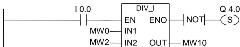
The DIV\_I box is activated if I0.0 = "1". The result of the division MW0 by MW2 is output to MW10. If the result was outside the permissible range for an integer, the output Q4.0 is set.
