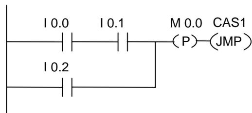
The edge memory bit M0.0 saves the old RLO state. When there is a signal change at the RLO from "0" to "1", the program jumps to label CAS1.
