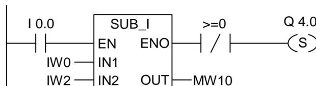
Q4.0 is set if the function is properly executed and the result is **not** greater than or equal to "0".
