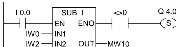
The box is activated by signal state "1" at I0.0. If the value of IW0 is different to the value of IW2, the result of the math function "IW0 - IW2" is not equal to "0". Q4.0 is set if the function is properly executed and the result is **not equal** to "0".
