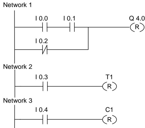
The signal state of output Q4.0 is reset to "0" if one of the following conditions exists:
