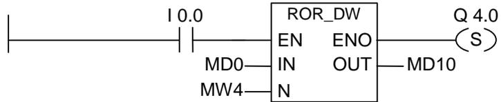
The ROR\_DW box is activated by logic "1" at I0.0. MD0 is loaded and rotated to the right by the number of bits specified with MW4. The result is written to MD10. Q4.0 is set.
