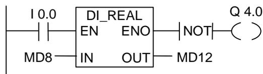
If I0.0 is "1", then the content of MD8 is read as a double integer and converted to a floating-point number. The result is stored in MD12. The output Q4.0 is "1" if the conversion is not executed (ENO = EN = 0).
