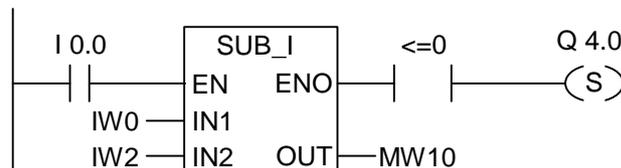
The box is activated by signal state "1" at I0.0. If the value of IW0 is less than or equal to the value of IW2 the result of the math function "IW0 - IW2" is less than or equal to "0". Q4.0 is set if the function is well properly executed and the result is **less** than or equal to "0".
