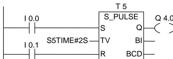
If the signal state of input I0.0 changes from "0" to "1" (positive edge in RLO), the timer T5 will be started. The timer will continue to run for the specified time of two seconds (2 s) as long as I0.0 is "1". If the signal state of I0.0 changes from "1" to "0" before the timer has expired the timer will be stopped. If the signal state of input I0.1 changes from "0" to "1" while the timer is running, the time is reset.
