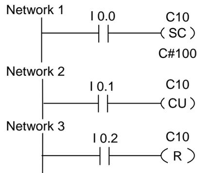
If the signal state of input I0.0 changes from "0" to "1" (positive edge in RLO), the preset value of 100 is loaded to counter C10.
