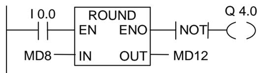
If I0.0 is "1", then the content of MD8 is read as a floating-point number and converted to the closest double integer. The result of this "Round to nearest" function is stored in MD12. The output Q4.0 is "1" if an overflow occurred or the instruction was not executed (I0.0 = 0).
