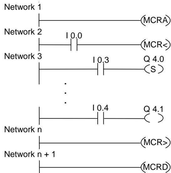
MCR functionality is activated by the MCRA rung. The rungs between the MCR< and the MCR> (outputs Q4.0, Q4.1) are executed as follows:
