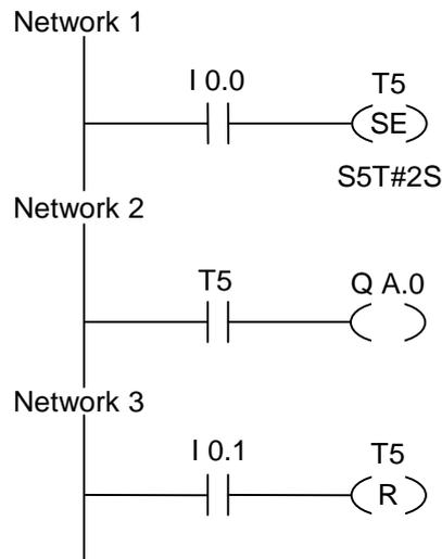
If the signal state of input I0.0 changes from "0" to "1" (positive edge in RLO), the timer T5 is started. The timer continues to run without regard to a negative edge of the RLO. If the signal state of I0.0 changes from "0" to "1" before the timer has expired, the timer is re-triggered.
