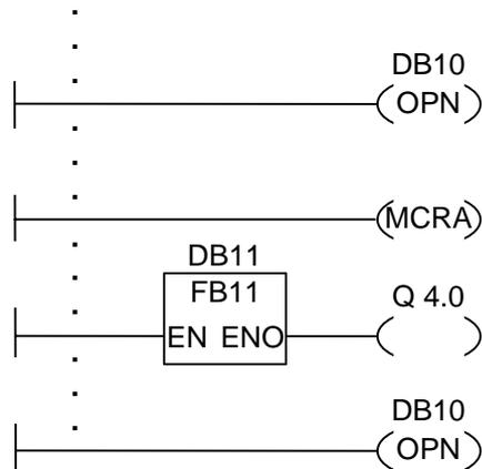
The Ladder rungs shown above are program sections from a function block written by a user. In this FB, DB10 is opened and MCR functionality is activated. If the unconditional call of FB11 is executed, the following occurs:
