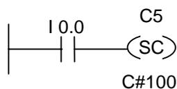
The counter C5 is preset with the value of 100 if there is a positive edge at input I0.0 (change from "0" to "1"). If there is no positive edge, the value of counter C5 remains unchanged.
