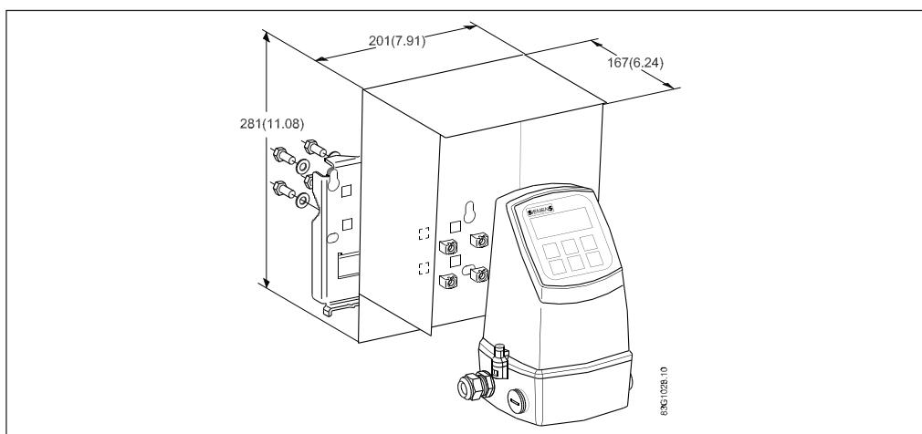
Refer to the adjacent figure and mount the sun shield as shown using the supplied screws and hardware.
