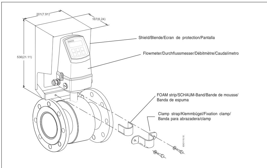
Refer to the adjacent figure and mount the sun shield as shown using the supplied foam strip, clamp strap, and hardware.
