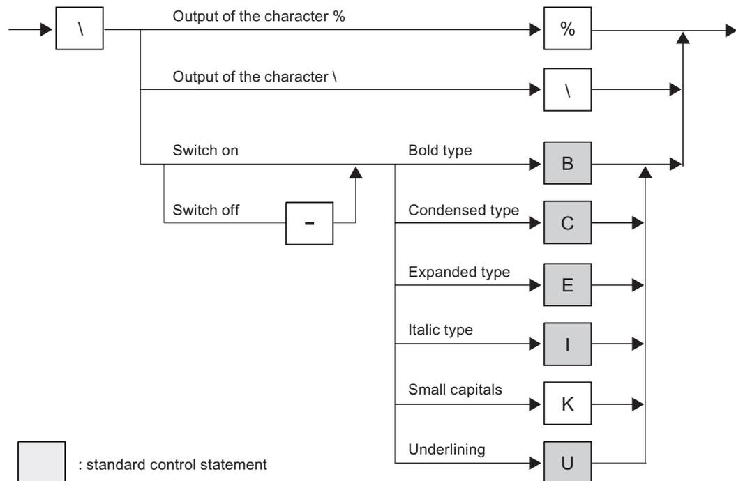
Figure 2-30 Schematic structure of control statements
