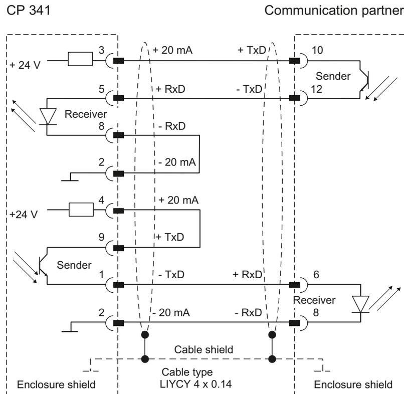
Figure B-10 20mA-TTY connecting cable CP 341 - CP 523
