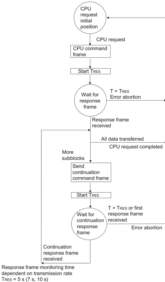
Figure 2-18 Flow diagram of data transmission with the RK 512 when CPU requests are made
