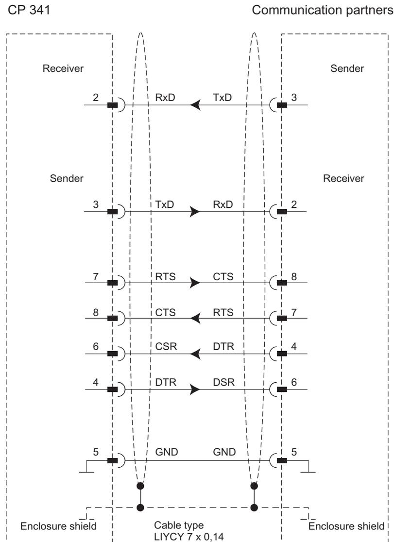
Figure B-1 RS 232C connecting cable CP 341 - CP 340/CP 341/CP 441
