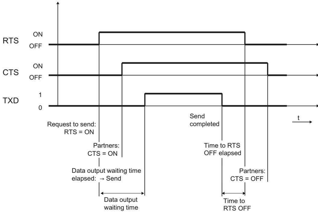
Figure 2-24 Timing diagram of automatic control of the RS 232C accompanying signals
