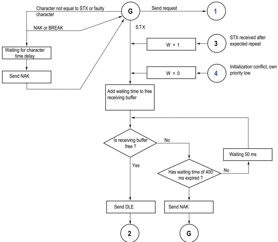
Figure 2-8 Flow Diagram for Receiving with the 3964(R) Procedure (Part 1)
