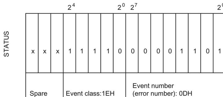
Figure 8-2 Example: Structure of the STATUS parameter for the the "Request canceled due to complete restart, restart or reset" event
