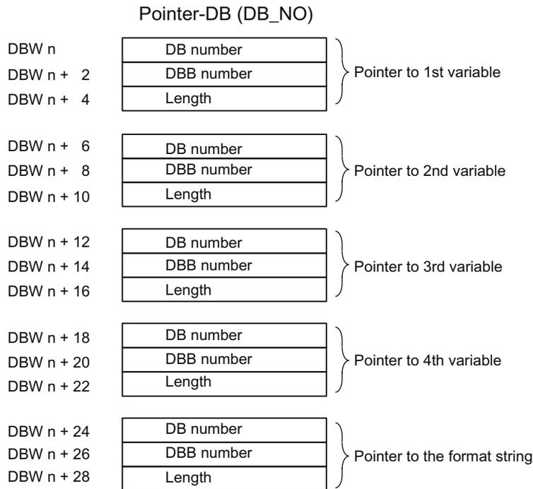
Figure 6-7 Structure of the POINTER DB for the FB P\_PRINT\_RK function block
