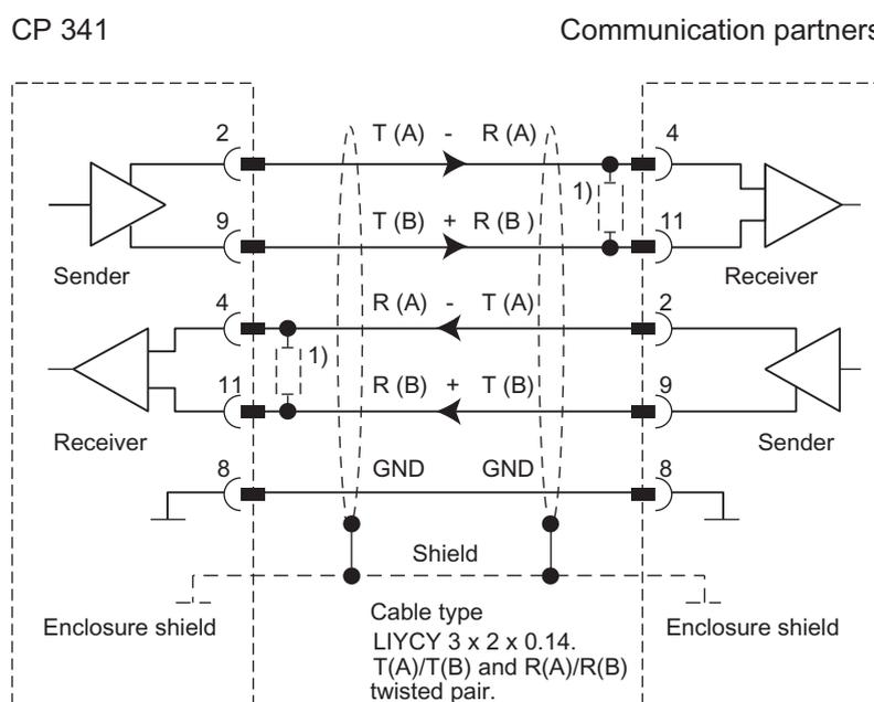
1) For line lengths of more than 50 m, you will have to weld in a terminating resistor of approximately  $330 \Omega$  on the receiver end for trouble-free data traffic.
