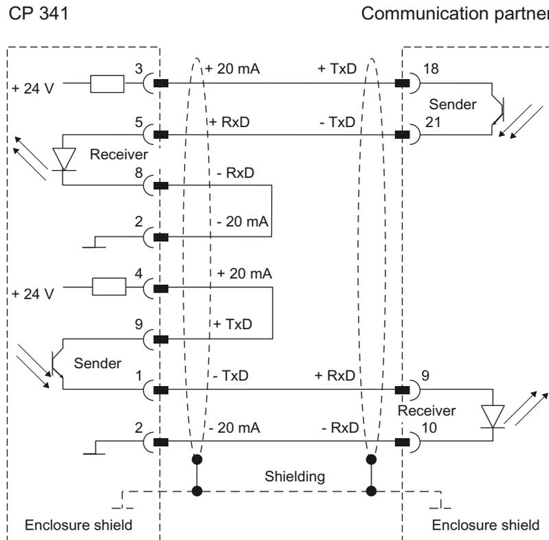
Figure B-11 20mA-TTY connecting cable CP 341 - CP 521 SI/CP 521 BASIC
