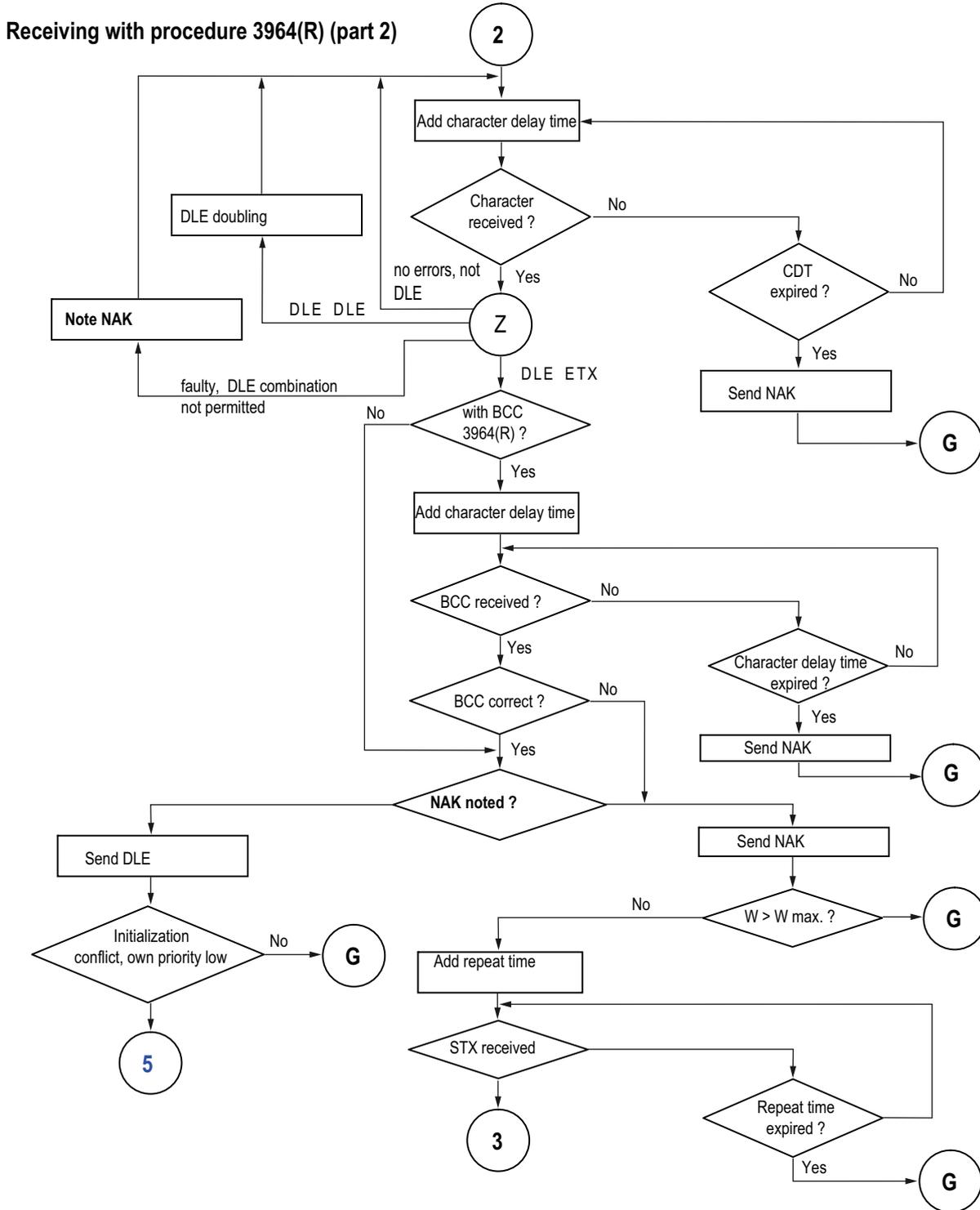
Figure 2-9 Flow diagram for receiving with the 3964(R) procedure (Part 2)
