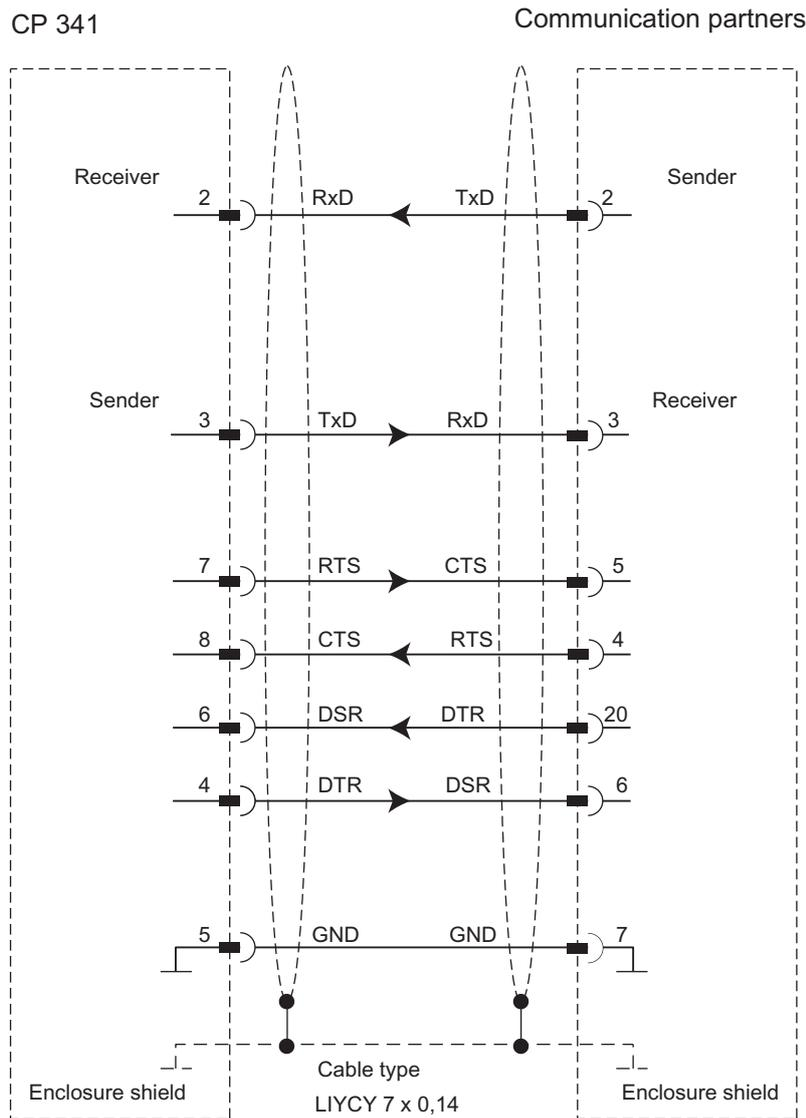
Figure B-2 RS 232C connecting cable (CP 341 - CP 544, CP 524, CPU 928B, CPU 945, CPU 948)
