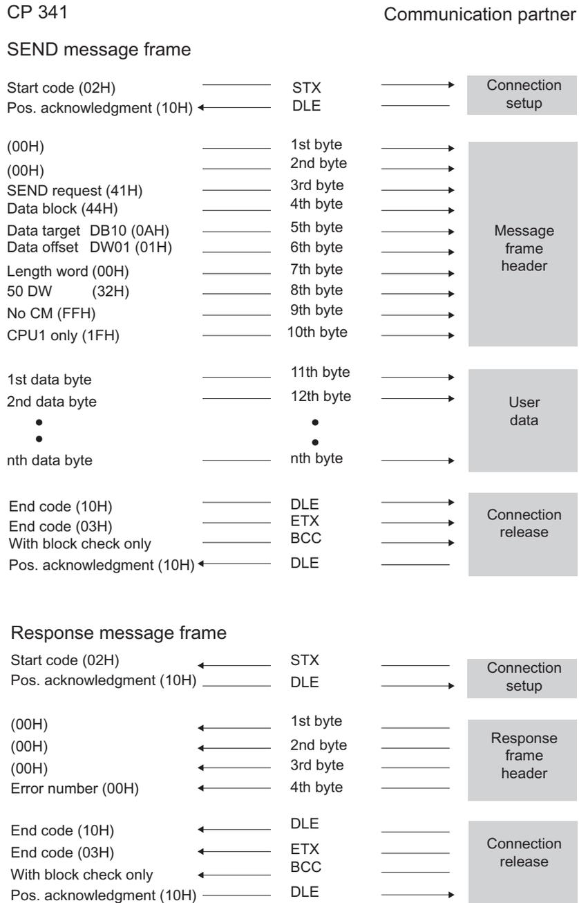
Figure 2-13 Data traffic when sending with a response message frame
