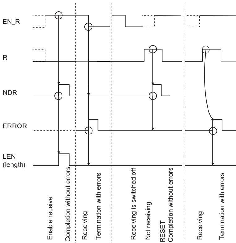
Figure 6-5 Time sequence chart of FB 7 P\_RCV\_RK for "Provide data" request
