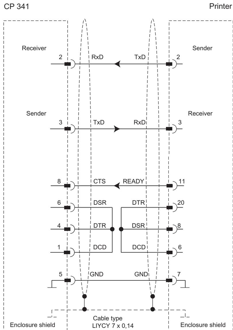
Figure B-5 RS 232C connecting cable CP 341 - IBM Proprinter
