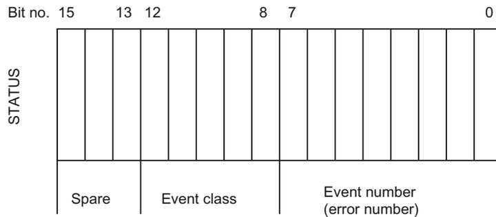
Figure 8-1 Structure of the STATUS parameter
