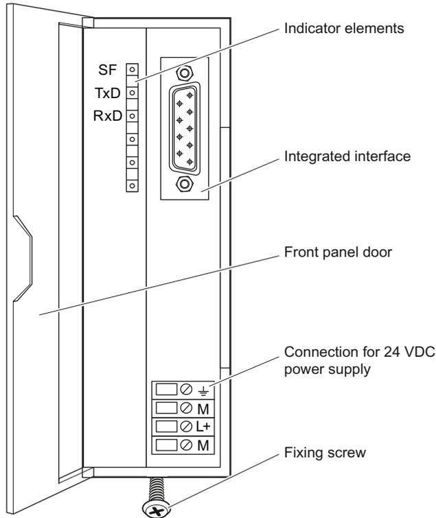
Figure 1-1 Positions of the module elements on the CP 341 communication processor
