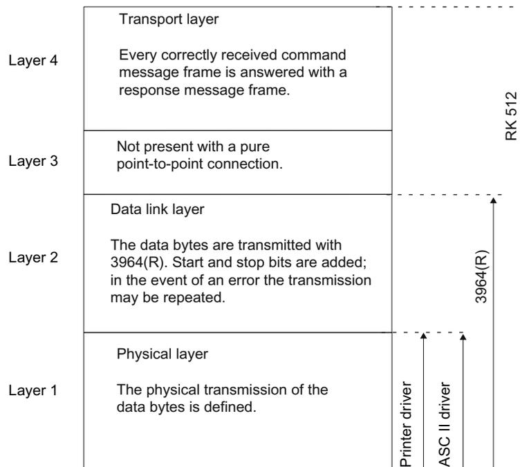
Figure 2-3 Position of the supplied protocols of the CP 341 in the reference model
