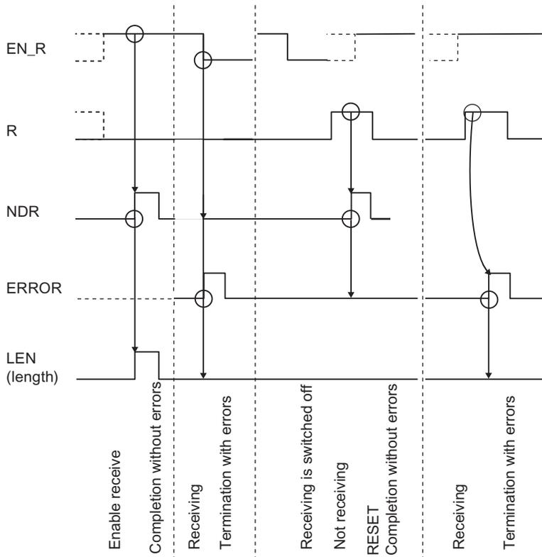
Figure 6-4 Time sequence chart of FB 7 P\_RCV\_RK for "Receive data" request
