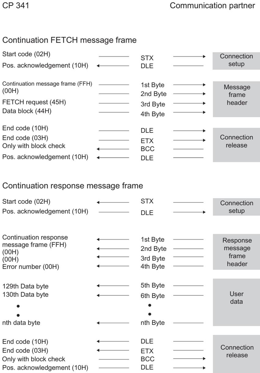
Figure 2-16 Sequence of a continuation FETCH message frame with a continuation response message frame
