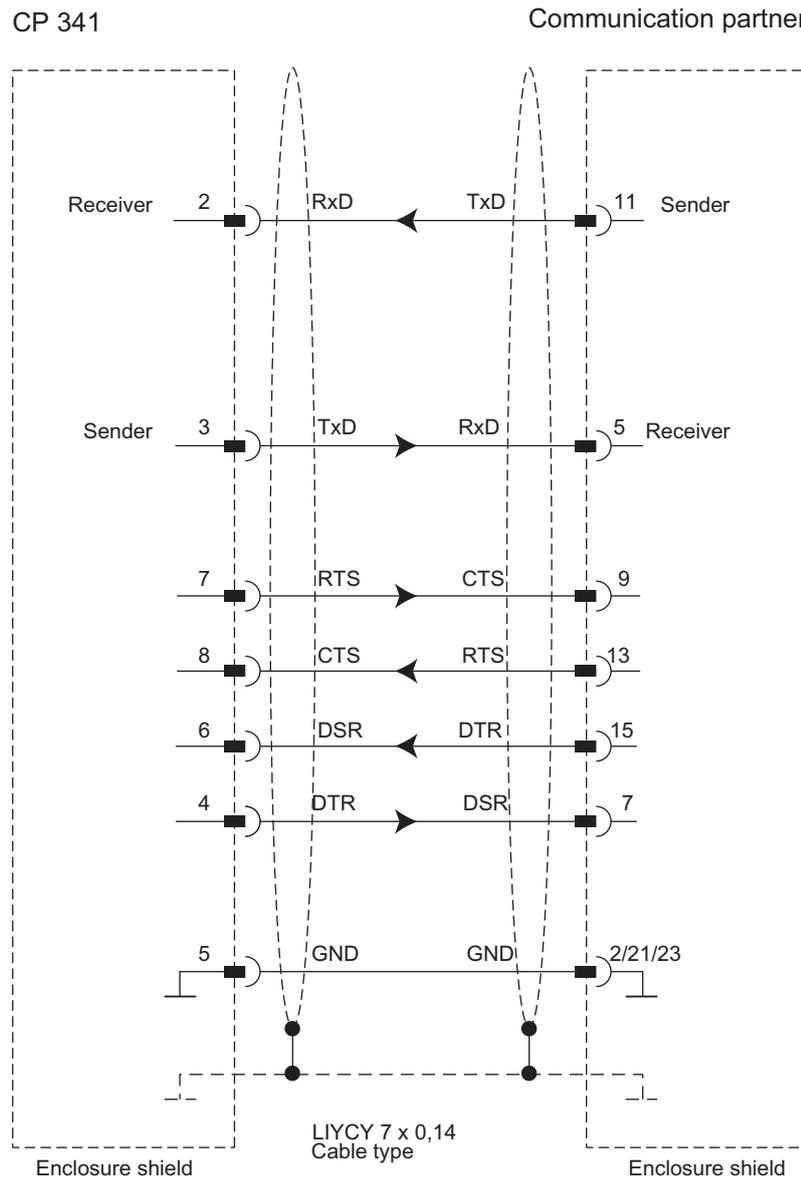
Figure B-4 RS 232C connecting cable CP 341 - CP 523
