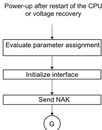
Figure 2-12 Flow diagram of the start-up of the 3964(R) Procedure
