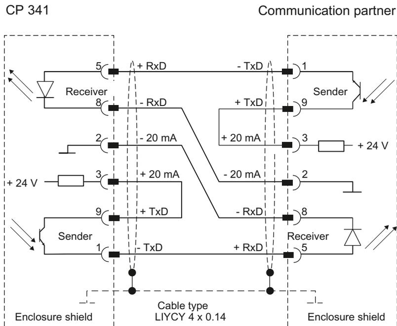
Figure B-8 20mA-TTY connecting cable CP 341 - CP 340/CP 341/CP 441
