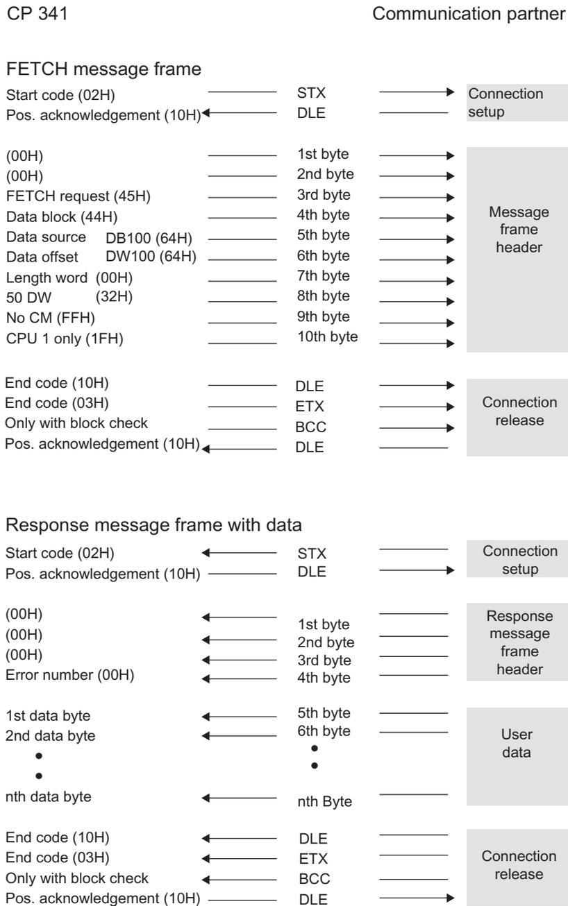
Figure 2-15 Data traffic when fetching with a response message frame
