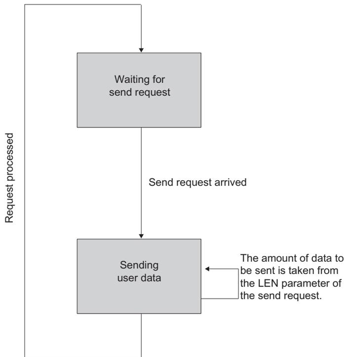
Figure 2-20 Flowchart of a send operation
