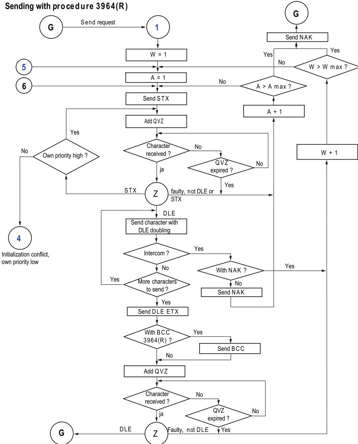
Figure 2-6 Flow diagram of sending with the 3964(R) procedure
