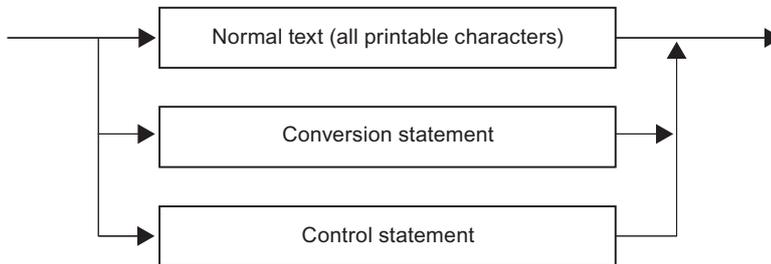
Figure 2-28 Schematic structure of the format string
