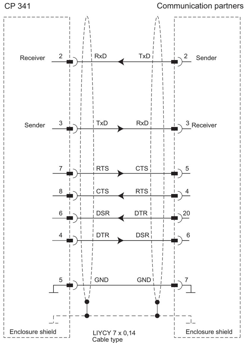
Figure B-3 RS 232C connecting cable CP 341 - CP 521 SI/CP 521 BASIC
