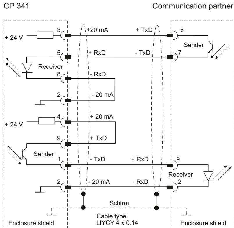
Figure B-12 20mA-TTY connecting cable CP 341 - CPU 944/AG 95
