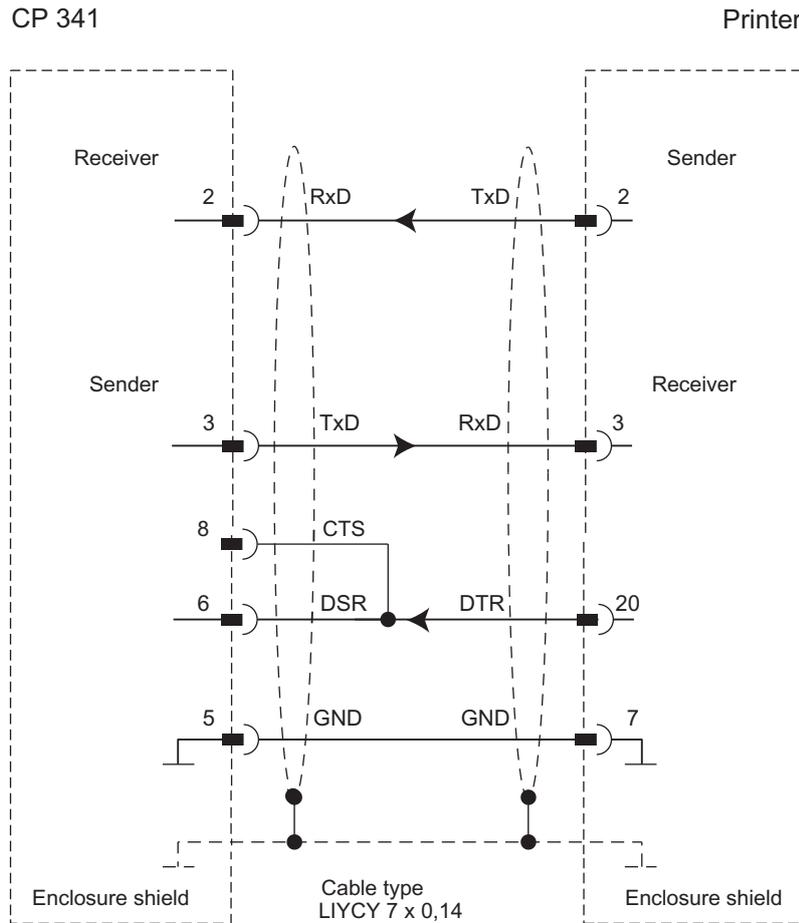
Figure B-6 RS 232C connecting cable CP 341 - laser printer
