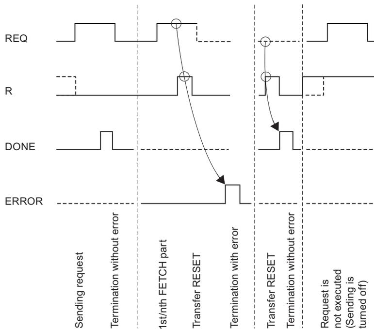
Figure 6-6 Time sequence chart of FB 8 P\_SND\_RK for "Fetch data" request
