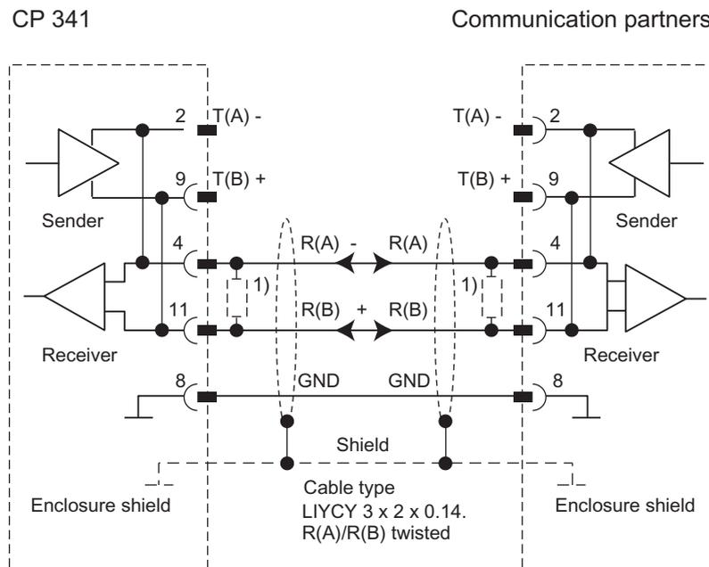
1) For line lengths of more than 50 m, you will have to weld in a terminating resistor of approximately 330 Ω on the receiver end for trouble-free data traffic.
