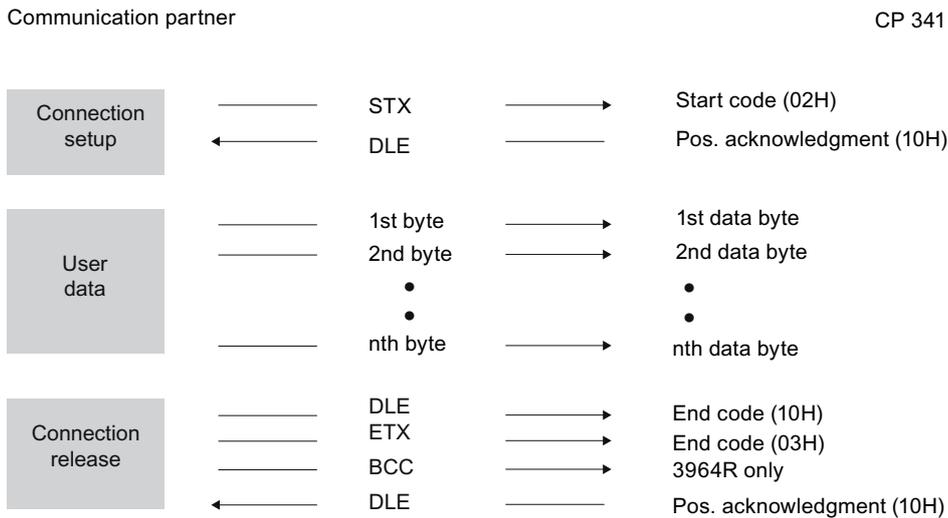
Figure 2-7 Data traffic when receiving with the 3964(R) procedure
