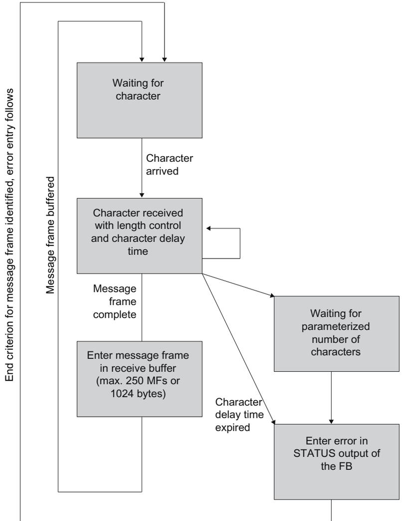
Figure 2-23 Flow diagram for receiving with end criterion "Fixed message frame length"
