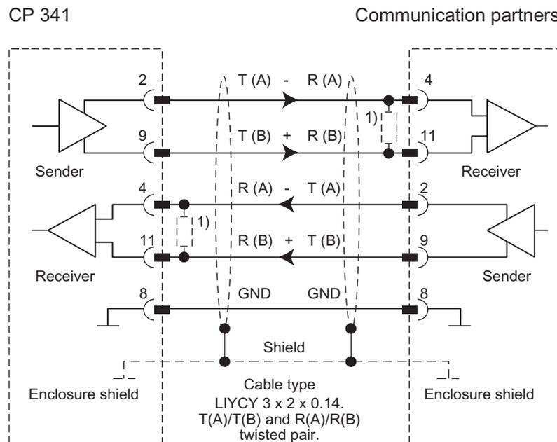
1) For line lengths of more than 50 m, you will have to weld in a terminating resistor of approximately  $330 \Omega$  on the receiver end for trouble-free data traffic.
