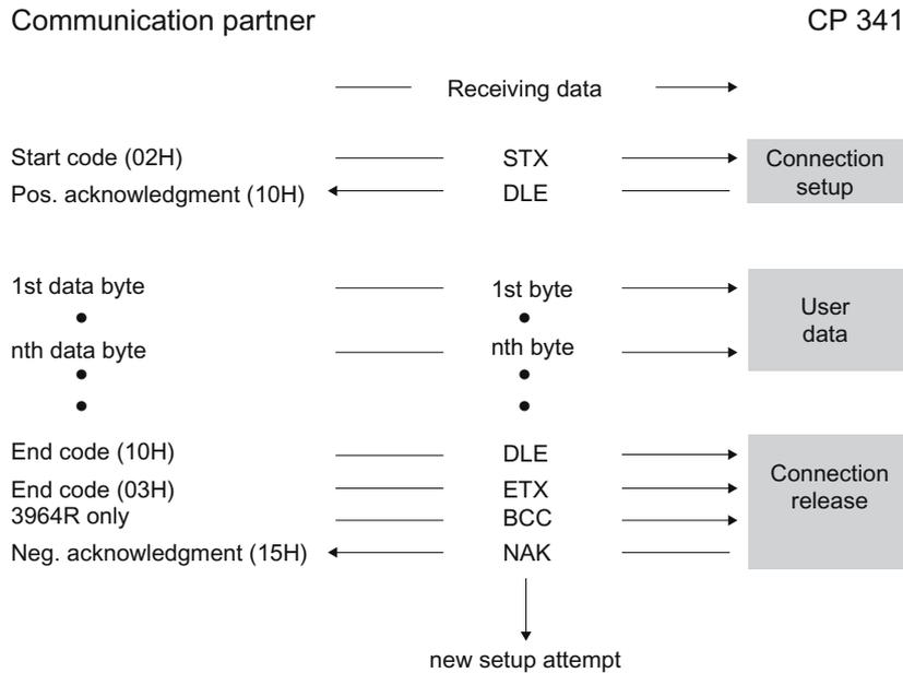
Figure 2-10 Data traffic when erroneous data is received
