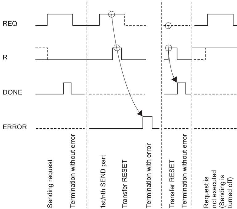
Figure 6-3 FB 8 P\_SND\_RK time sequence chart for "Send data" request
