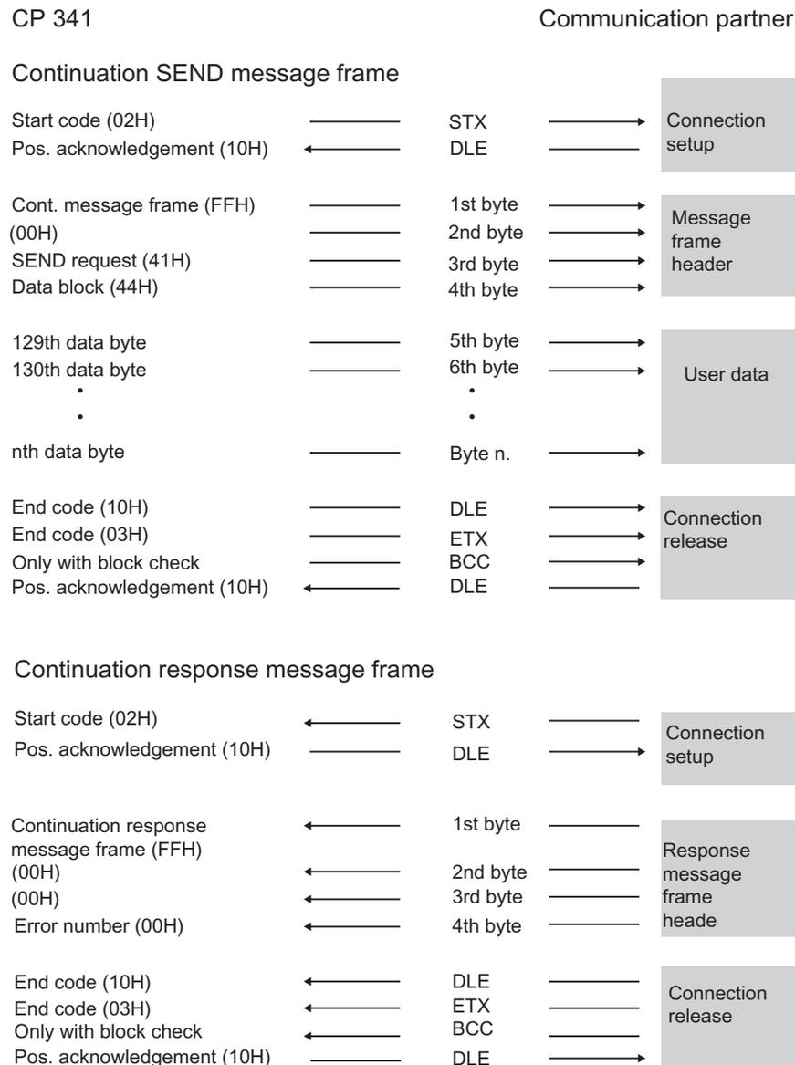
Figure 2-14 Sequence of a continuation SEND message frame with a continuation response message frame
