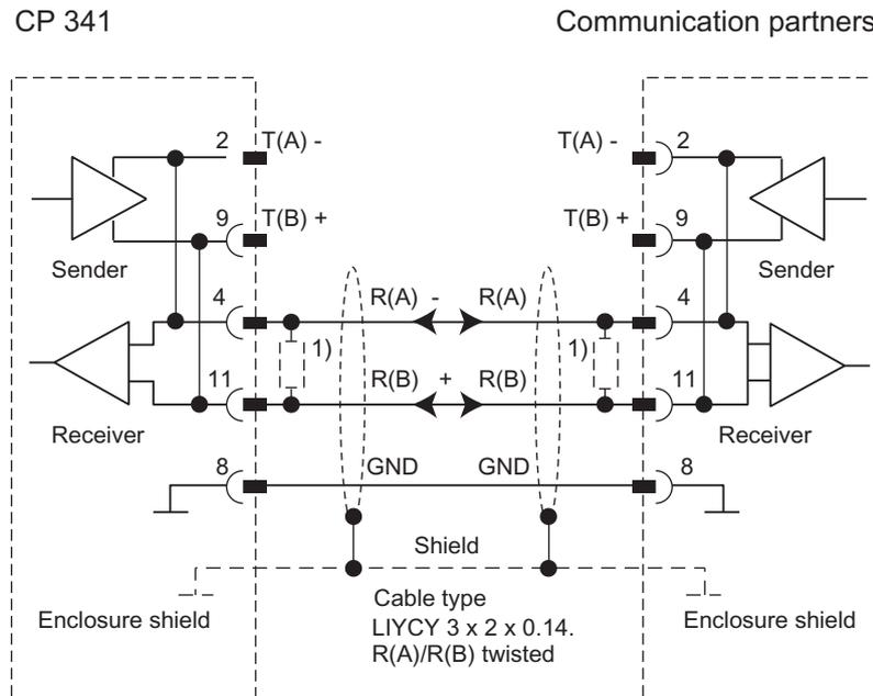
1) For line lengths of more than 50 m, you will have to weld in a terminating resistor of approximately 330 Ω on the receiver end for trouble-free data traffic.
