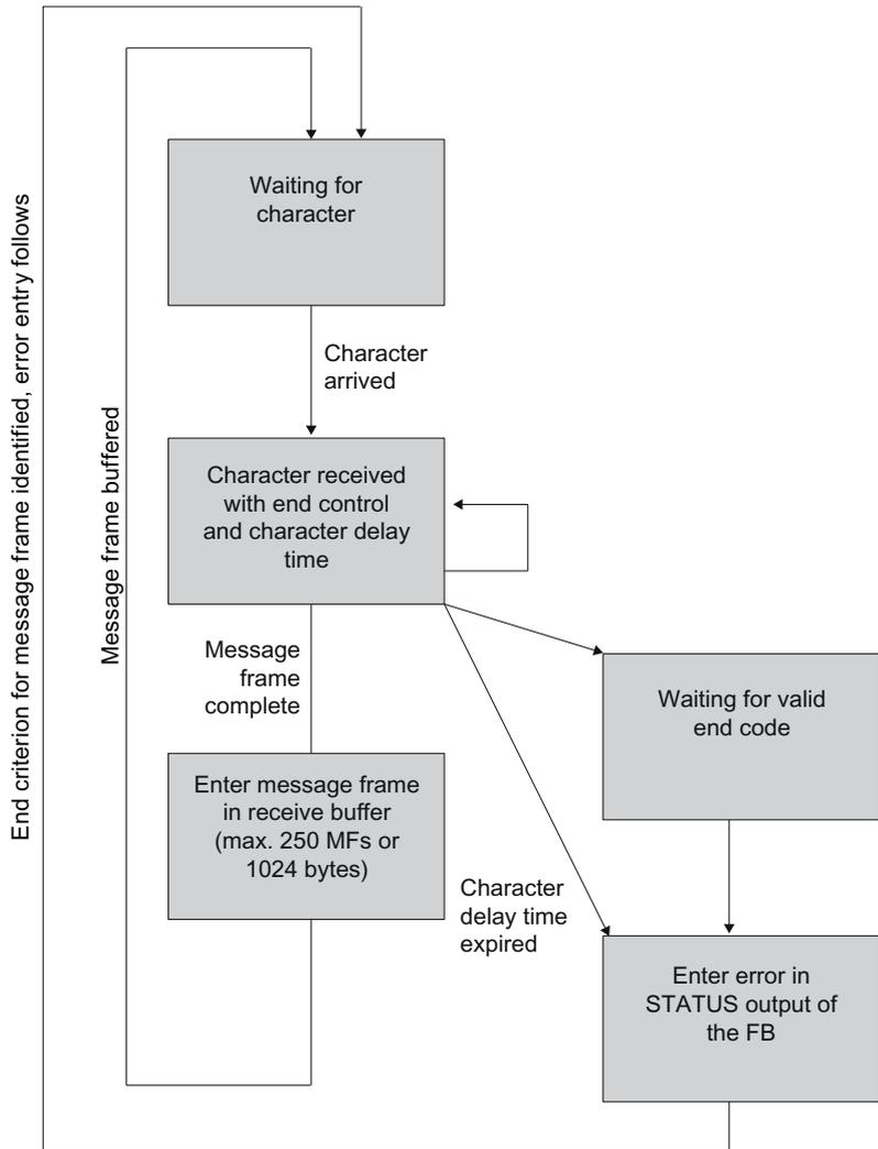
Figure 2-22 Flow diagram for receiving with end criterion "End-of-text character"
