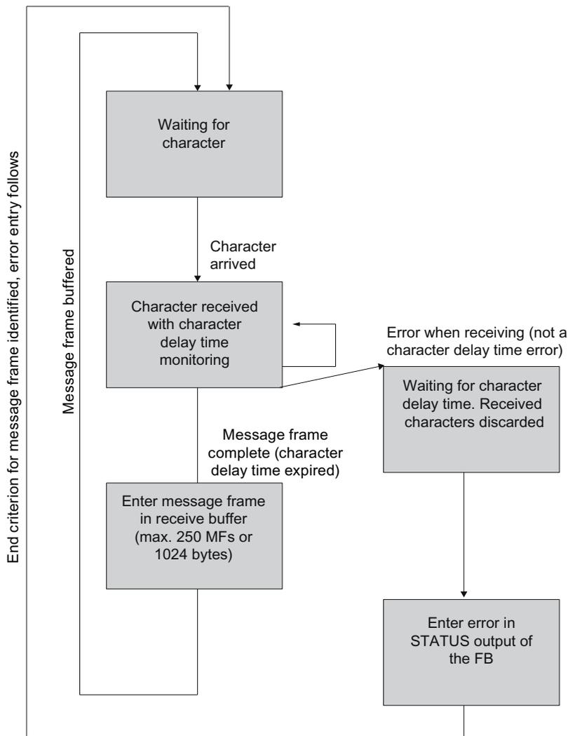
Figure 2-21 Flow diagram for receiving with end criterion "Expiration of character delay time"
