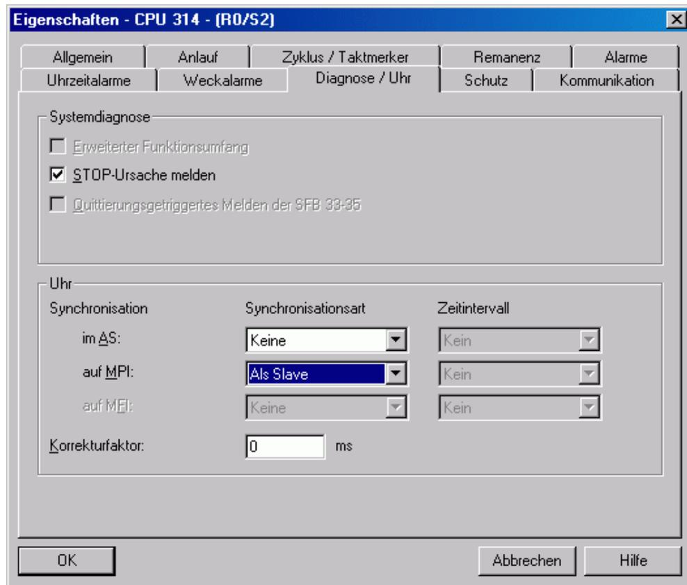
Further information about SIMATIC time synchronization can be found in the FAQ "How is the SIMATIC S7-300 configured as time master or time slave for time synchronization via Industrial Ethernet with the SIMATIC procedure?":
