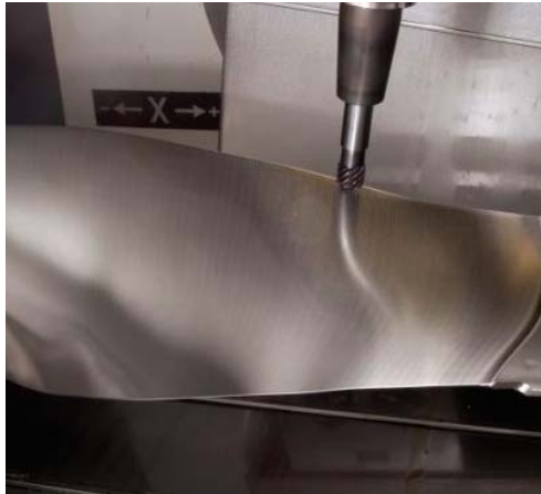
Turbine blade during machining. Face milling on the other side with rotation about the X axis.
