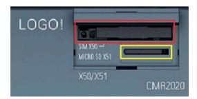
Figure 3-2 Compartment for the SIM card (red rectangle)
