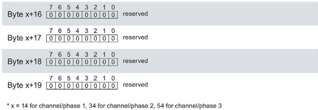
Figure A-4 Channel parameter block
