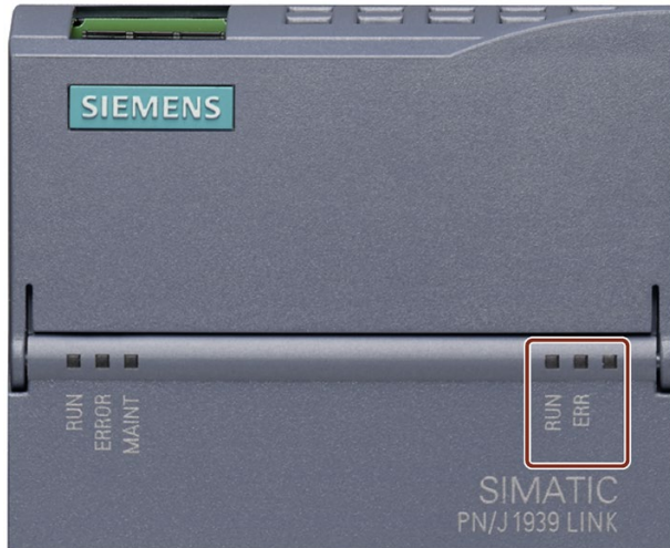
Figure 10-3 Status LEDs PN/J1939 LINK
