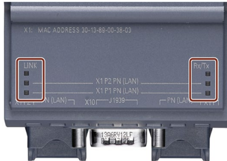
Figure 10-2 Status LEDs, Ethernet interfaces
