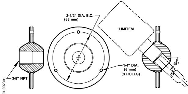
**Figure 2. Swivel Flange Mounting Kit
