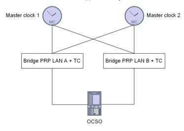
Figure 10-9 IEEE 1588 Time Synchronization via a PRP Network, Using External Master Clocks
