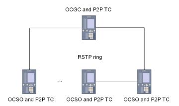
Figure 10-16 IEEE 1588 Time Synchronization via an RSTP Ring, Using SIPROTEC 5 as the Grandmaster-Capable Clock
