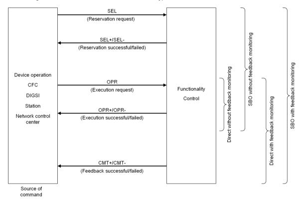
Figure 2-32 Command Sources, Command Types and Control Models
