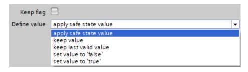
Figure 11-26 Value Definition of a Data Object of the SPS Type
