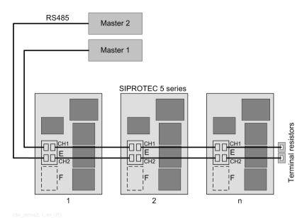
Figure 1-20 Redundant Communication with 2 Masters Using RS485 Bus (for Example, Redundant IEC 60870-5-103 Protocol)
