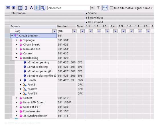
Figure 2-16 GOOSE Indication in the Logical Node
