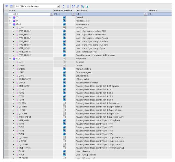
Figure 2-19 IEC 61850 Structure of a SIPROTEC 5 Device (SIPROTEC 4 Similar View)
