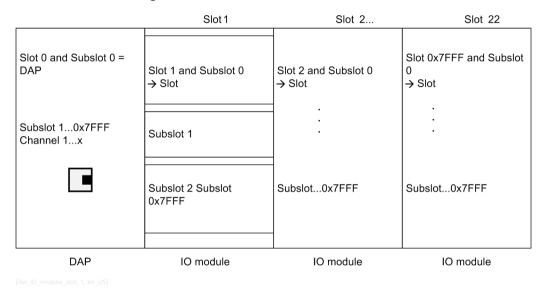
Figure 7-2 Addressing of IO Data in PROFINET Based on Slots and Subslots
