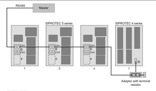
Figure 1-19 Communication with a Single Master Using an RS485 Bus
