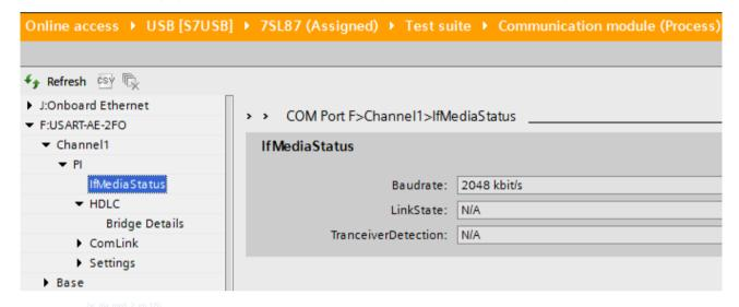
Figure 11-18 Diagnostic Data of the Protection-Interface Log - Media Status
