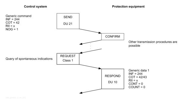
Figure 6-6 Reading an Individual Parameter
