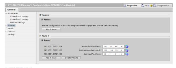
Figure 1-34 Static IP Route Settings
