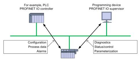
Field devices PROFINET IO device
