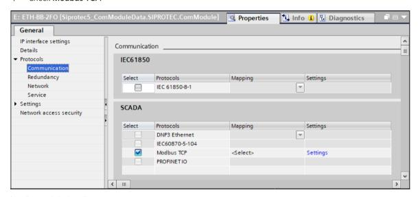
Figure 5-1 Modbus-TCP Activation
