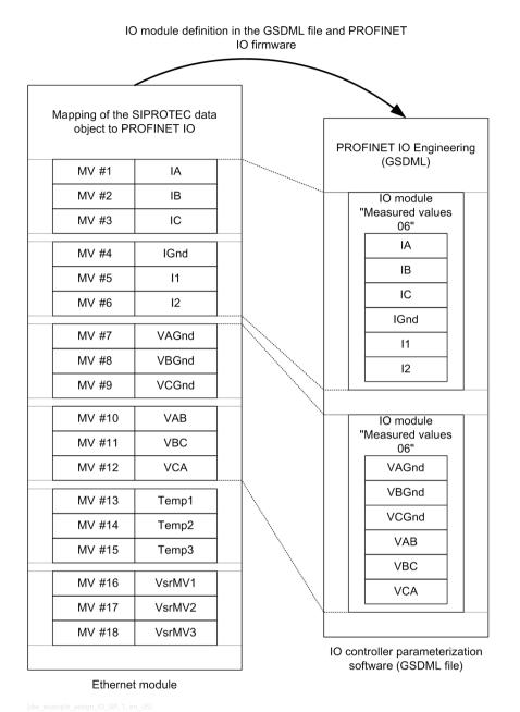
Figure 7-15 Example of Assigning the IO Modules to SIPROTEC 5 Data Objects (Measured Values)
