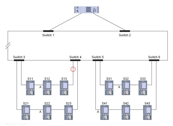
Figure 1-15 Broken Connection with Shifting of the Alternate Ports
