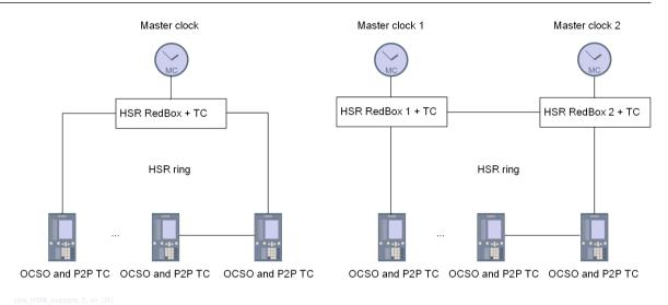
Figure 10-12 IEEE 1588 Time Synchronization via an HSR Ring, Using External Master Clocks
