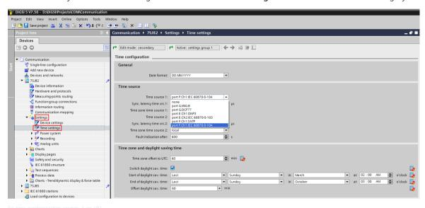
Figure 1-46 Setting Possibilities for the Time Sources
