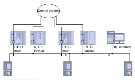
Figure 4-4 Master Redundancy
