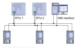
Figure 4-3 Media Redundancy
