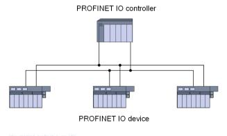
Figure 7-20 Media Redundancy
