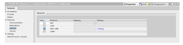
Figure 10-5 IEEE 1588 Activation for the Module ETH-BD-2FO
