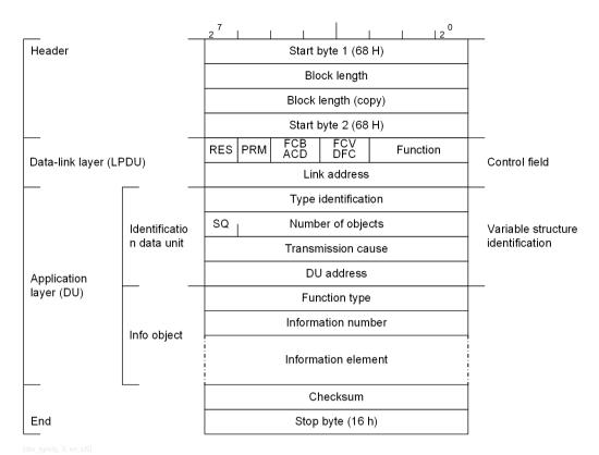
Figure 6-1 Telegram with Variable Length
