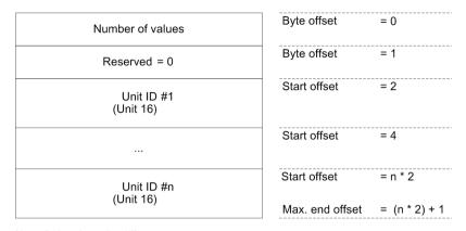
Figure 7-19 Acyclic Data Telegram and Reading Unit IDs
