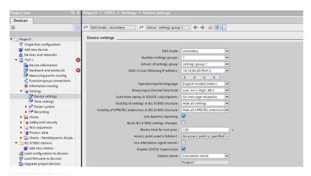
Figure 11-28 Device Settings for IEC 61850 – Enable GOOSE Supervision
