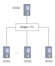
Figure 10-8 IEEE 1588 Time Synchronization via Line Mode, Using SIPROTEC 5 as the Grandmaster-Capable Clock
