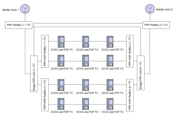
Figure 10-17 IEEE 1588 Time Synchronization via a PRP-HSR Network
