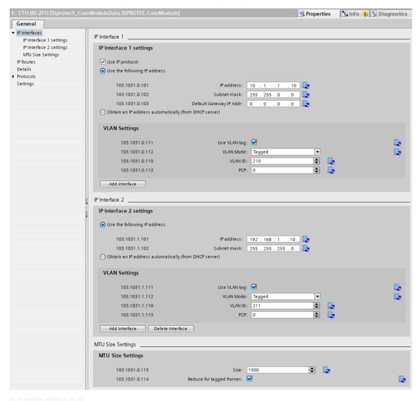
Figure 1-32 Multiple IP-Interfaces Settings
