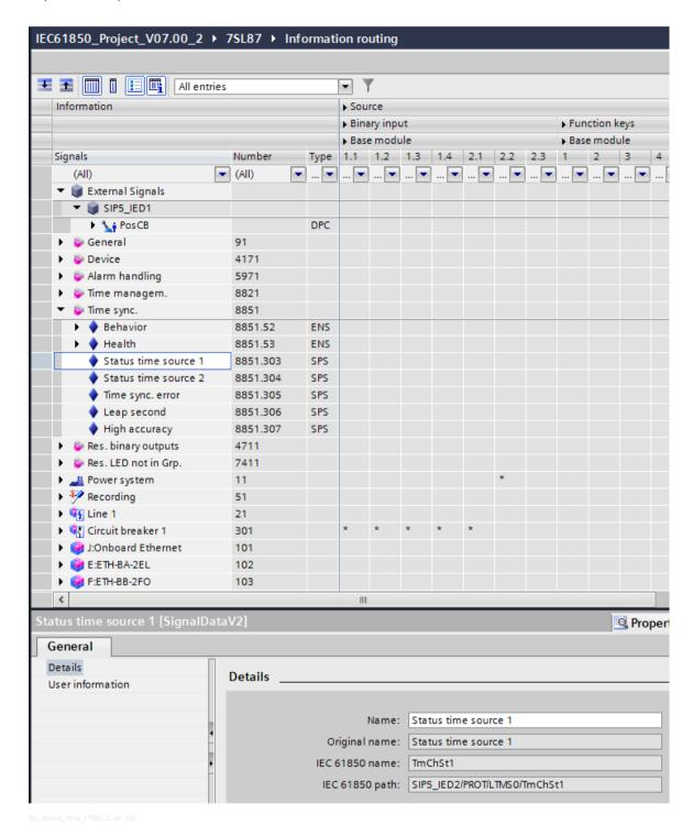
Figure 2-39 Device-Time Messages – Example LN/LTMS
