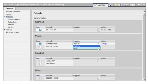
Figure 1-37 Selecting Mapping – Example for DNP3
