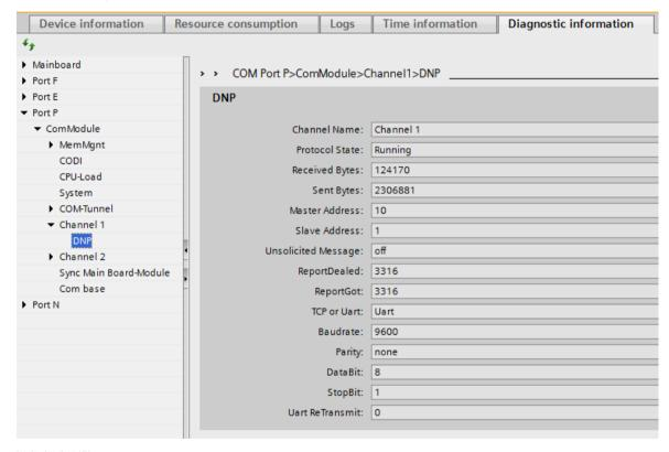
Figure 11-8 DNP3 Serial Diagnostic Data in DIGSI
