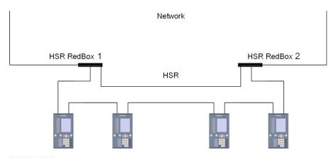
Figure 1-13 SIPROTEC Devices Arranged in Rings
