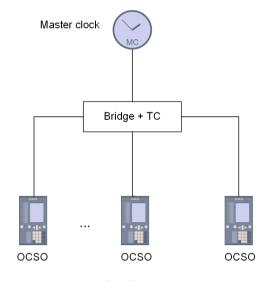
Figure 10-7 IEEE 1588 Time Synchronization via Line Mode, Using an External Master Clock
