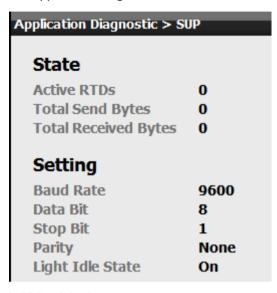
Figure 10-59 Application Diagnostic – SUP Serial
