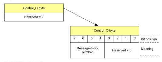
Figure 7-18 Structure of the Event List Data, Output Direction (ACK)
