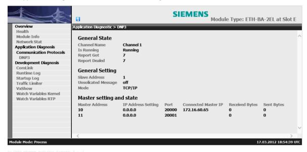
Figure 10-54 Application Diagnostic – DNP3 Ethernet
