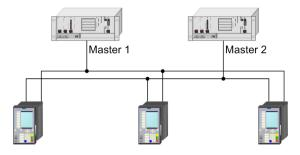
Figure 6-4 Master Redundancy
