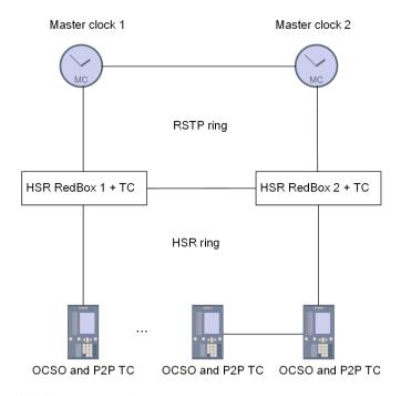
Figure 10-18 IEEE 1588 Time Synchronization via an RSTP-HSR Network
