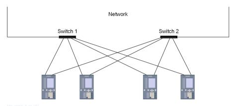
Figure 1-12 SIPROTEC Devices Connected via 2 Independent Networks (LAN A and LAN B)
