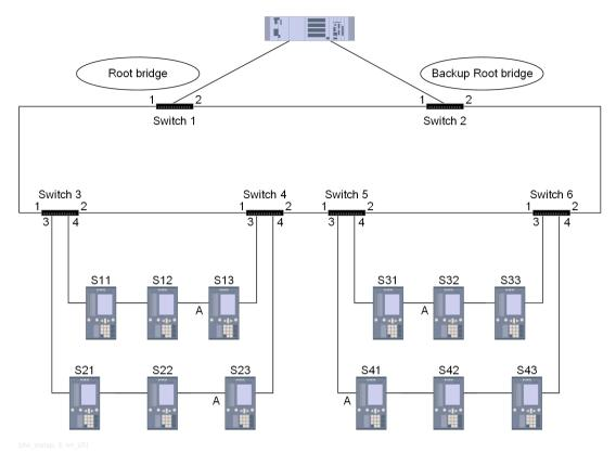
Figure 1-14 Structure with Alternate Ports
