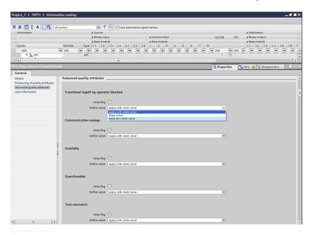
Figure 11-25 Advanced Quality Attributes for GOOSE Later Binding
