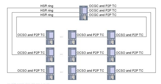
Figure 10-14 IEEE 1588 Time Synchronization via HSR Rings, Using SIPROTEC 5 as the Grandmaster-Capable Clock
