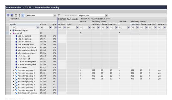
Figure 6-10 Mapping Commands for Settings Group Switching
