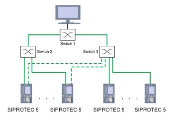
Figure 1-6 Dual Homing with 2 Switches
