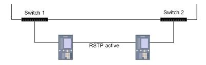
Figure 1-7 Redundant Connection with Different Network Switches
