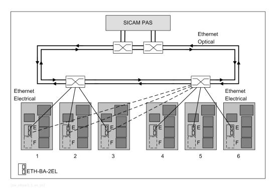
Figure 1-17 Operation of Ethernet Modules Without Integrated Switch Function with Single or Redundant Connection to the Switch
