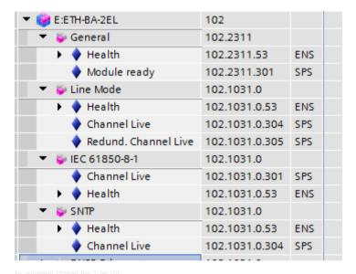
Figure 11-39 Signal Redund. Channel Live in the Information Routing
