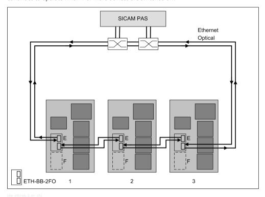
Figure 1-16 Operation of Ethernet Modules with an Integrated Switch Function
