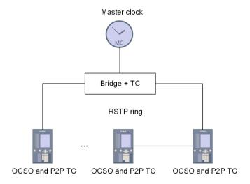
Figure 10-15 IEEE 1588 Time Synchronization via an RSTP Ring, Using an External Master Clock
