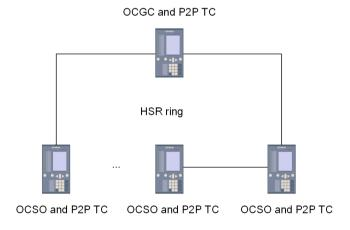
Figure 10-13 IEEE 1588 Time Synchronization via an HSR Ring, Using SIPROTEC 5 as the Grandmaster-Capable Clock
