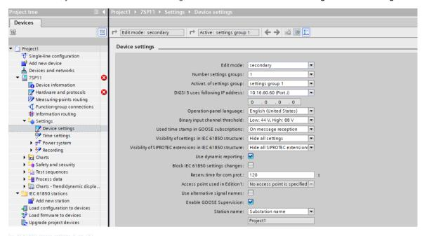
Figure 2-1 Device Settings for IEC 61850
