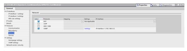
Figure 10-20 Selecting SNMP as the Network Protocol
