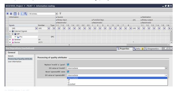
Figure 11-27 Influence Option When Linking a DPC Type Data Object
