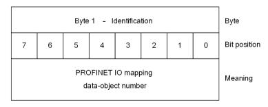
Figure 7-12 Byte 1: Identification in the Data Type Message Block
