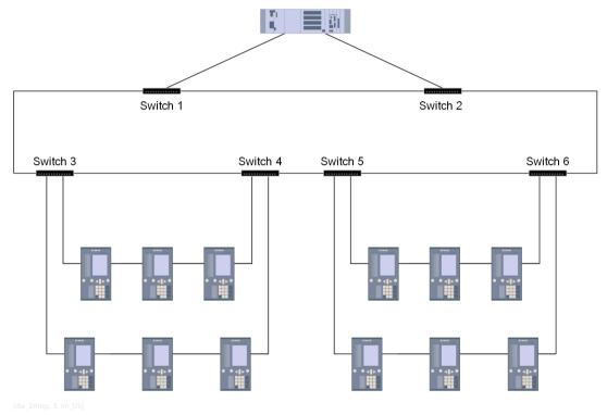
Figure 1-11 Dual-Ring Structure
